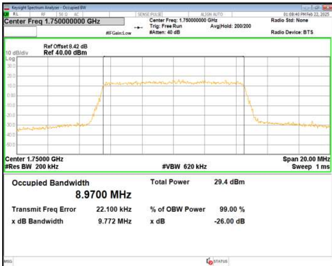
Band4 QPSK BW=15MHz Channel=20025 RB Size=75 Position=#0
