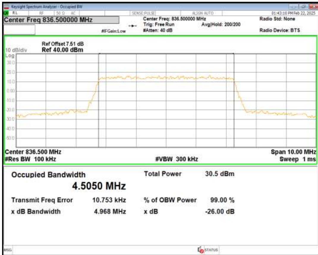
Band5 16QAM BW=5MHz Channel=20525 RB Size=25 Position=#0
