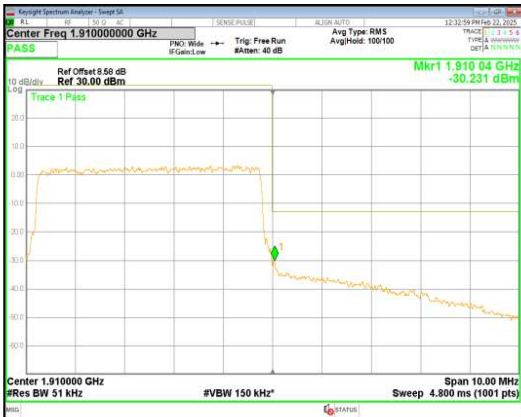
Band2 QPSK BW=10MHz Channel=18650 RB Size=50 Position=#0
