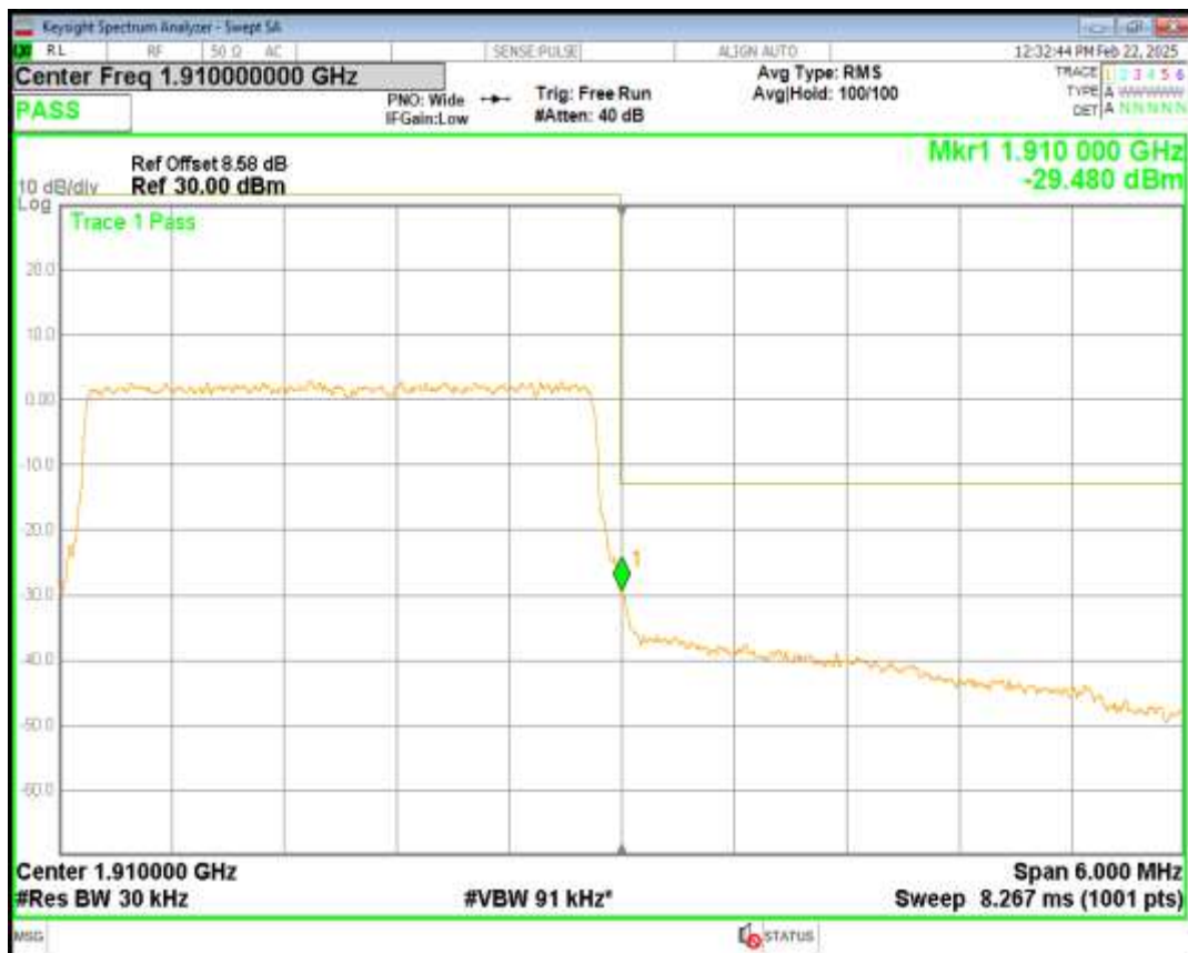
Band2 QPSK BW=5MHz Channel=18625 RB Size=25 Position=#0
