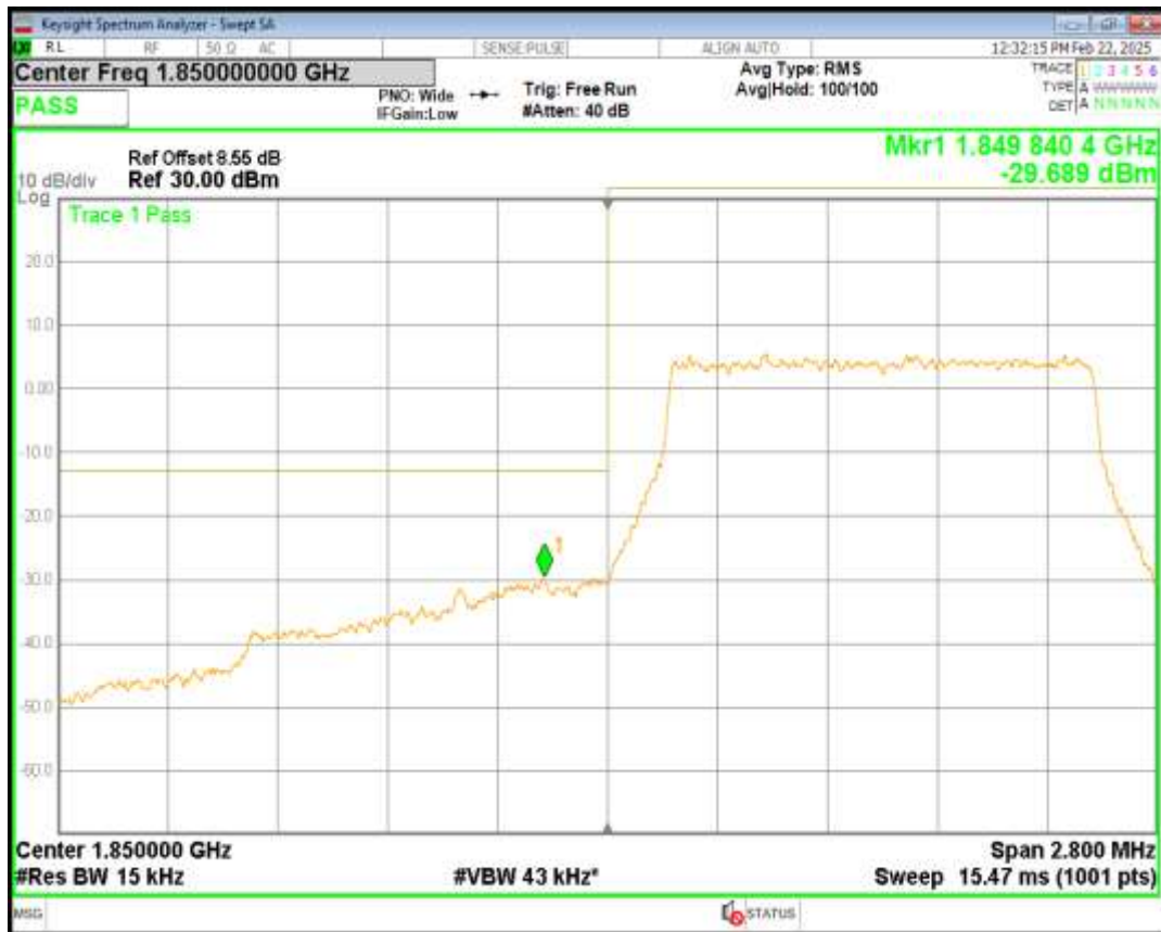
Band2 16QAM BW=1.4MHz Channel=18607 RB Size=6 Position=#0
