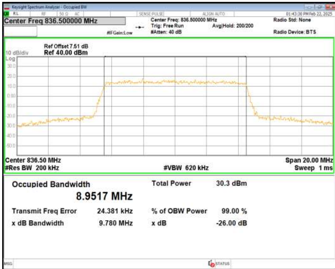
Band5 16QAM BW=10MHz Channel=20525 RB Size=50 Position=#0
