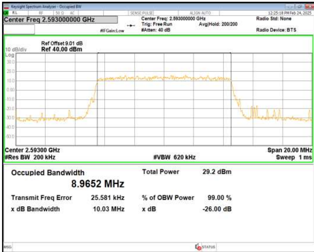
Band41 16QAM BW=10MHz Channel=40620 RB Size=50 Position=#0
