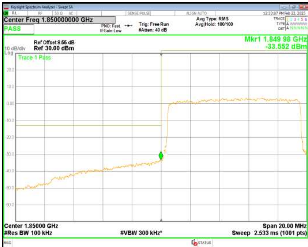
Band2 QPSK BW=10MHz Channel=19150 RB Size=50 Position=#0
