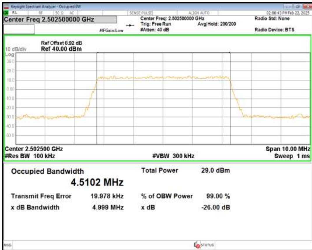
Band7 16QAM BW=5MHz Channel=20775 RB Size=25 Position=#0
