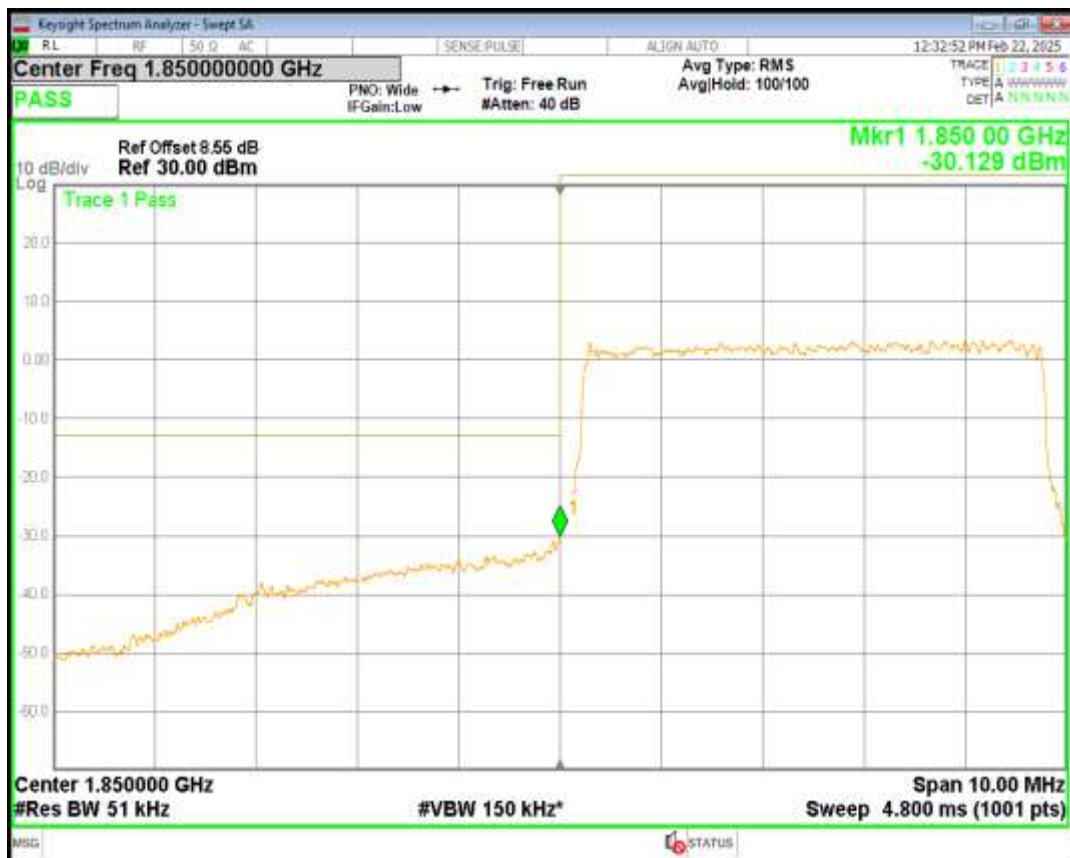
Band2 QPSK BW=5MHz Channel=19175 RB Size=25 Position=#0
