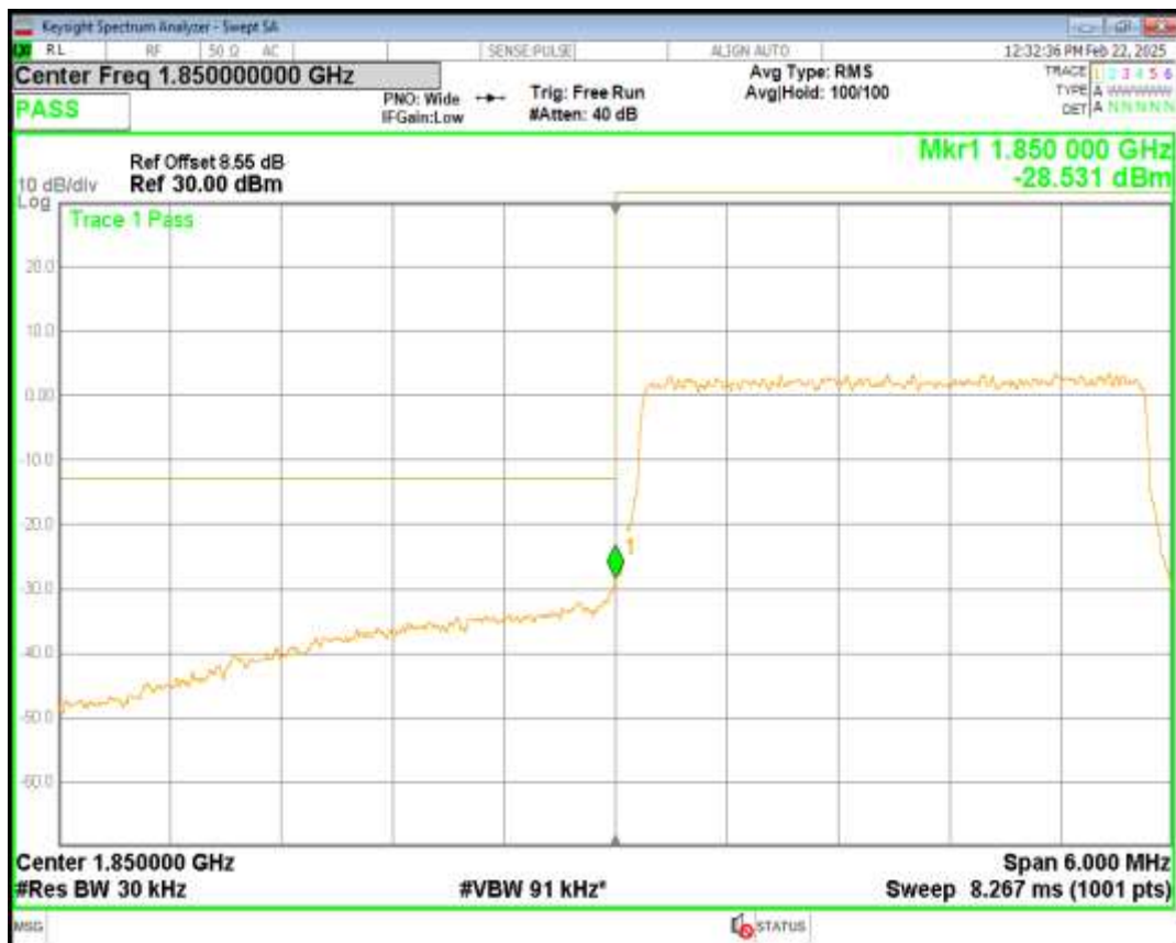
Band2 QPSK BW=3MHz Channel=19185 RB Size=15 Position=#0
