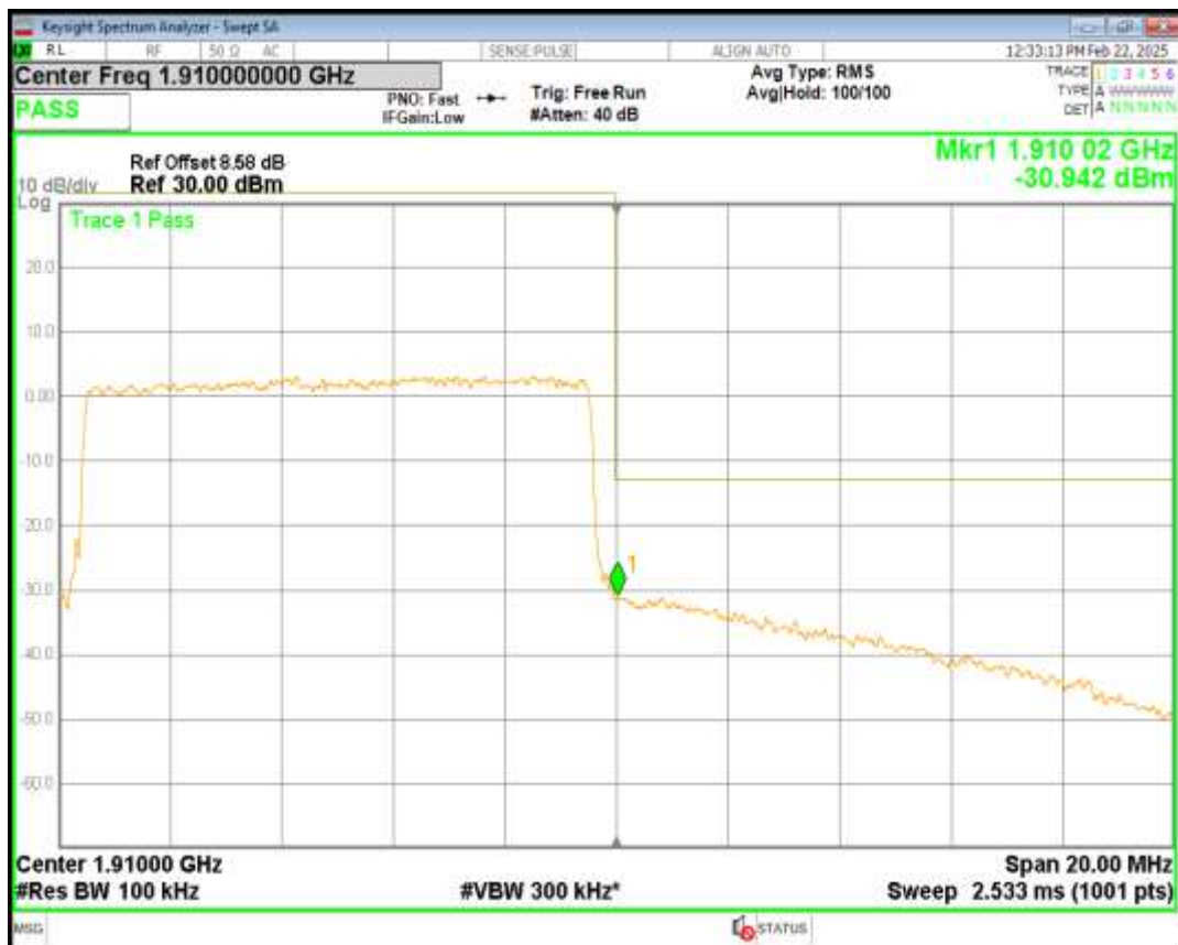
Band2 QPSK BW=15MHz Channel=18675 RB Size=75 Position=#0
