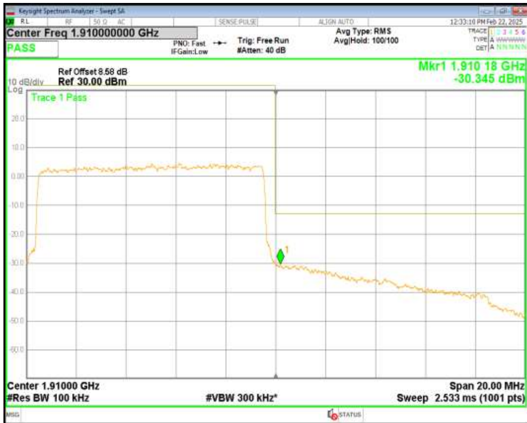
Band2 16QAM BW=10MHz Channel=19150 RB Size=50 Position=#0
