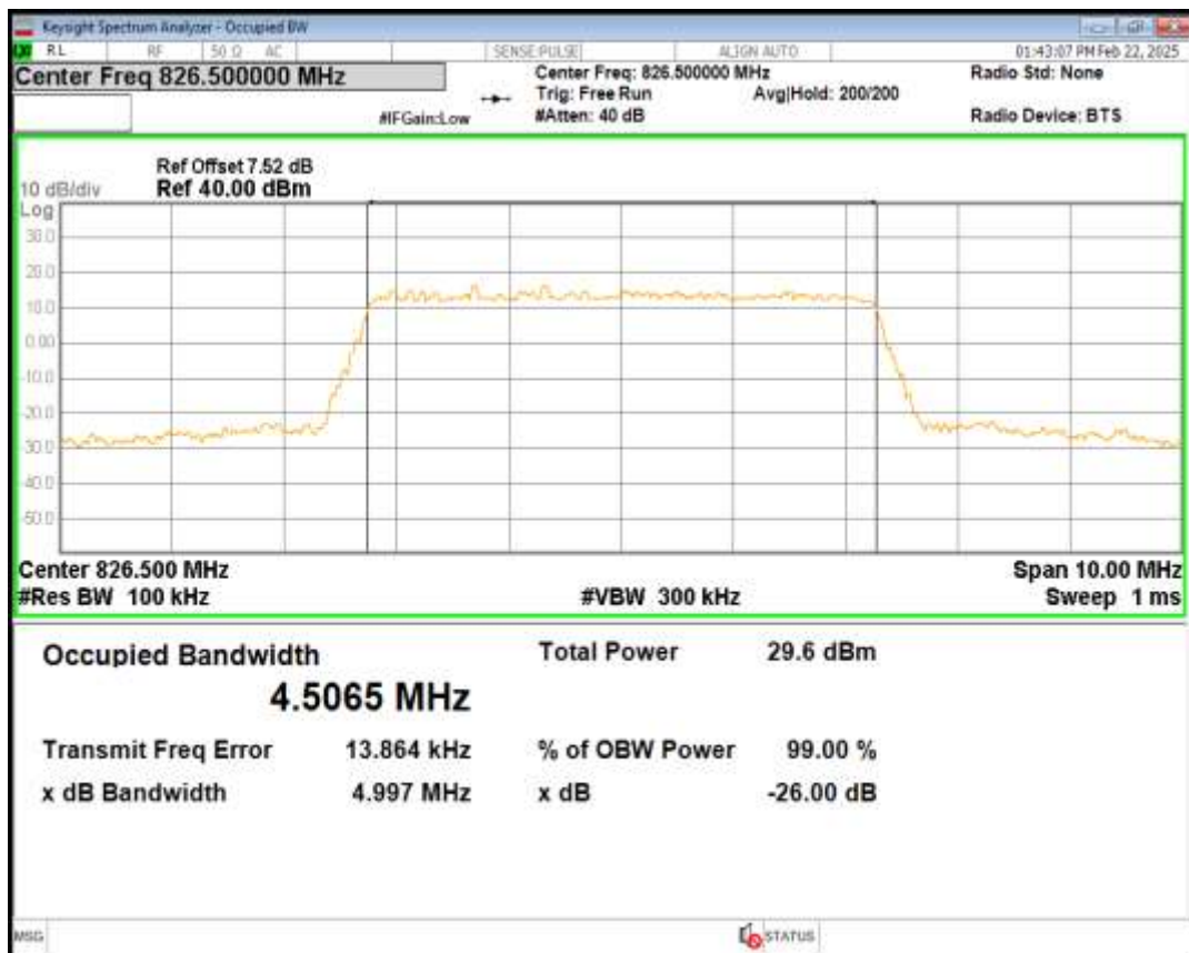
Band5 QPSK BW=5MHz Channel=20525 RB Size=25 Position=#0
