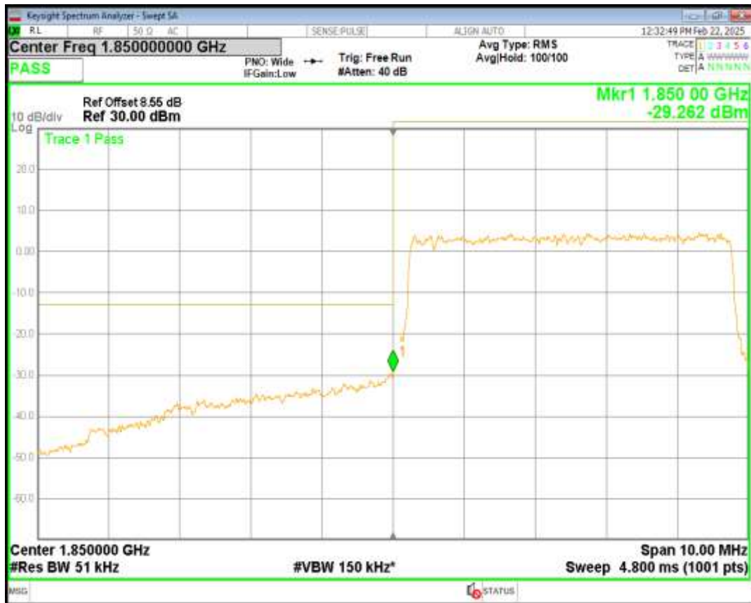
Band2 16QAM BW=5MHz Channel=18625 RB Size=25 Position=#0
