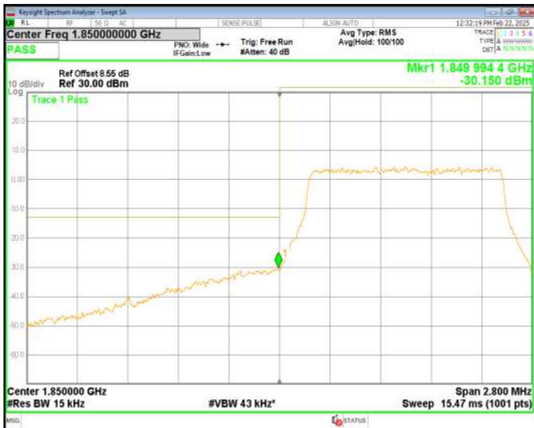
Band2 QPSK BW=1.4MHz Channel=19193 RB Size=6 Position=#0
