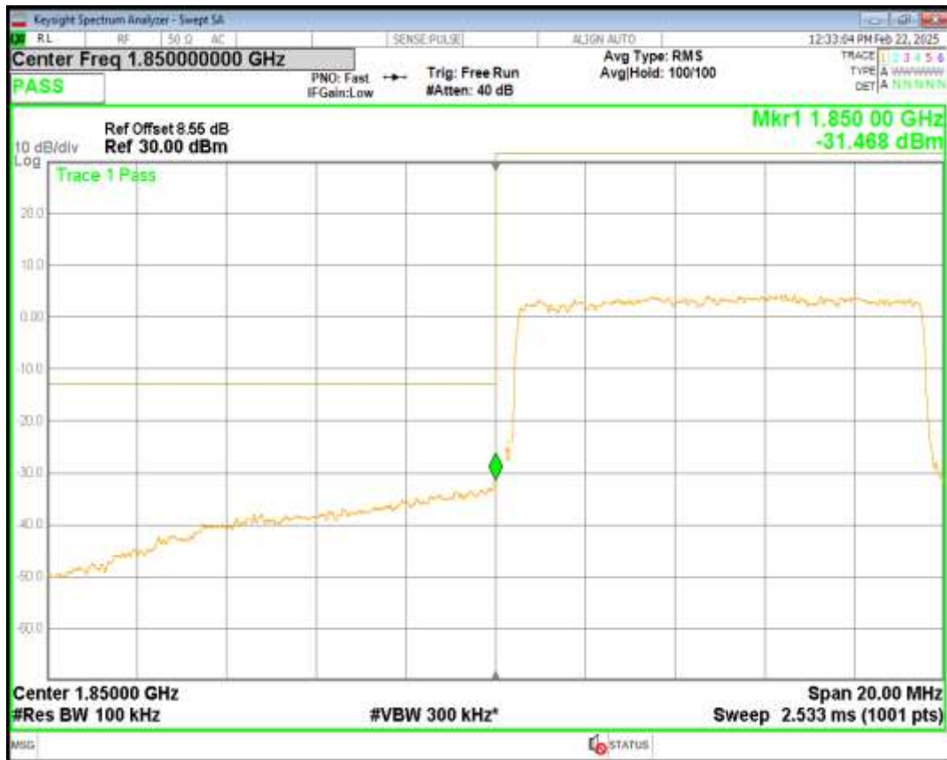
Band2 16QAM BW=10MHz Channel=18650 RB Size=50 Position=#0
