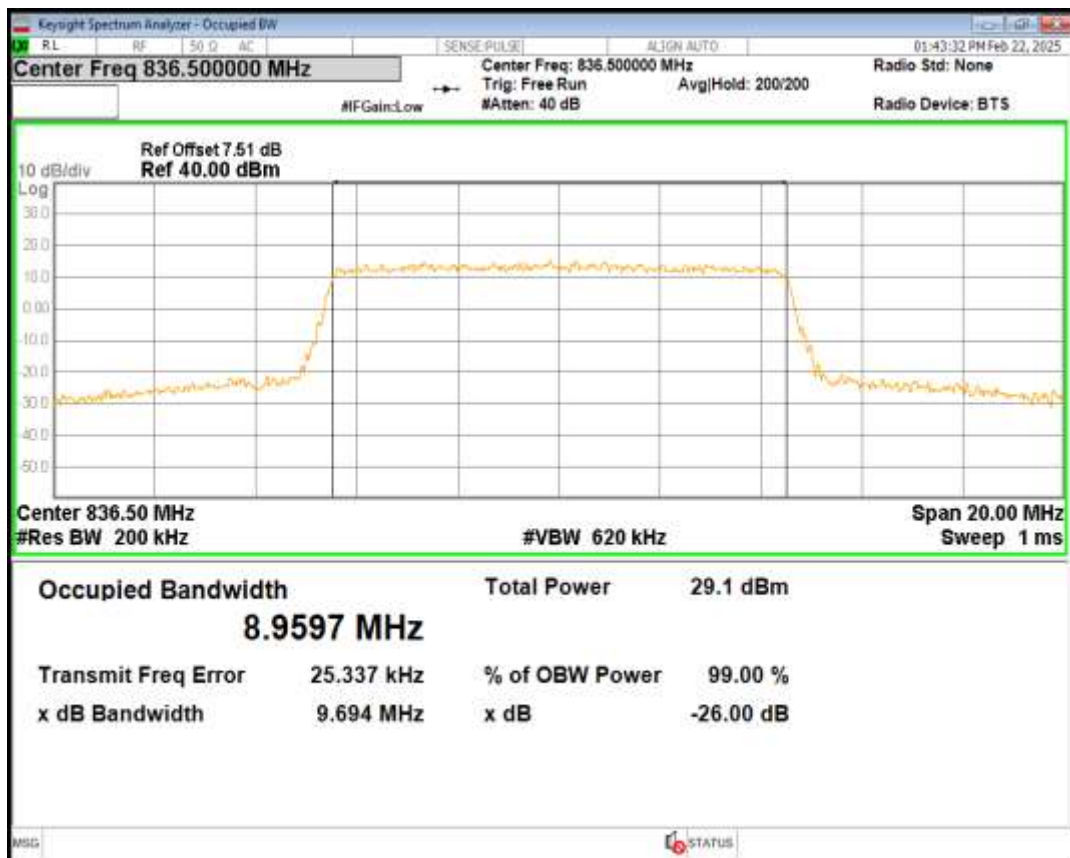
Band5 QPSK BW=10MHz Channel=20600 RB Size=50 Position=#0
