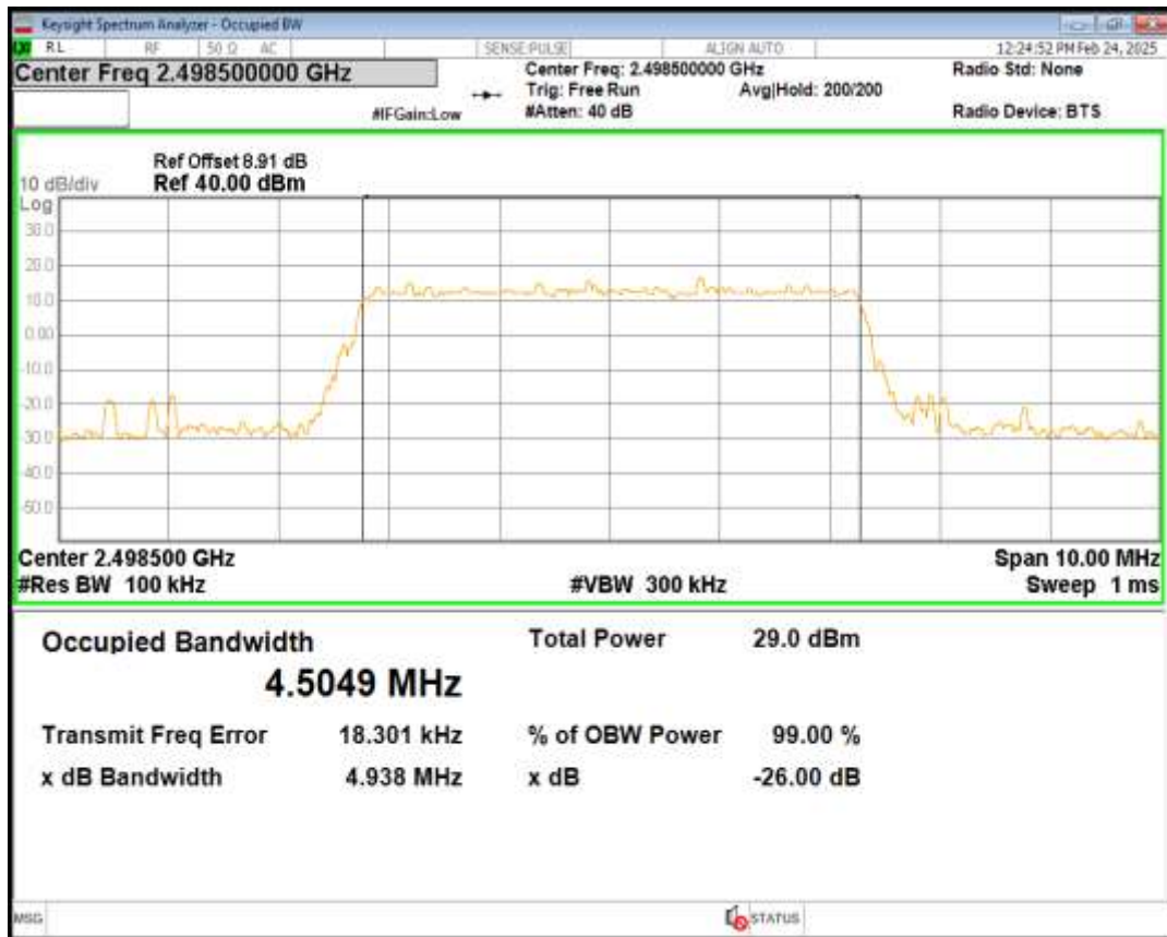
Band41 16QAM BW=5MHz Channel=39675 RB Size=25 Position=#0
