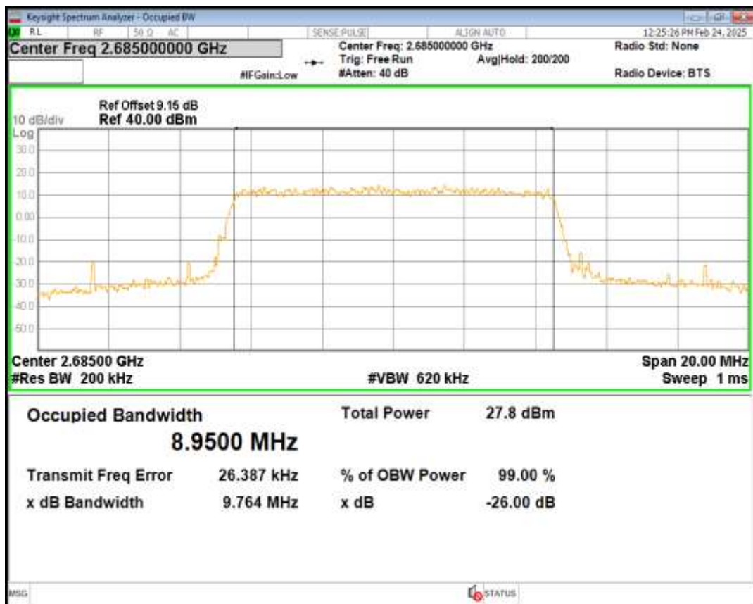
Band41 QPSK BW=15MHz Channel=39725 RB Size=75 Position=#0
