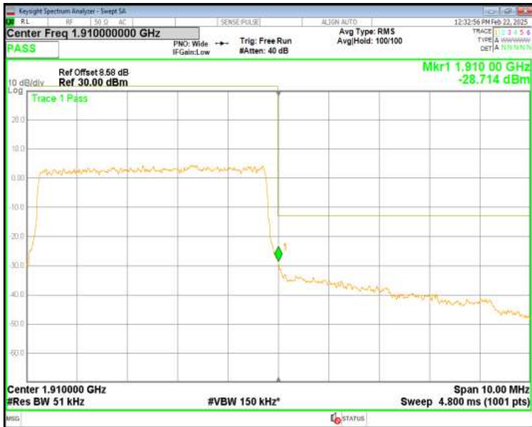
Band2 16QAM BW=5MHz Channel=19175 RB Size=25 Position=#0
