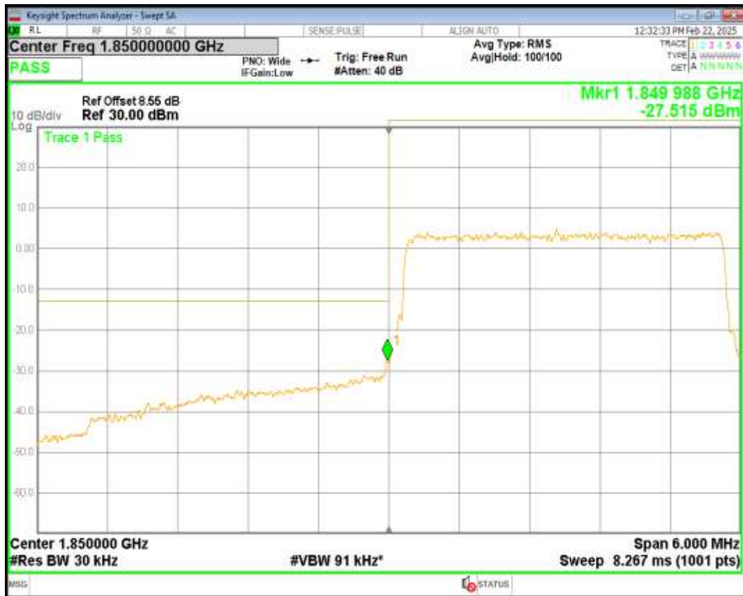
Band2 16QAM BW=3MHz Channel=18615 RB Size=15 Position=#0
