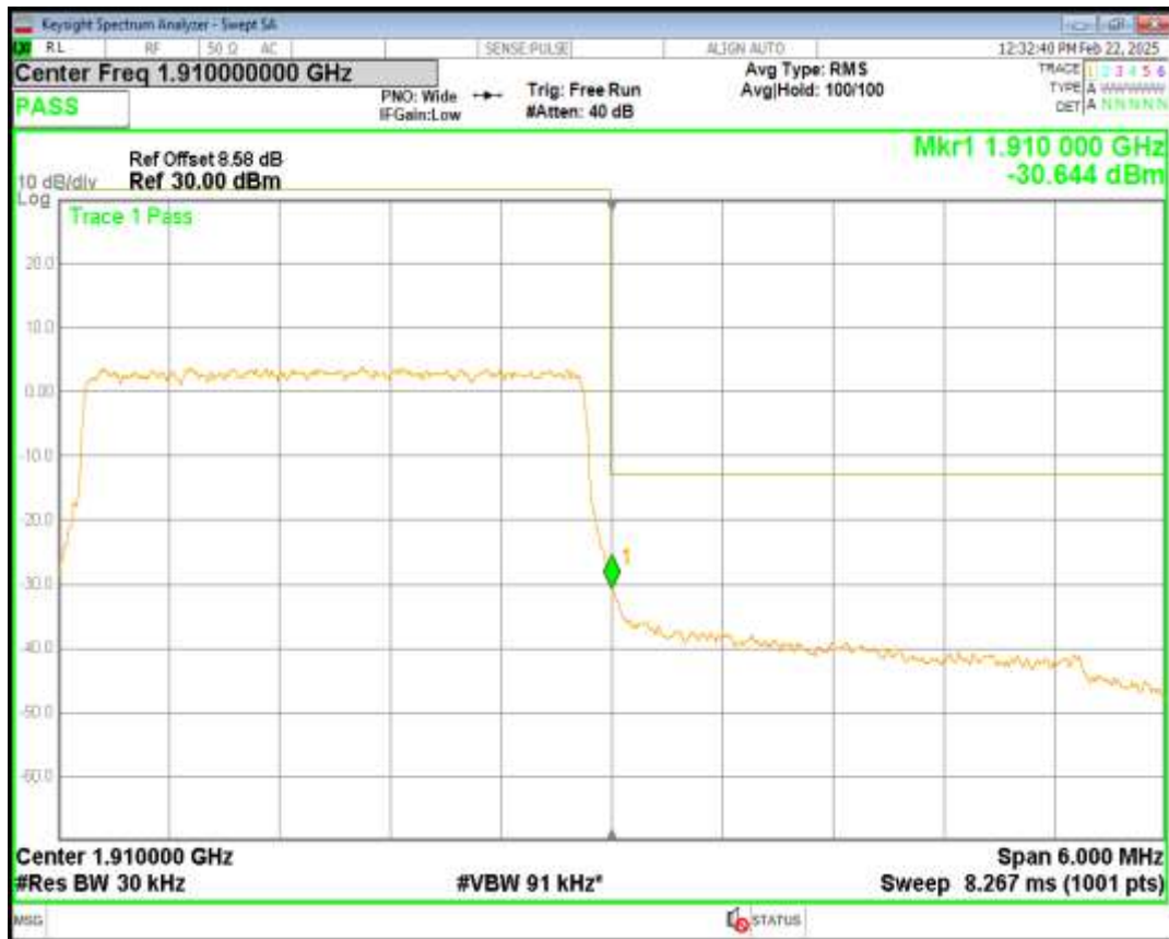
Band2 16QAM BW=3MHz Channel=19185 RB Size=15 Position=#0
