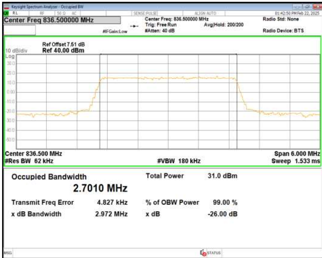
Band5 16QAM BW=3MHz Channel=20525 RB Size=15 Position=#0
