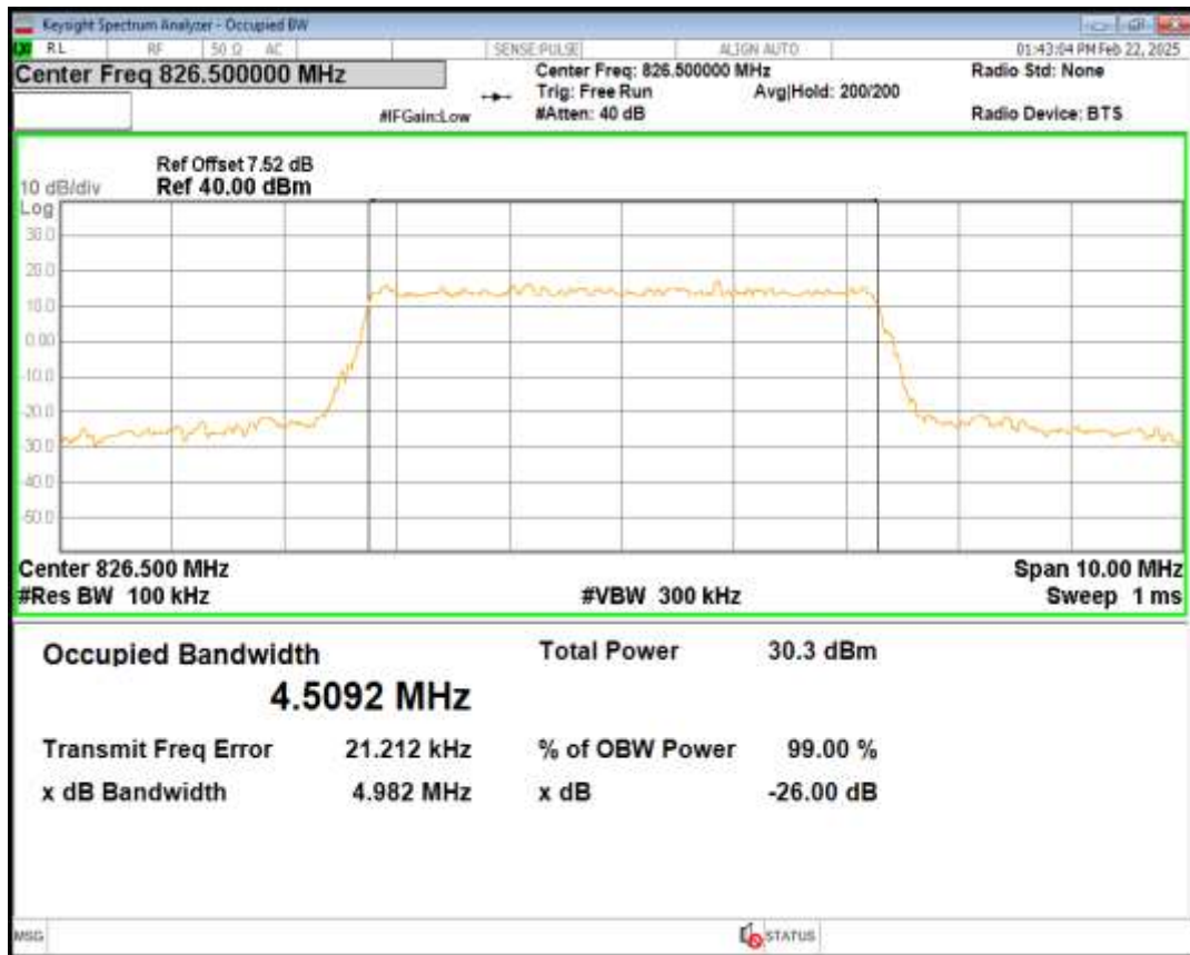
Band5 16QAM BW=5MHz Channel=20425 RB Size=25 Position=#0
