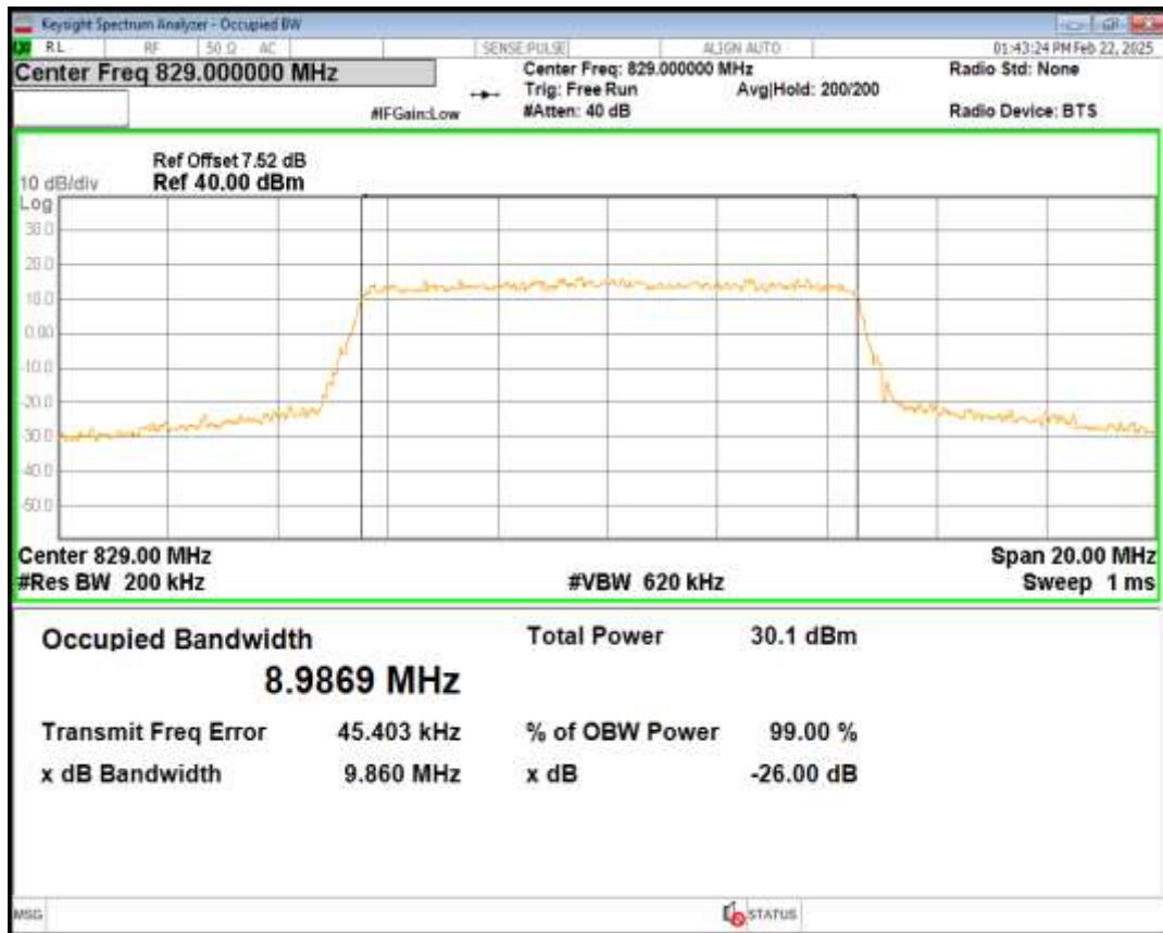
Band5 16QAM BW=10MHz Channel=20450 RB Size=50 Position=#0
