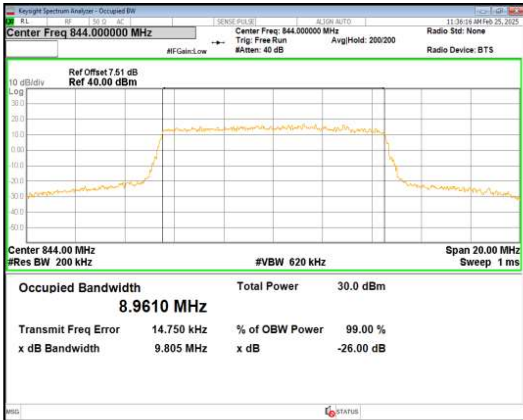
Band26(824-849) 16QAM BW=10MHz Channel=26990 RB Size=50 Position=#0
