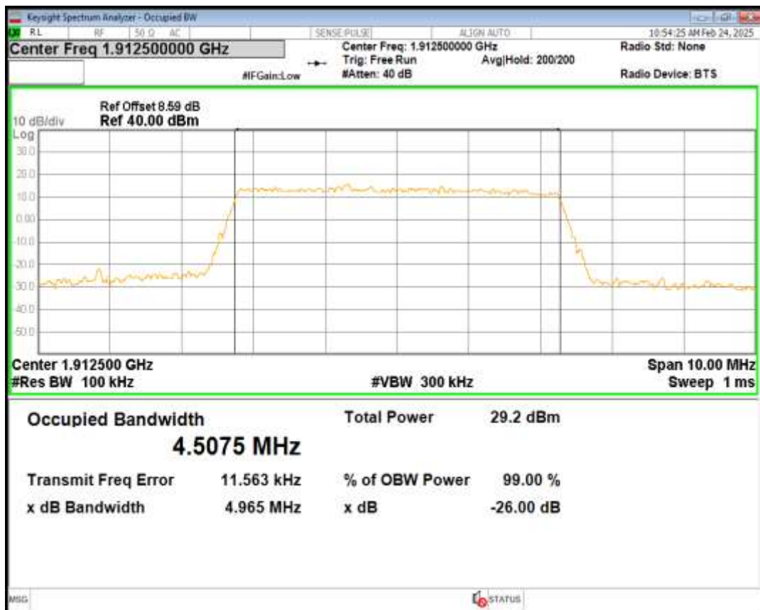
Band25 QPSK BW=10MHz Channel=26090 RB Size=50 Position=#0
