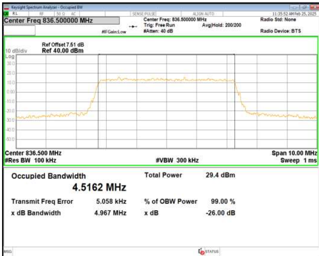
Band26(824-849) QPSK BW=5MHz Channel=27015 RB Size=25 Position=#0
