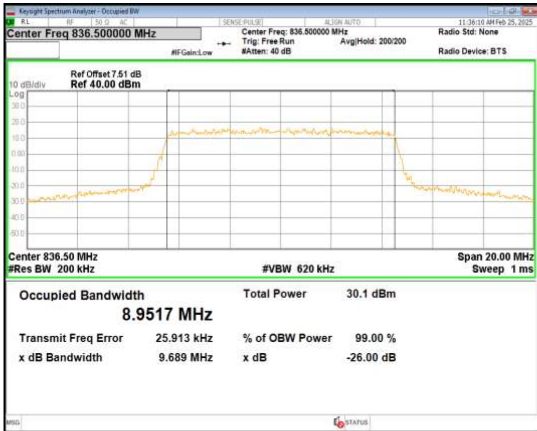
Band26(824-849) 16QAM BW=10MHz Channel=26915 RB Size=50 Position=#0
