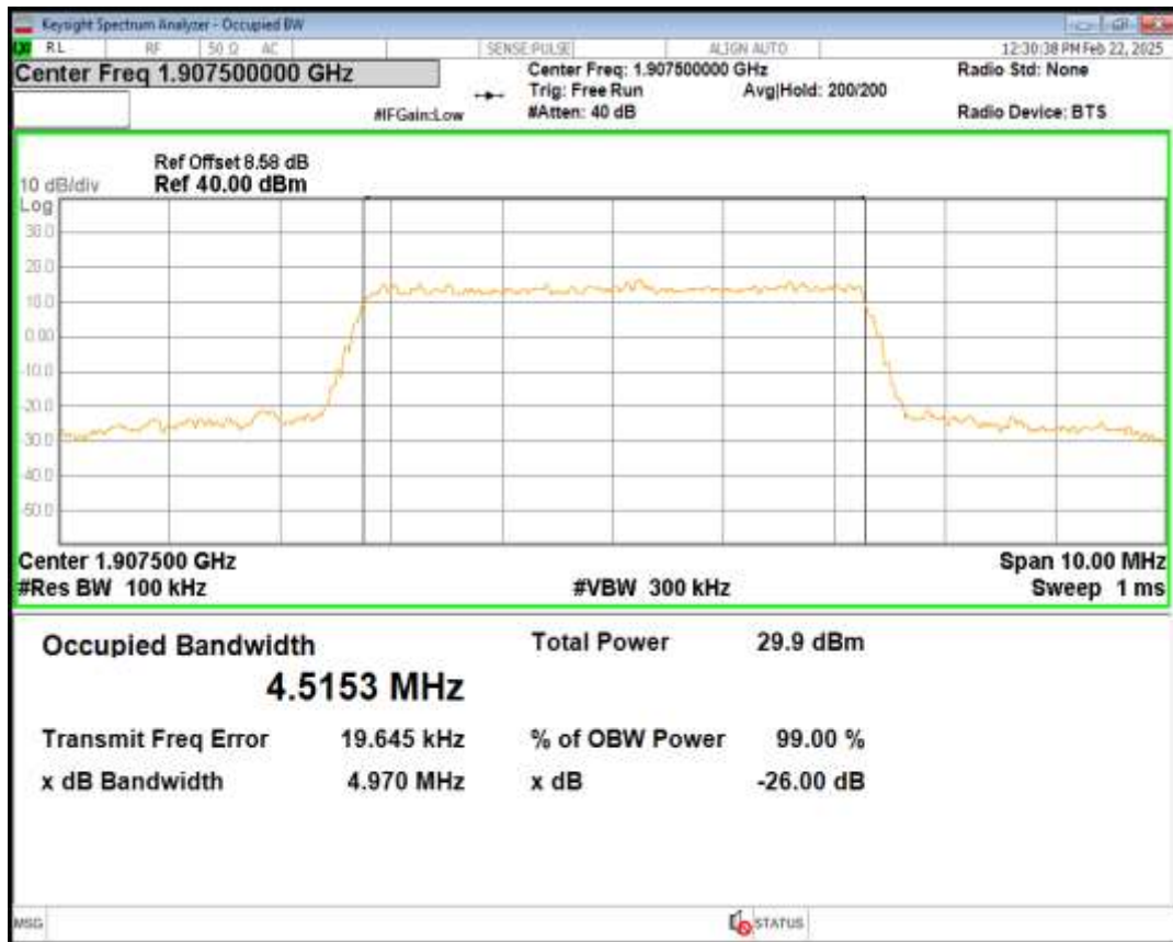
Band2 16QAM BW=5MHz Channel=19175 RB Size=25 Position=#0
