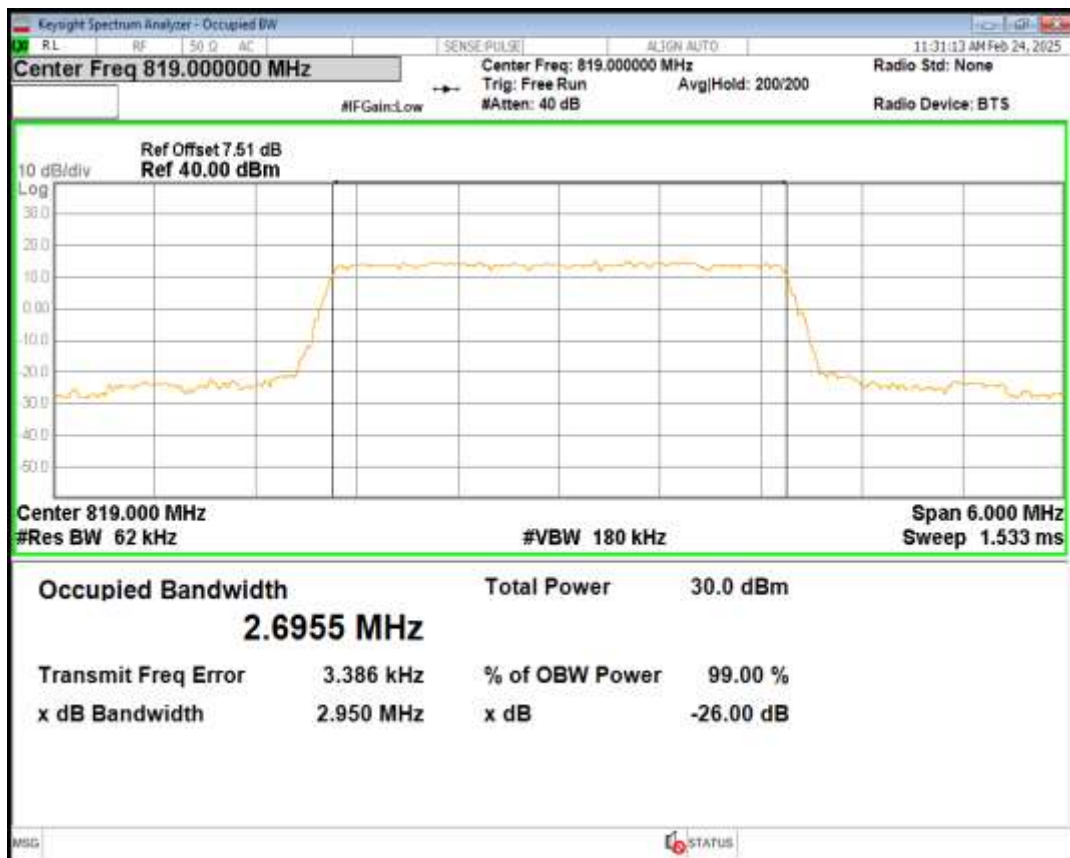
Band26(814-824) QPSK BW=3MHz Channel=26775 RB Size=15 Position=#0
