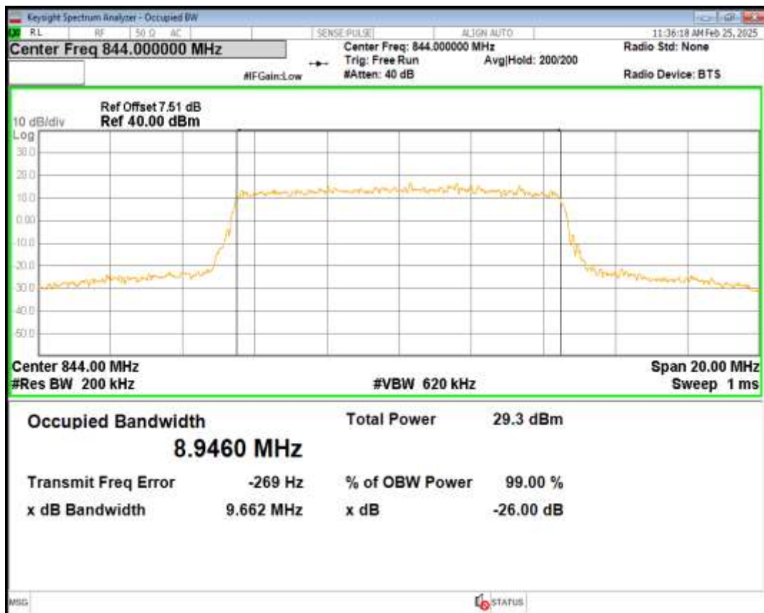
Band26(824-849) QPSK BW=15MHz Channel=26865 RB Size=75 Position=#0
