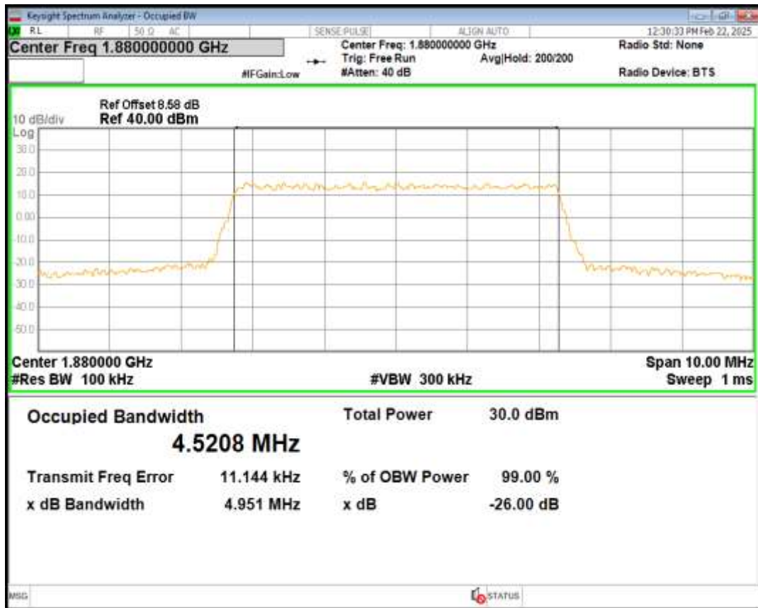
Band2 16QAM BW=5MHz Channel=18900 RB Size=25 Position=#0
