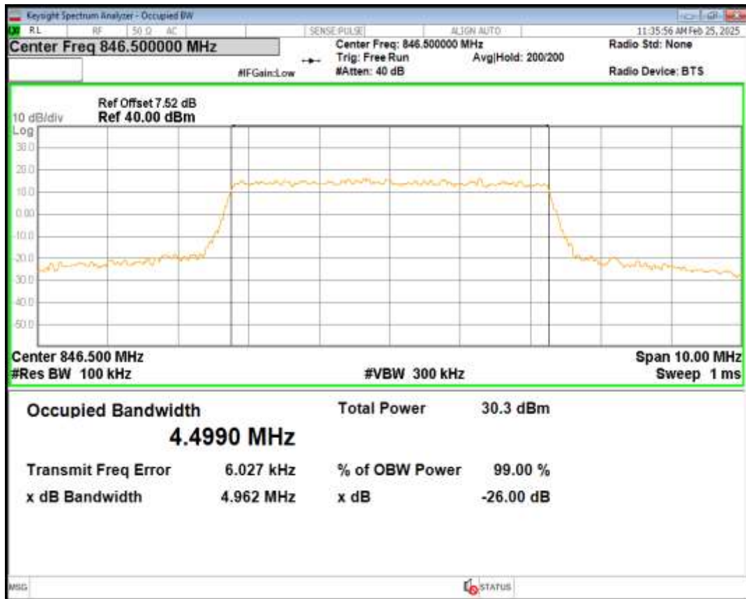
Band26(824-849) 16QAM BW=5MHz Channel=27015 RB Size=25 Position=#0
