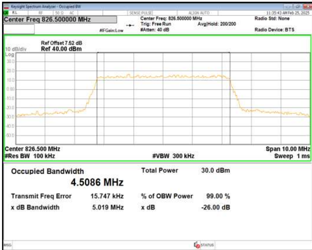
Band26(824-849) 16QAM BW=5MHz Channel=26815 RB Size=25 Position=#0
