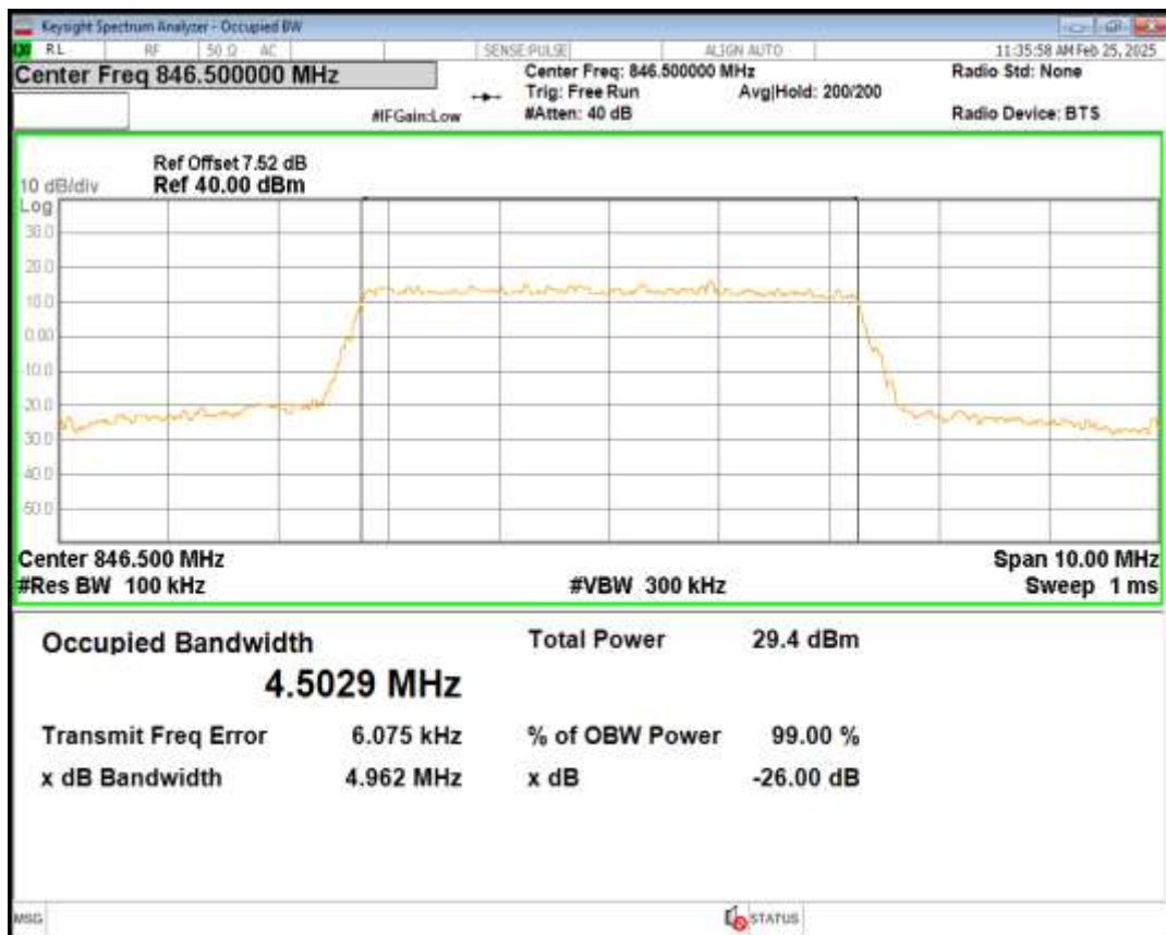
Band26(824-849) QPSK BW=10MHz Channel=26840 RB Size=50 Position=#0
