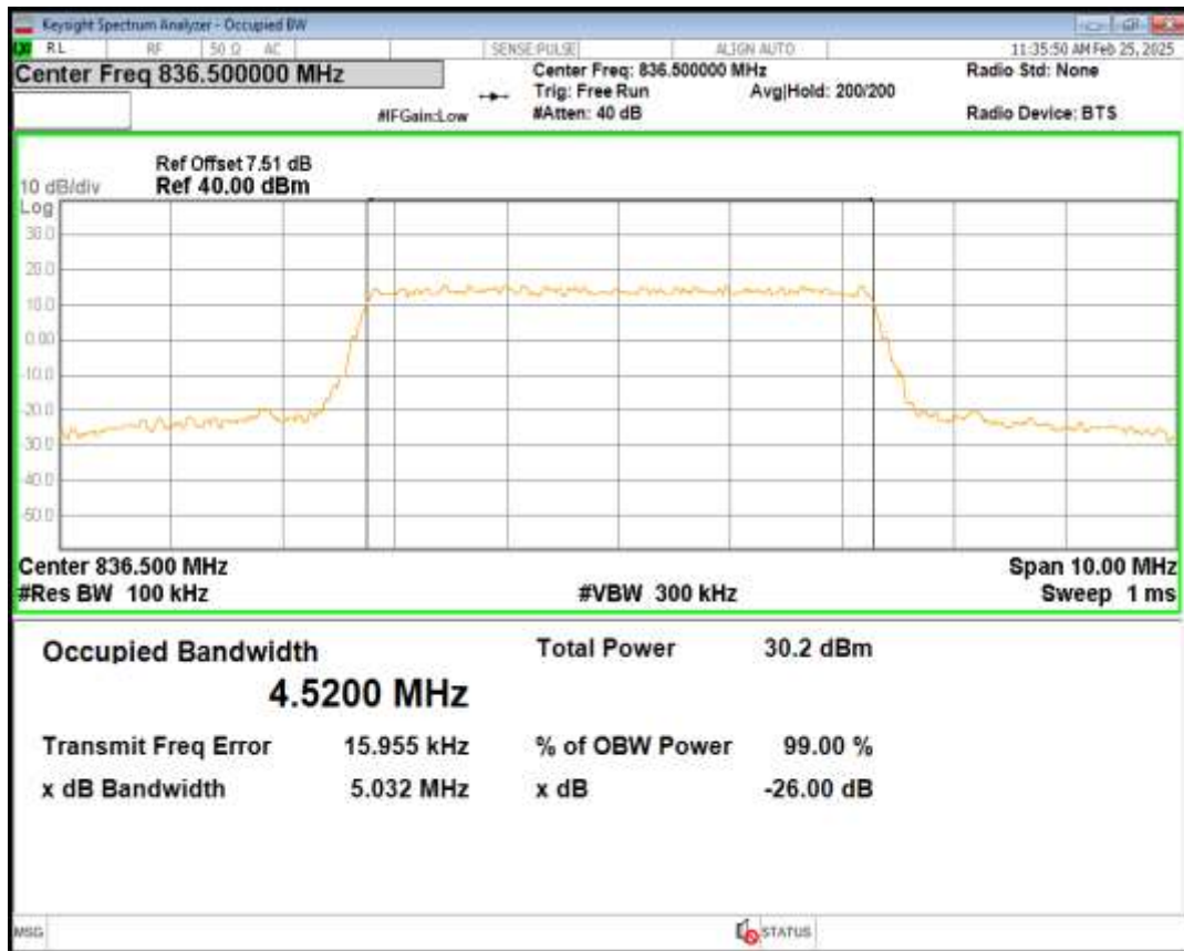
Band26(824-849) 16QAM BW=5MHz Channel=26915 RB Size=25 Position=#0
