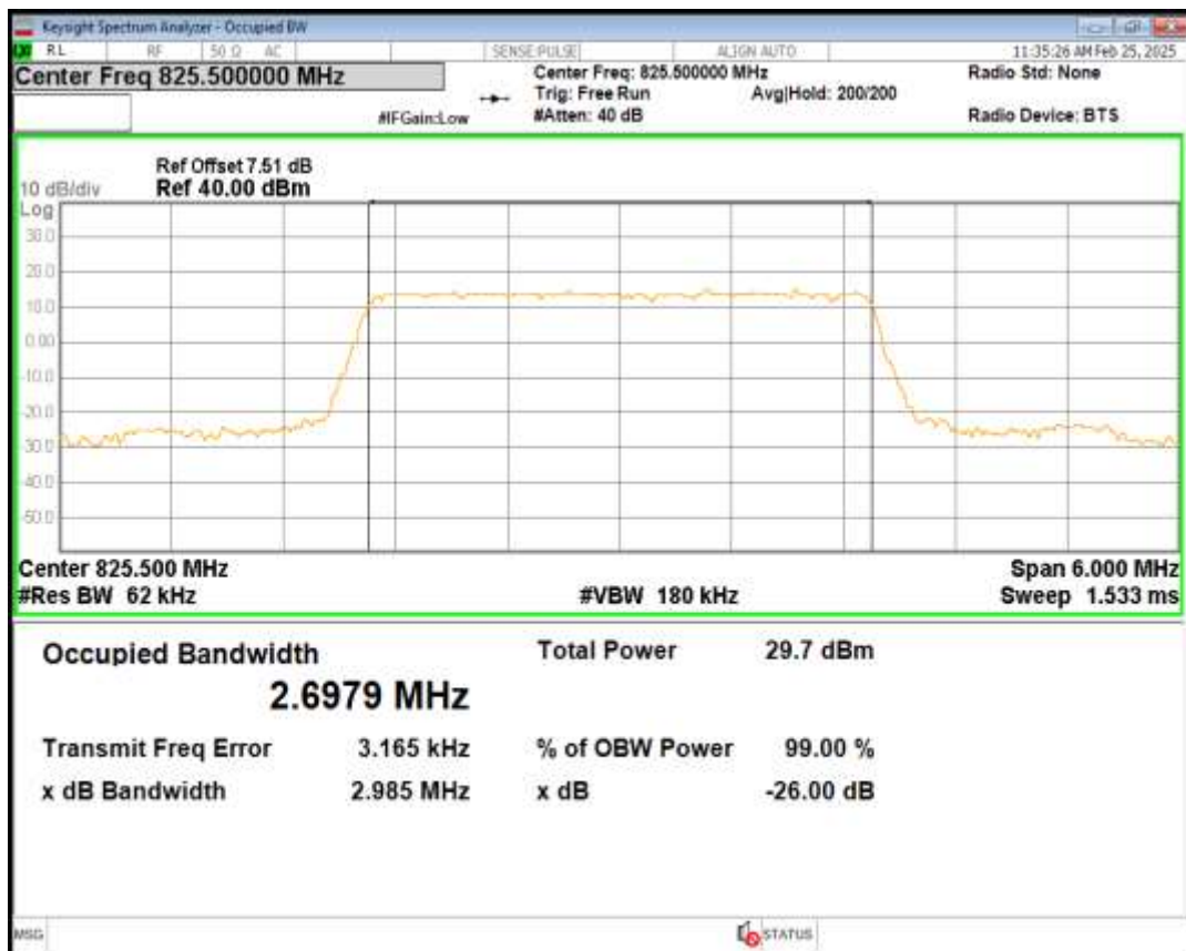
Band26(824-849) QPSK BW=3MHz Channel=26915 RB Size=15 Position=#0
