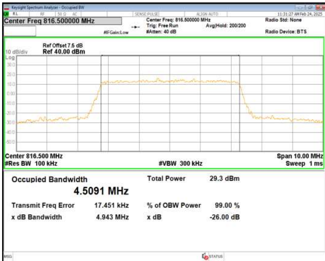
Band26(814-824) QPSK BW=5MHz Channel=26740 RB Size=25 Position=#0
