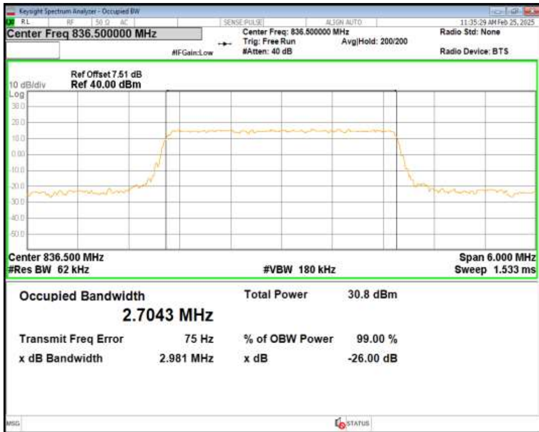
Band26(824-849) 16QAM BW=3MHz Channel=26915 RB Size=15 Position=#0
