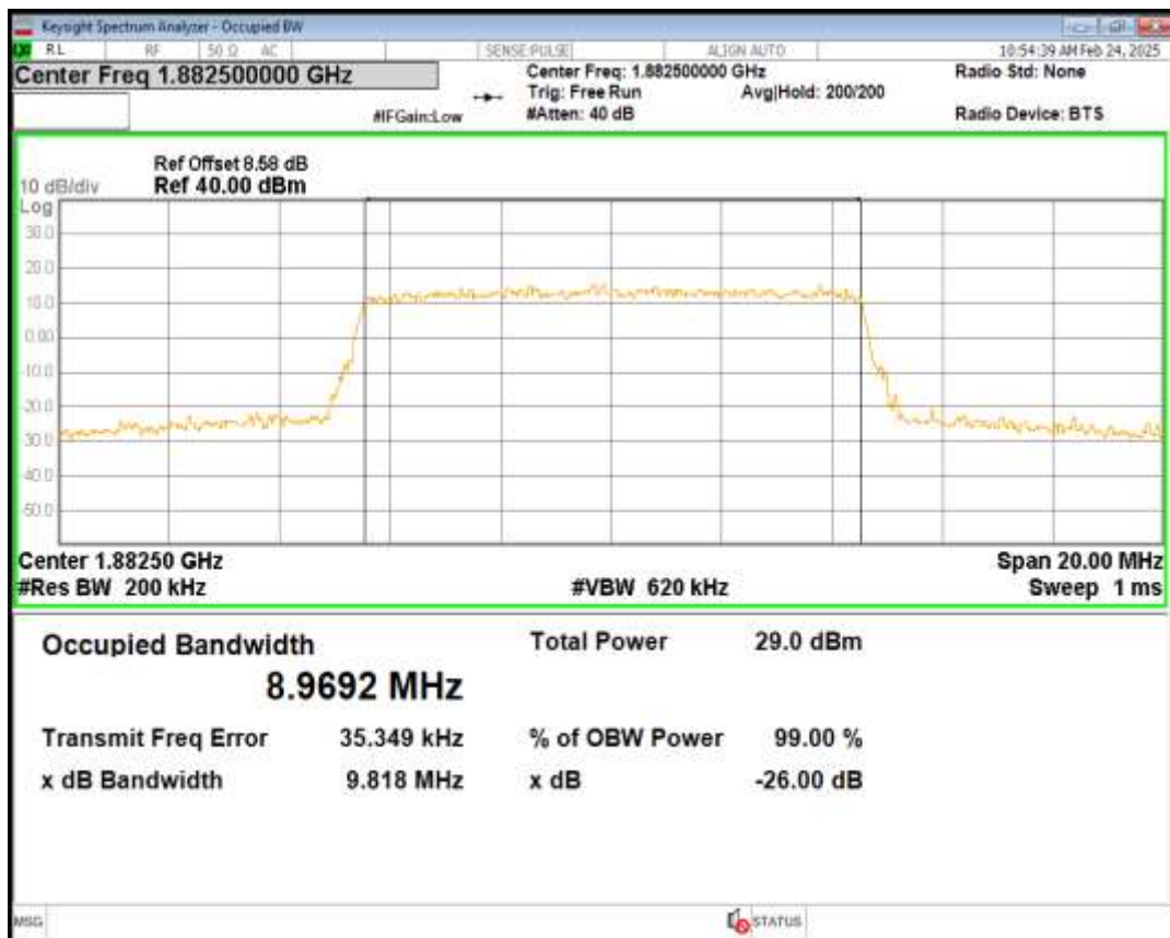
Band25 QPSK BW=10MHz Channel=26640 RB Size=50 Position=#0
