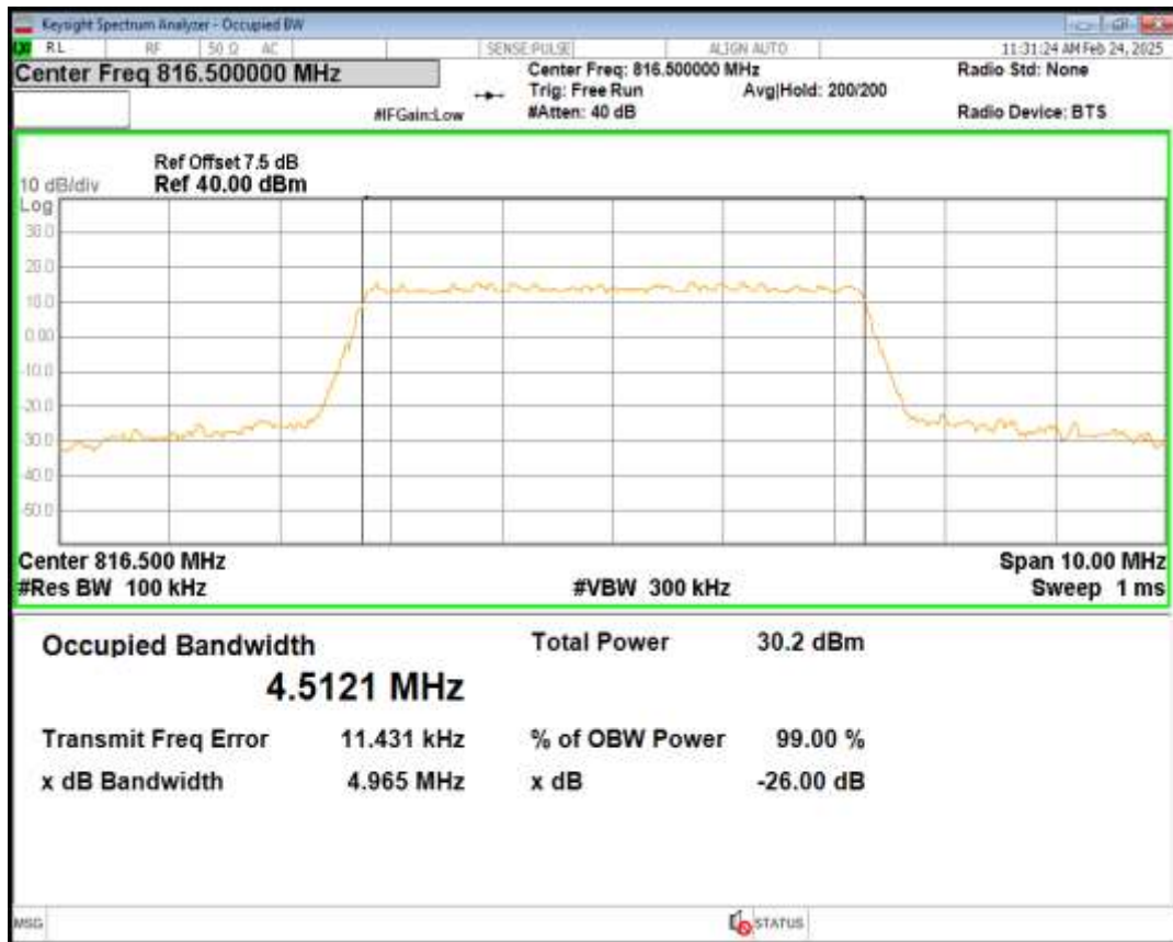
Band26(814-824) 16QAM BW=5MHz Channel=26715 RB Size=25 Position=#0
