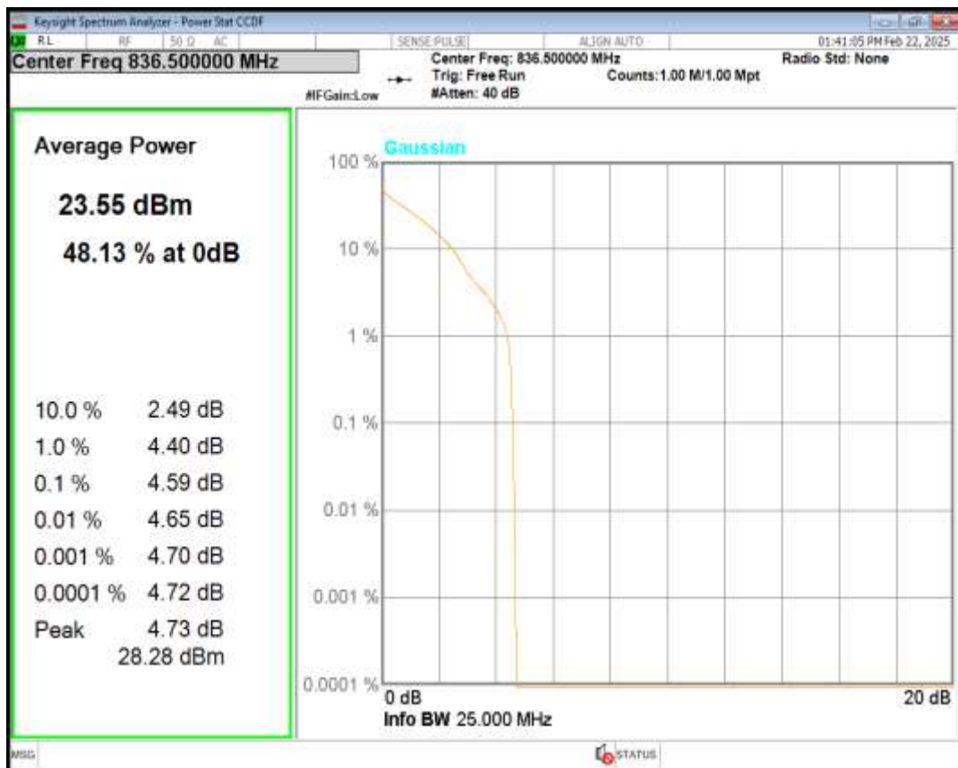
Band5 16QAM BW=3MHz Channel=20525 RB Size=1 Position=#0
