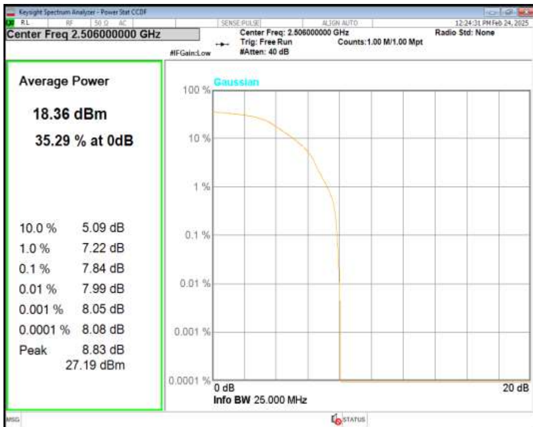
Band41 16QAM BW=20MHz Channel=39750 RB Size=1 Position=#0
