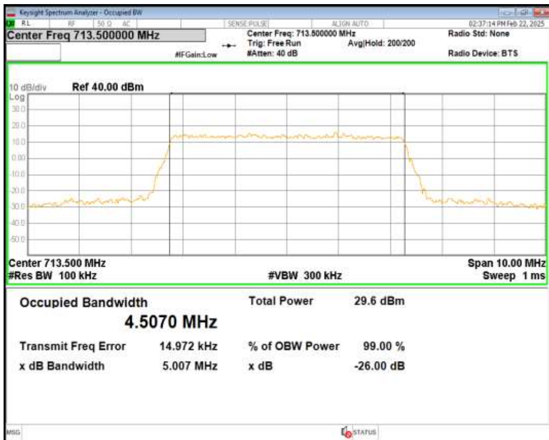
Band12 QPSK BW=10MHz Channel=23060 RB Size=50 Position=#0
