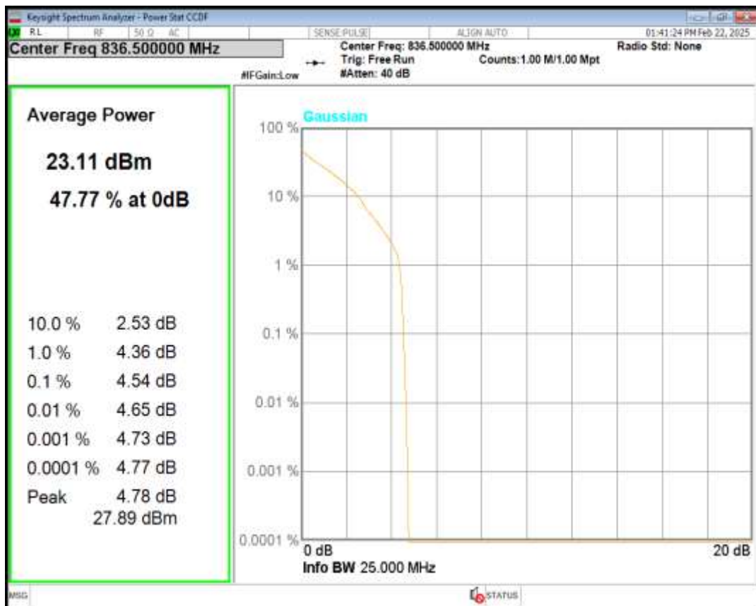
Band5 16QAM BW=5MHz Channel=20525 RB Size=1 Position=#0
