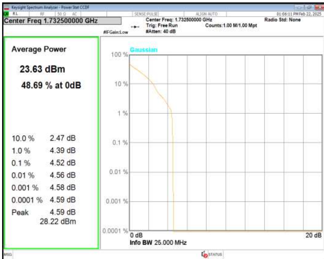
Band4 16QAM BW=15MHz Channel=20175 RB Size=1 Position=#0
