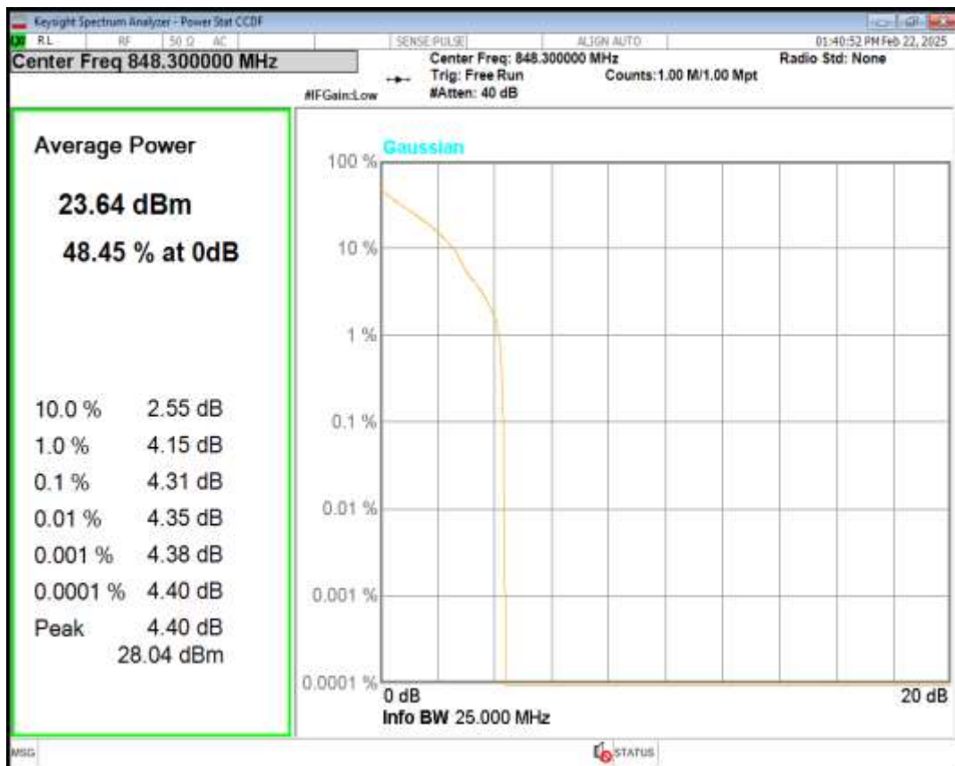
Band5 16QAM BW=1.4MHz Channel=20643 RB Size=1 Position=#0
