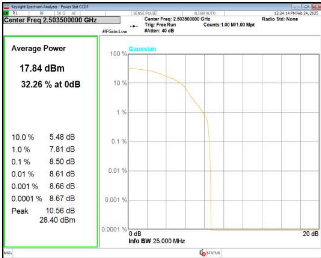
Band41 QPSK BW=15MHz Channel=40620 RB Size=1 Position=#0
