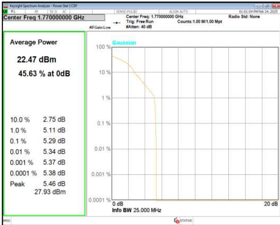
Band7 QPSK BW=5MHz Channel=20775 RB Size=1 Position=#0
