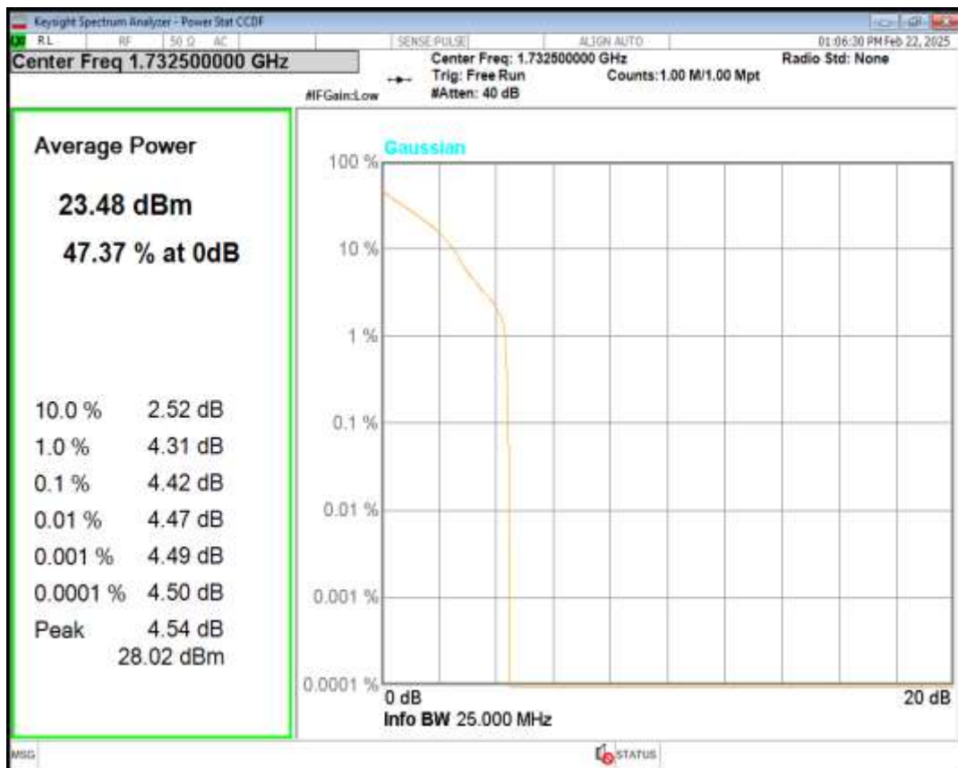
Band4 16QAM BW=20MHz Channel=20175 RB Size=1 Position=#0
