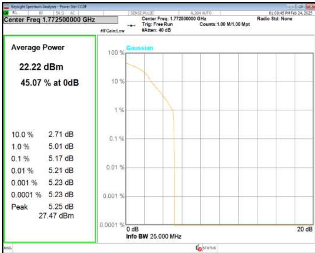
Band66 QPSK BW=20MHz Channel=132072 RB Size=1 Position=#0
