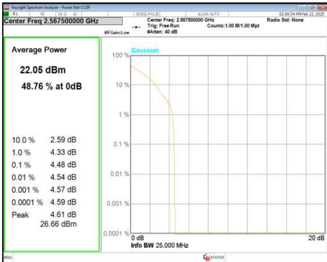
Band7 16QAM BW=5MHz Channel=21425 RB Size=1 Position=#0
