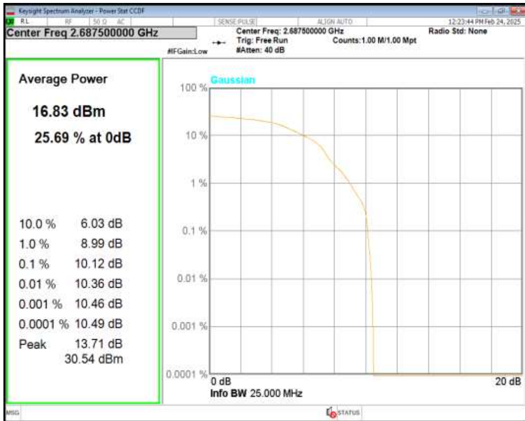
Band41 QPSK BW=10MHz Channel=39700 RB Size=1 Position=#0
