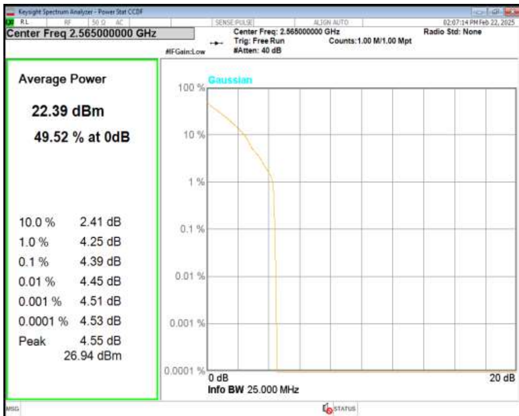
Band7 16QAM BW=10MHz Channel=21400 RB Size=1 Position=#0
