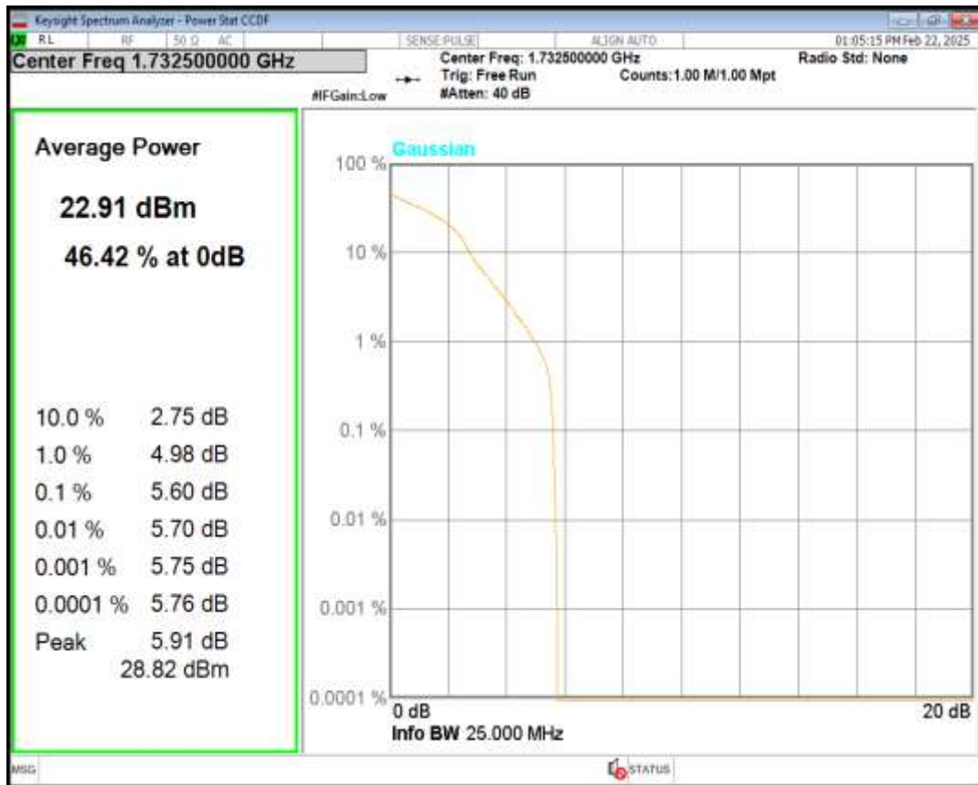
Band4 QPSK BW=3MHz Channel=20385 RB Size=1 Position=#0
