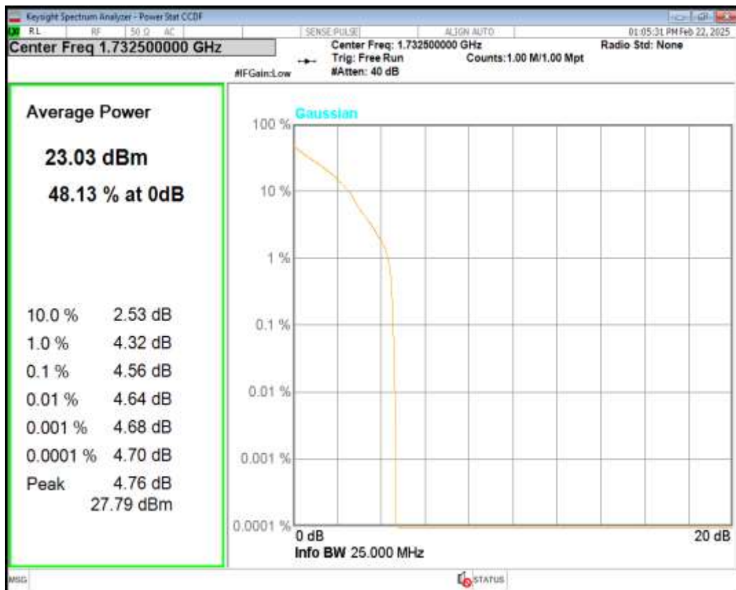
Band4 16QAM BW=5MHz Channel=20175 RB Size=1 Position=#0
