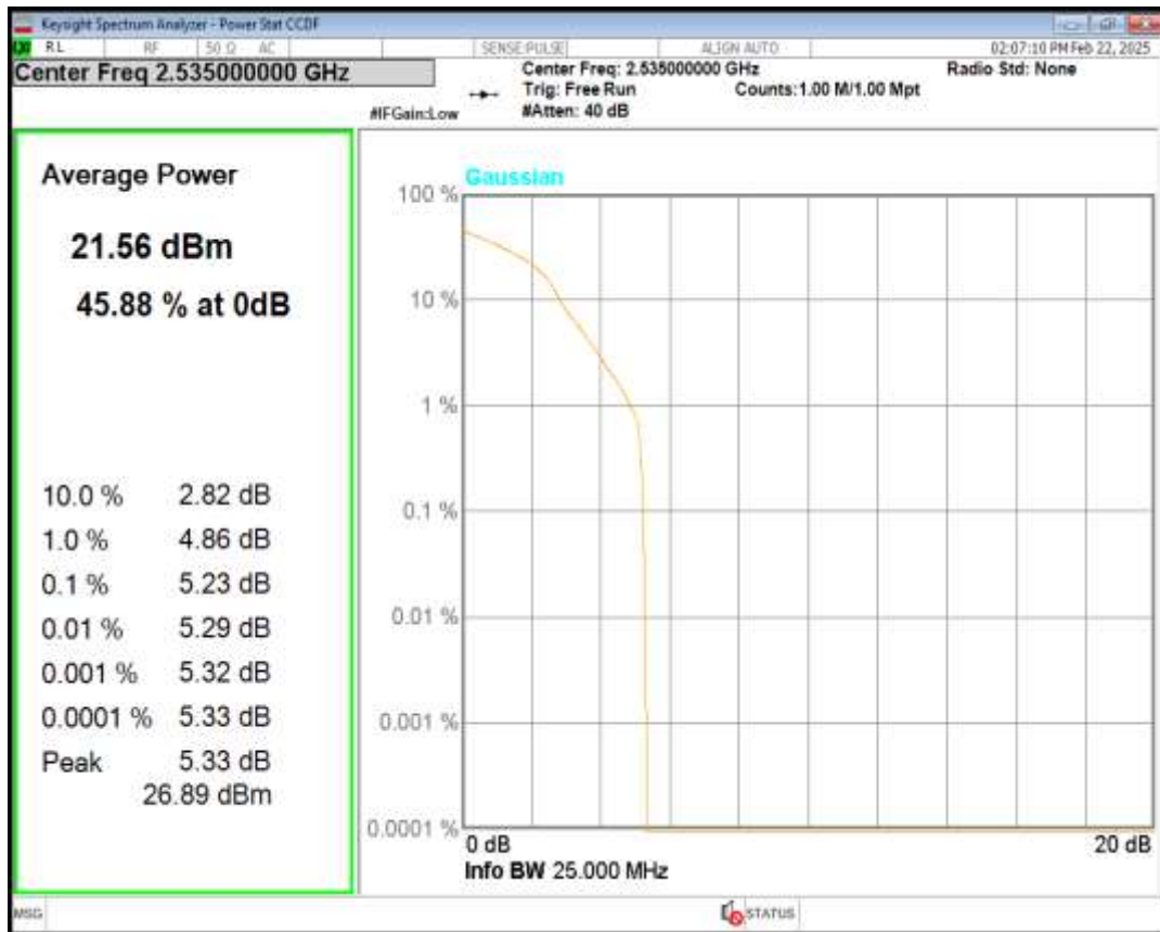
Band7 QPSK BW=10MHz Channel=21400 RB Size=1 Position=#0
