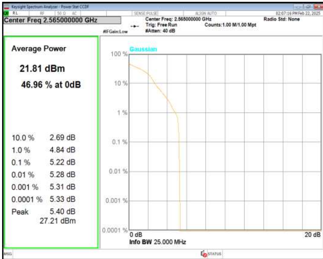
Band7 QPSK BW=15MHz Channel=20825 RB Size=1 Position=#0
