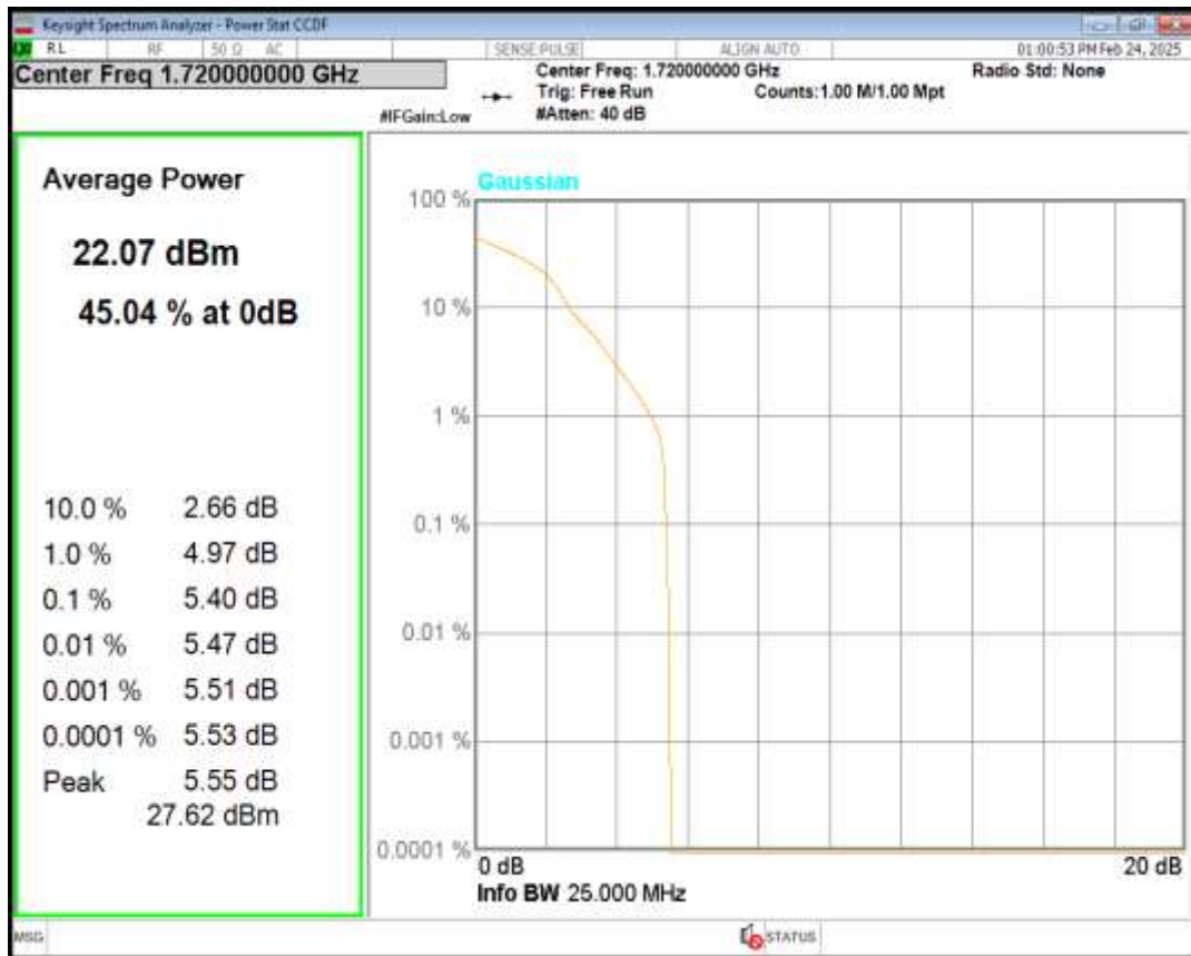
Band66 QPSK BW=20MHz Channel=132322 RB Size=1 Position=#0
