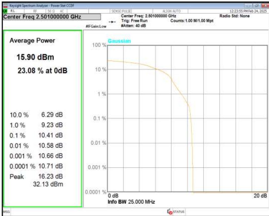
Band41 QPSK BW=10MHz Channel=40620 RB Size=1 Position=#0
