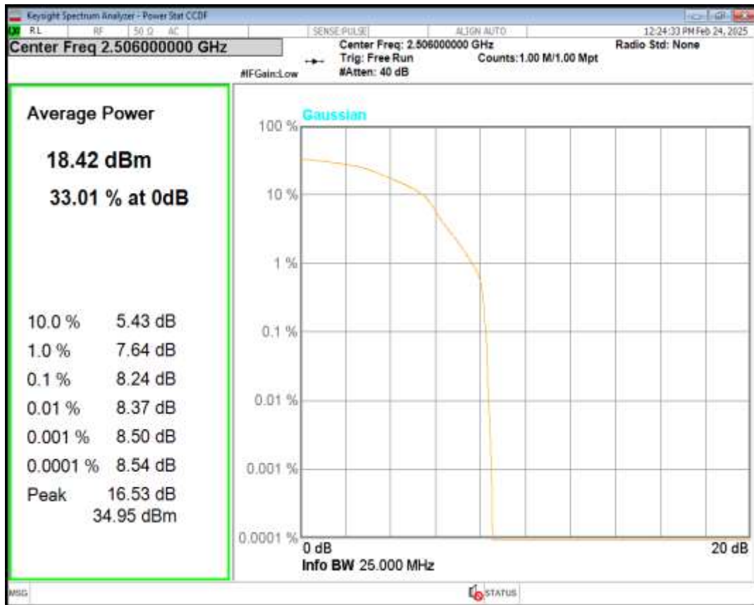
Band41 QPSK BW=20MHz Channel=40620 RB Size=1 Position=#0
