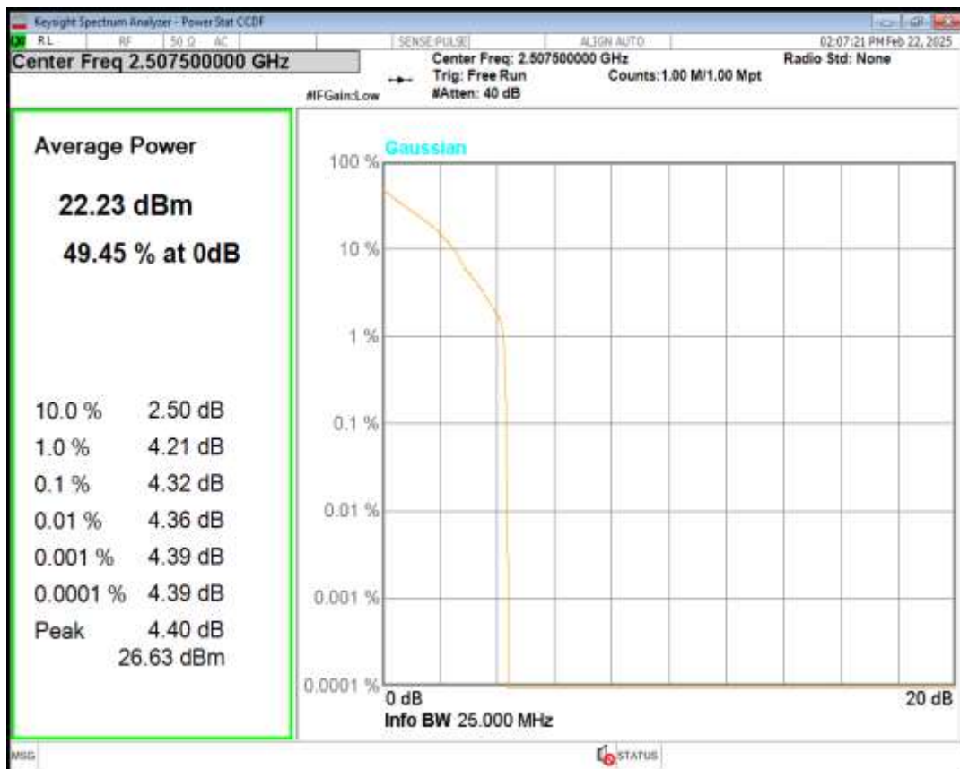
Band7 16QAM BW=15MHz Channel=20825 RB Size=1 Position=#0
