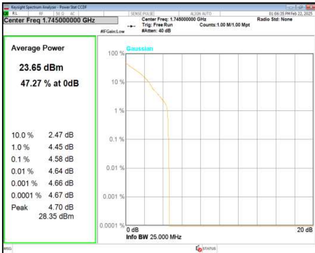
Band4 16QAM BW=20MHz Channel=20300 RB Size=1 Position=#0
