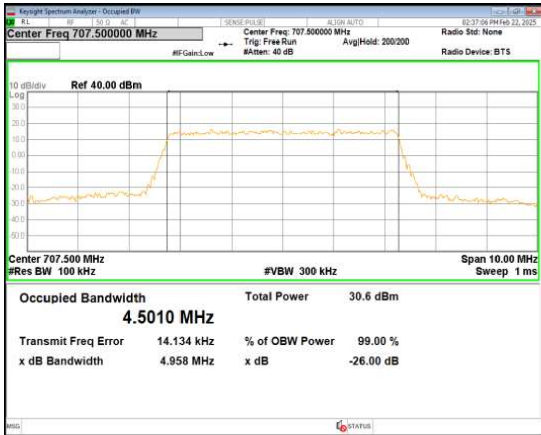
Band12 16QAM BW=5MHz Channel=23095 RB Size=25 Position=#0
