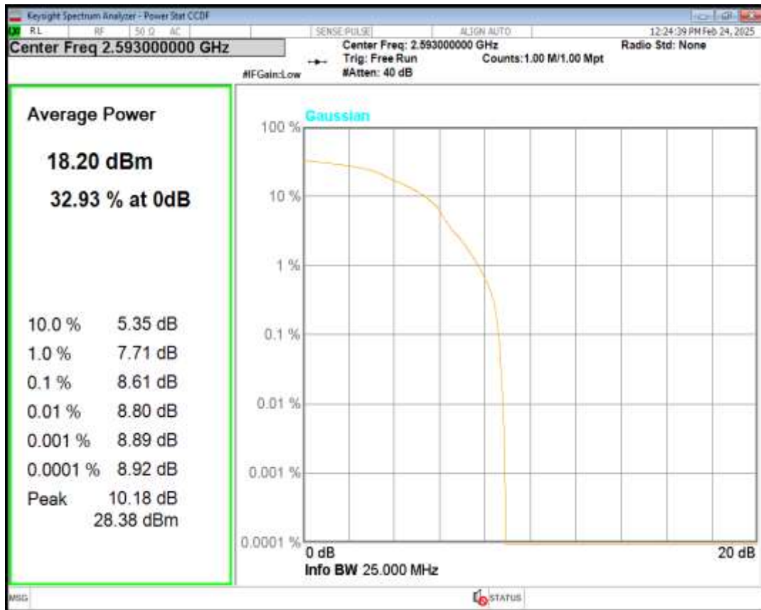
Band41 QPSK BW=20MHz Channel=41490 RB Size=1 Position=#0
