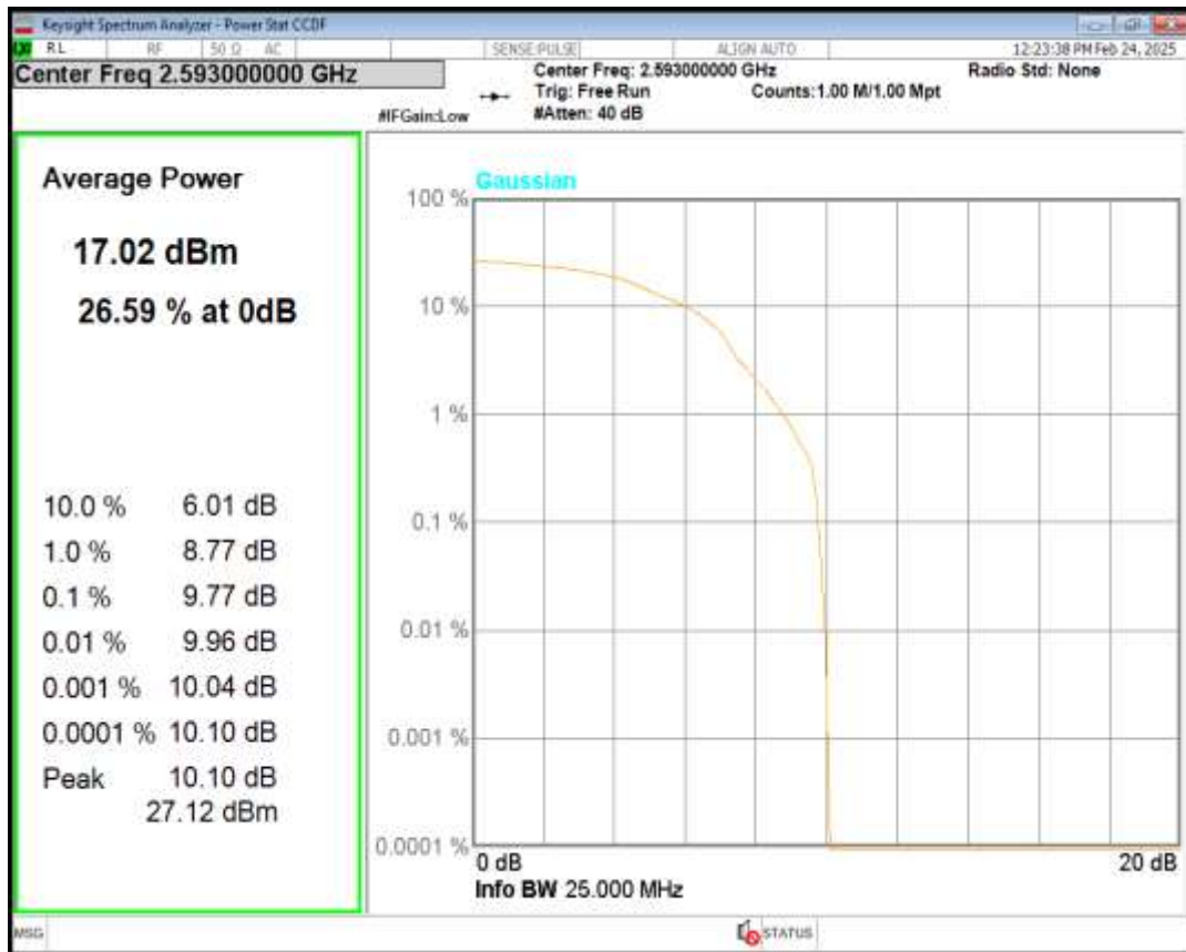
Band41 QPSK BW=5MHz Channel=41565 RB Size=1 Position=#0
