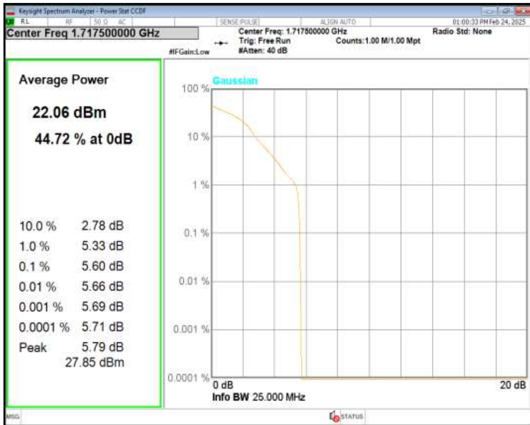
Band66 QPSK BW=15MHz Channel=132322 RB Size=1 Position=#0
