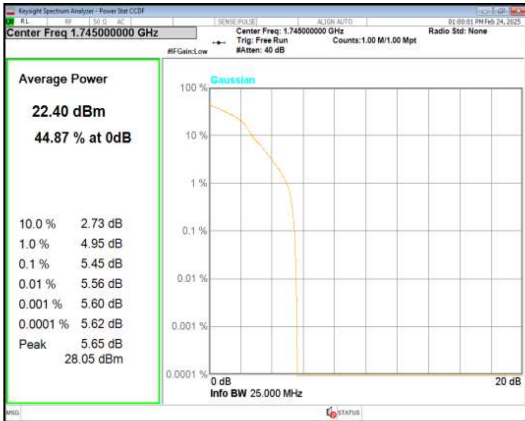
Band66 QPSK BW=5MHz Channel=132647 RB Size=1 Position=#0
