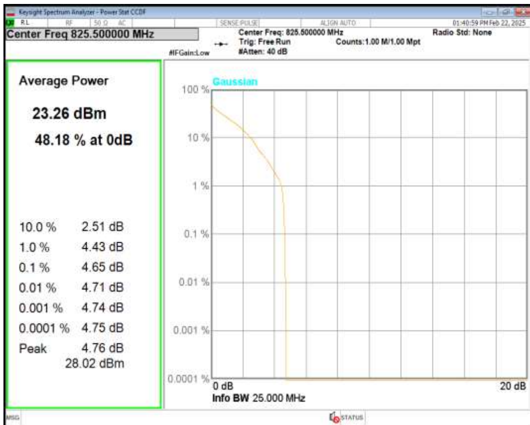
Band5 16QAM BW=3MHz Channel=20415 RB Size=1 Position=#0
