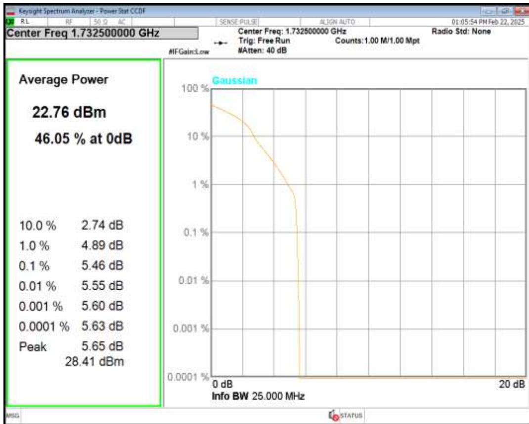
Band4 QPSK BW=10MHz Channel=20350 RB Size=1 Position=#0
