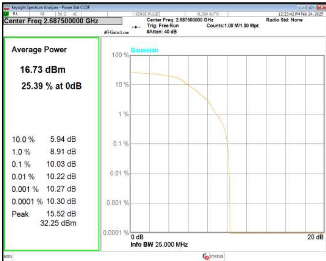
Band41 16QAM BW=5MHz Channel=41565 RB Size=1 Position=#0
