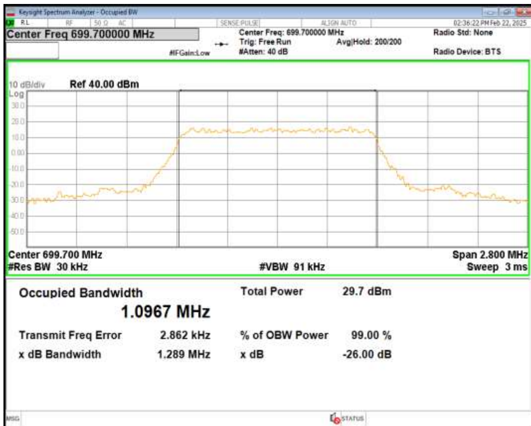
Band12 QPSK BW=1.4MHz Channel=23095 RB Size=6 Position=#0
