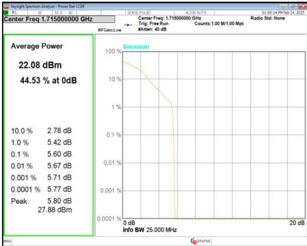
Band66 QPSK BW=10MHz Channel=132322 RB Size=1 Position=#0
