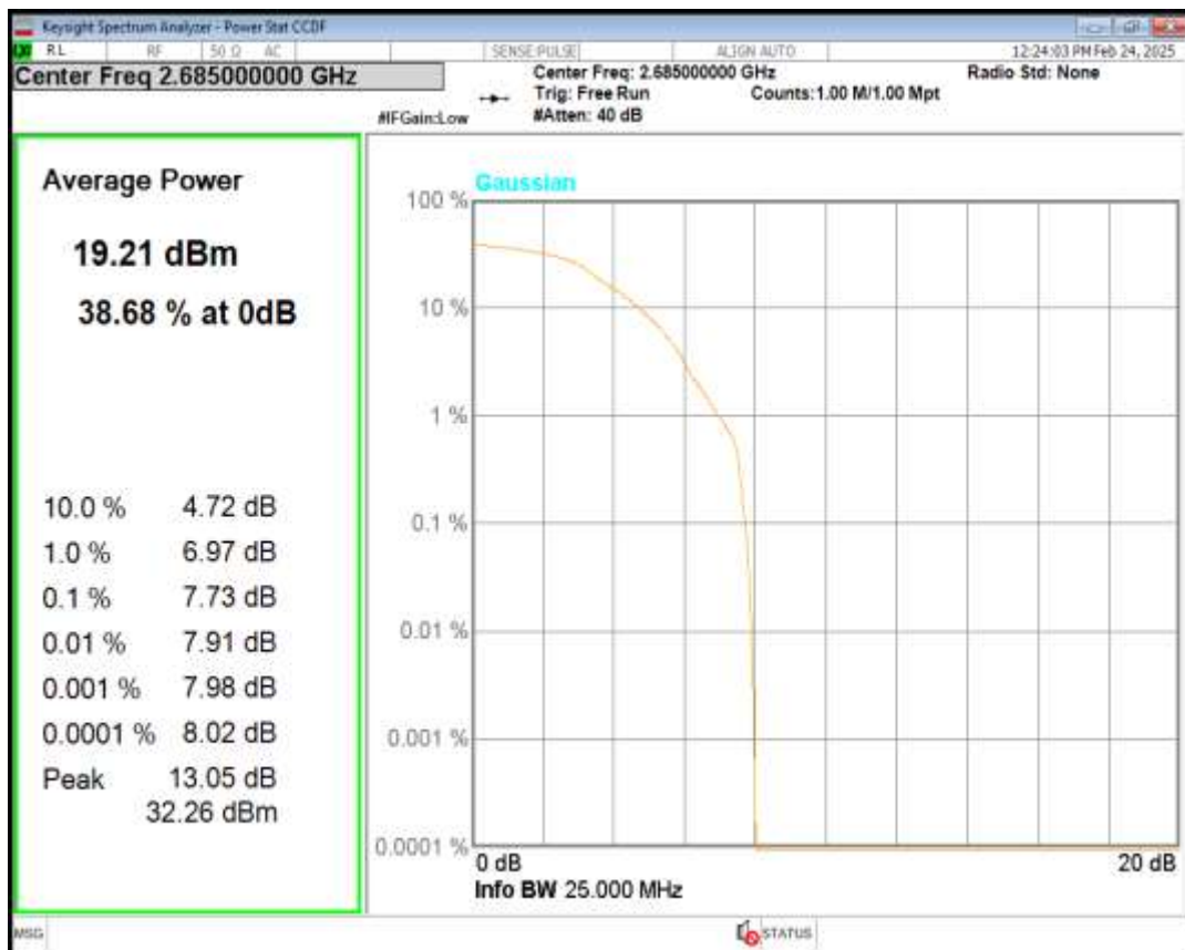
Band41 16QAM BW=10MHz Channel=41540 RB Size=1 Position=#0
