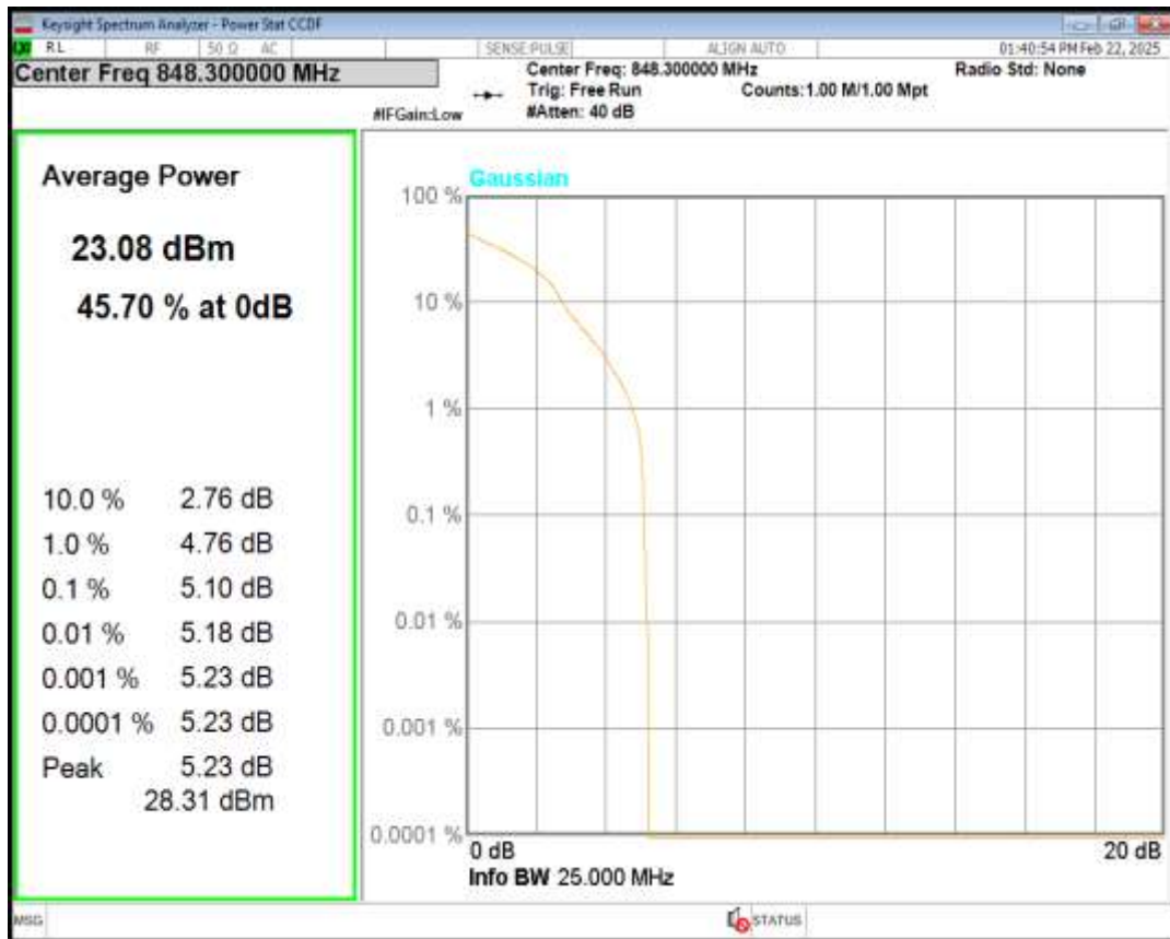
Band5 QPSK BW=3MHz Channel=20415 RB Size=1 Position=#0
