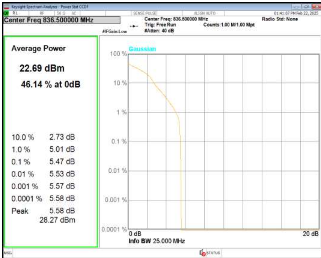
Band5 QPSK BW=3MHz Channel=20635 RB Size=1 Position=#0
