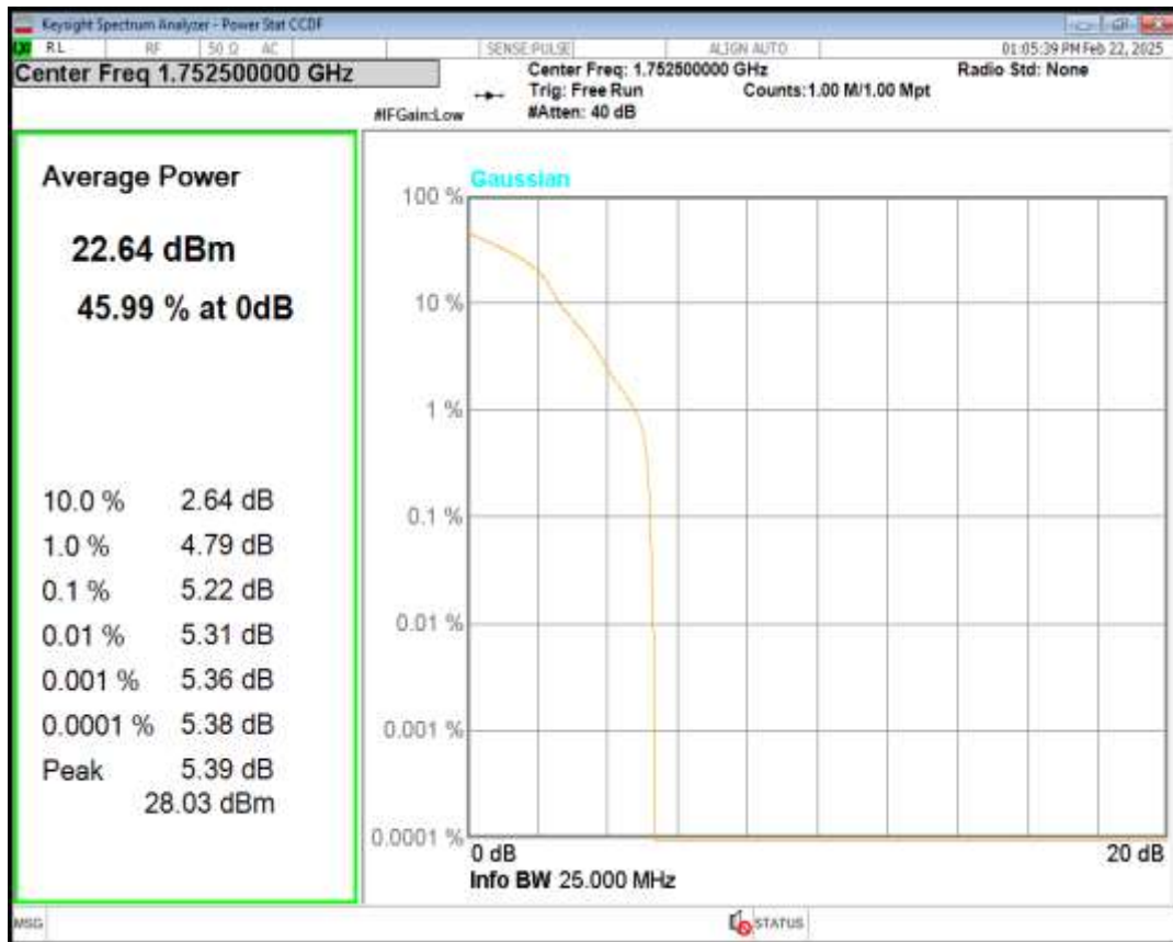
Band4 QPSK BW=10MHz Channel=20000 RB Size=1 Position=#0
