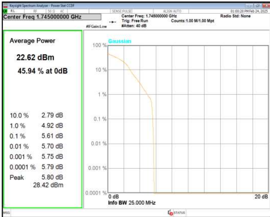
Band66 QPSK BW=10MHz Channel=132622 RB Size=1 Position=#0
