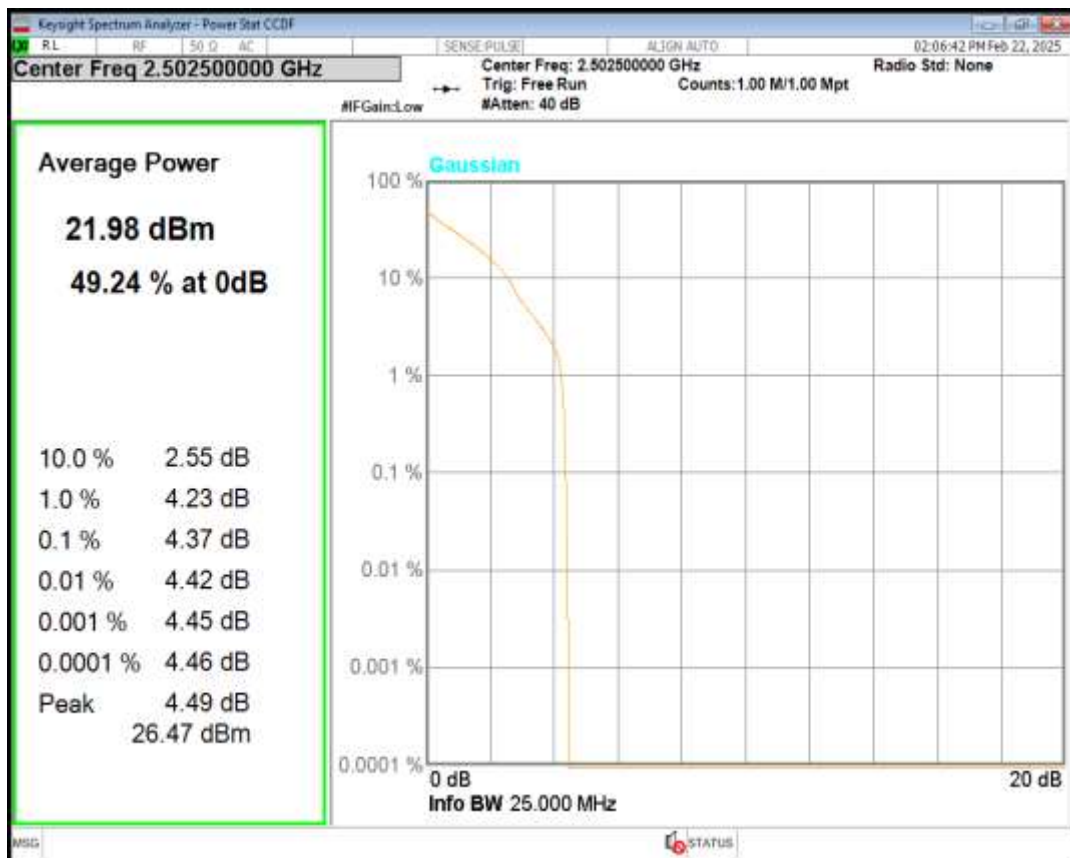
Band7 16QAM BW=5MHz Channel=20775 RB Size=1 Position=#0
