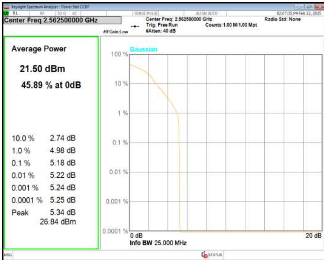
Band7 QPSK BW=20MHz Channel=20850 RB Size=1 Position=#0
