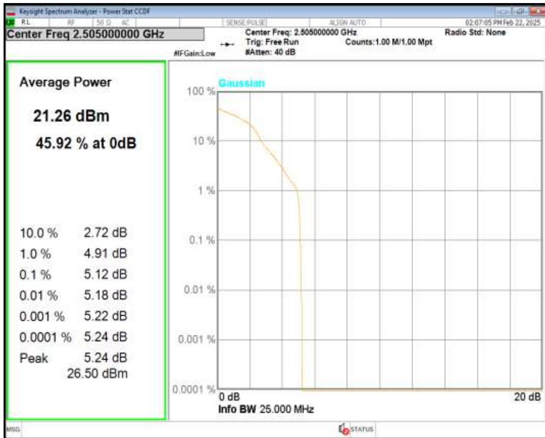
Band7 QPSK BW=10MHz Channel=21100 RB Size=1 Position=#0
