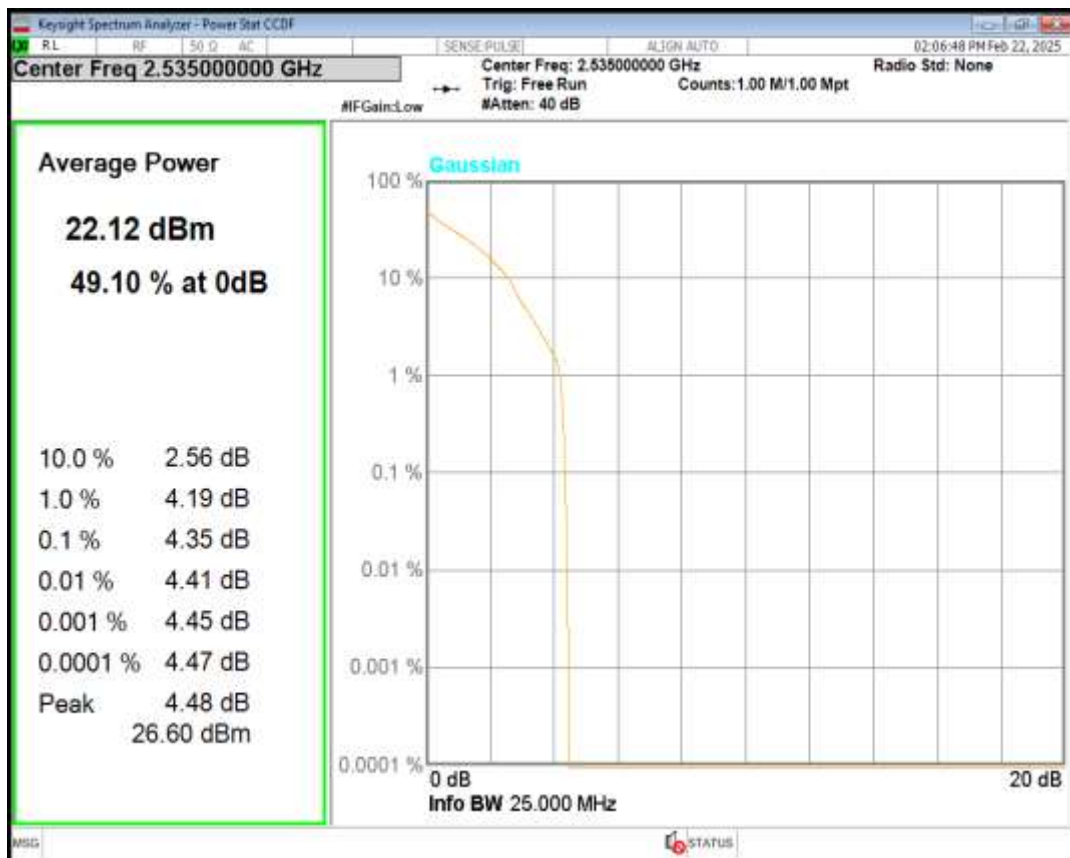
Band7 16QAM BW=5MHz Channel=21100 RB Size=1 Position=#0
