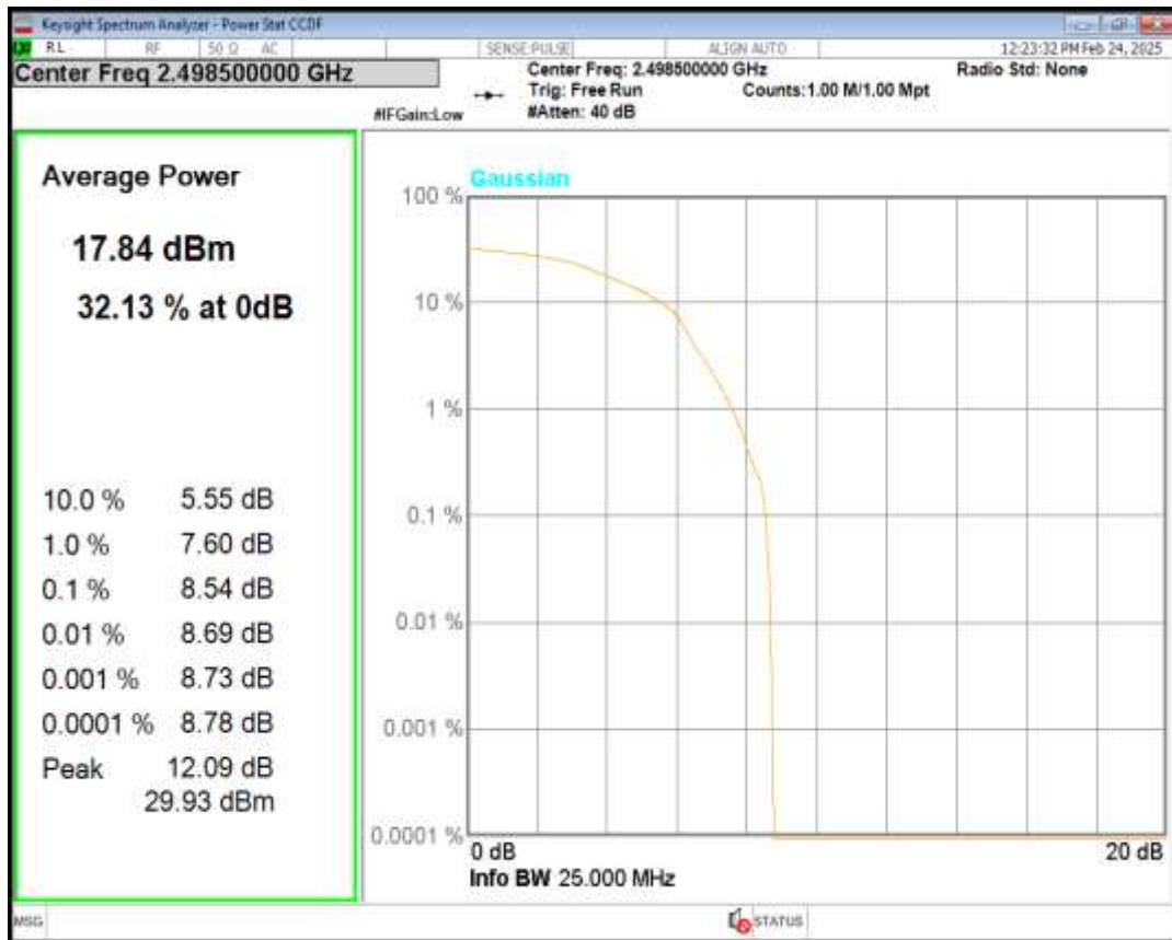
Band41 QPSK BW=5MHz Channel=40620 RB Size=1 Position=#0
