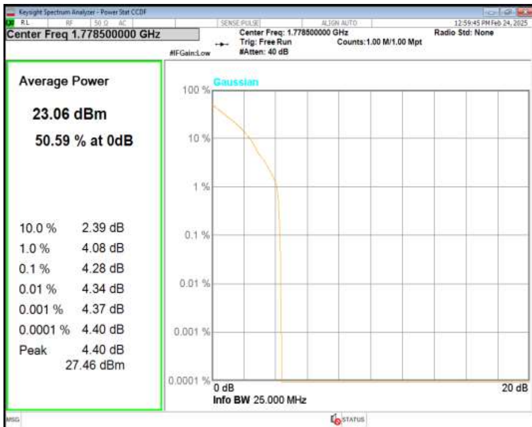
Band66 16QAM BW=3MHz Channel=132657 RB Size=1 Position=#0
