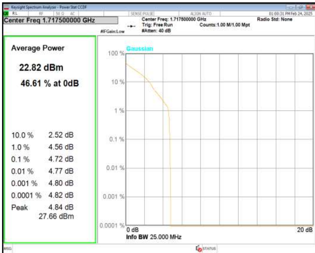
Band66 16QAM BW=15MHz Channel=132047 RB Size=1 Position=#0
