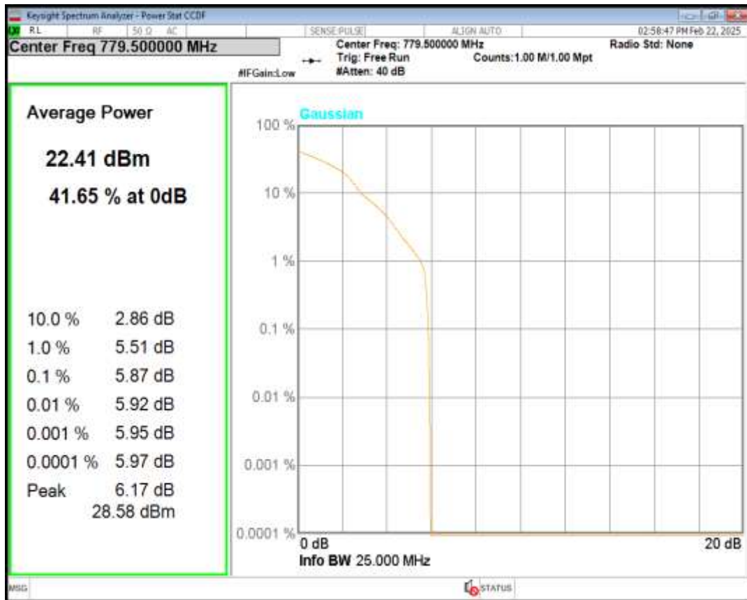
Band13 QPSK BW=5MHz Channel=23230 RB Size=1 Position=#0
