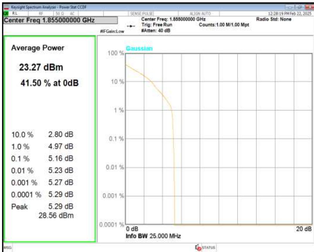
Band2 16QAM BW=10MHz Channel=18650 RB Size=1 Position=#0
