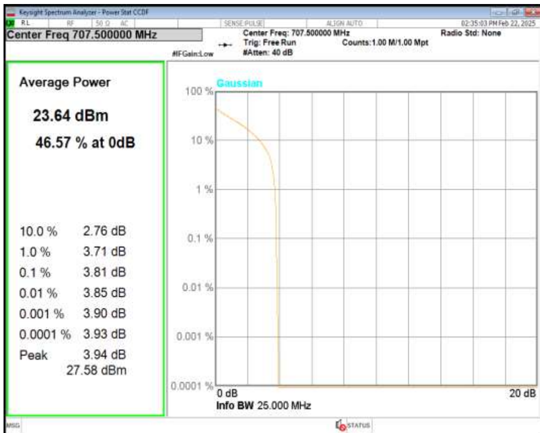
Band12 16QAM BW=5MHz Channel=23095 RB Size=1 Position=#0
