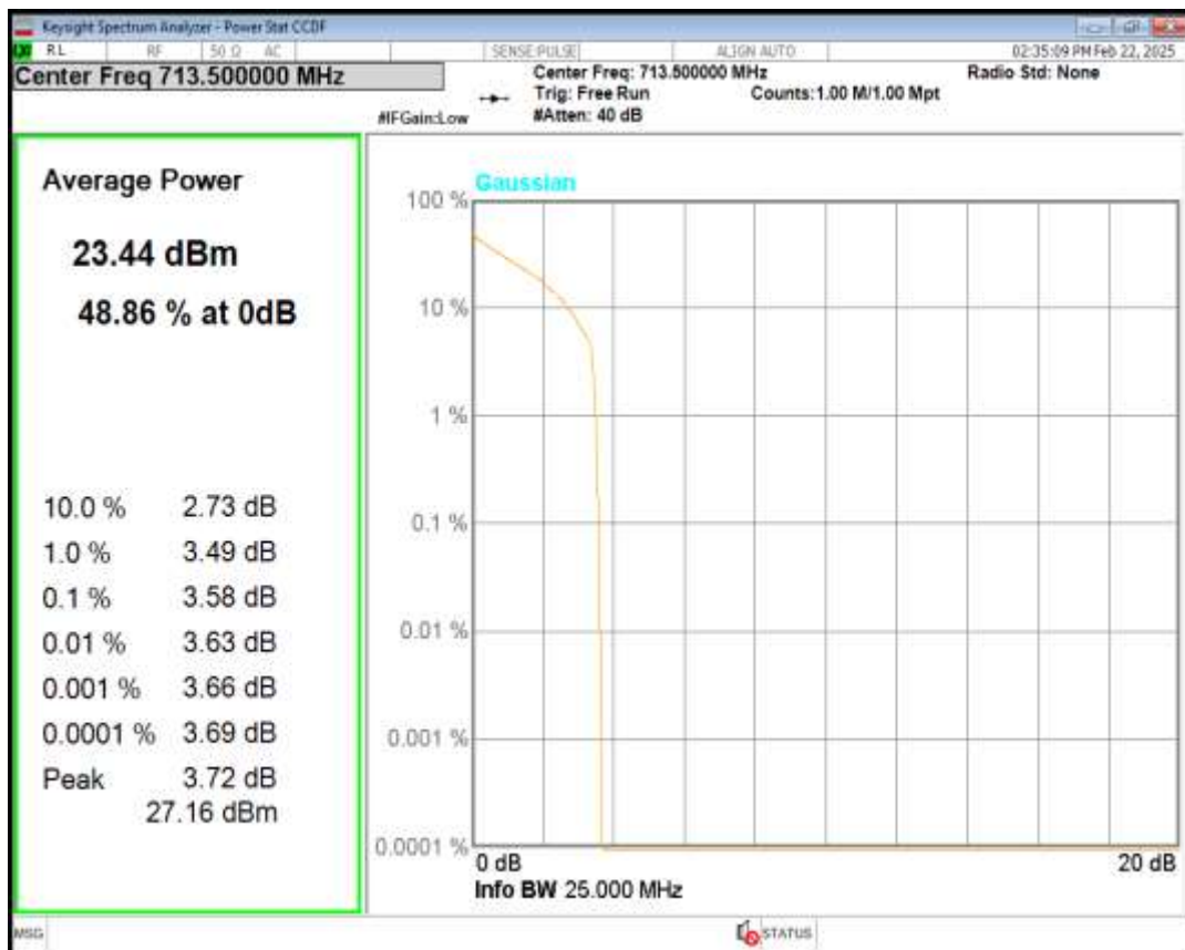
Band12 16QAM BW=5MHz Channel=23155 RB Size=1 Position=#0
