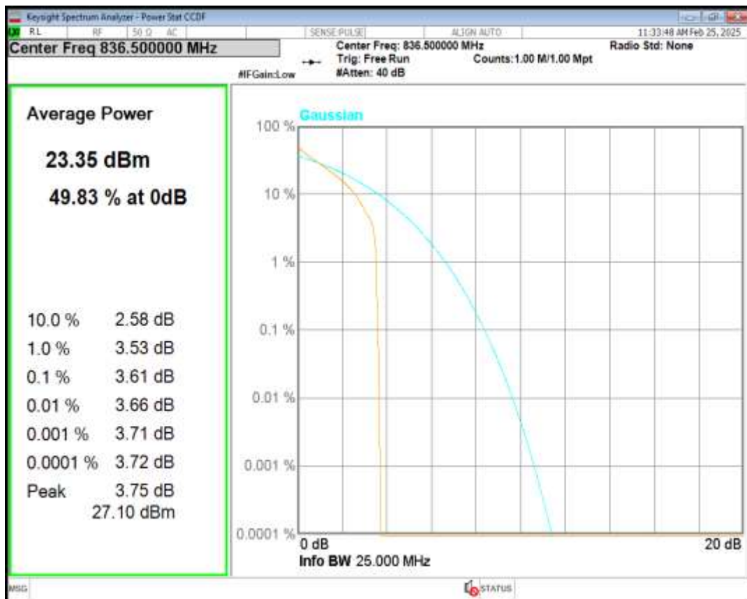
Band26(824-849) 16QAM BW=3MHz Channel=26915 RB Size=1 Position=#0
