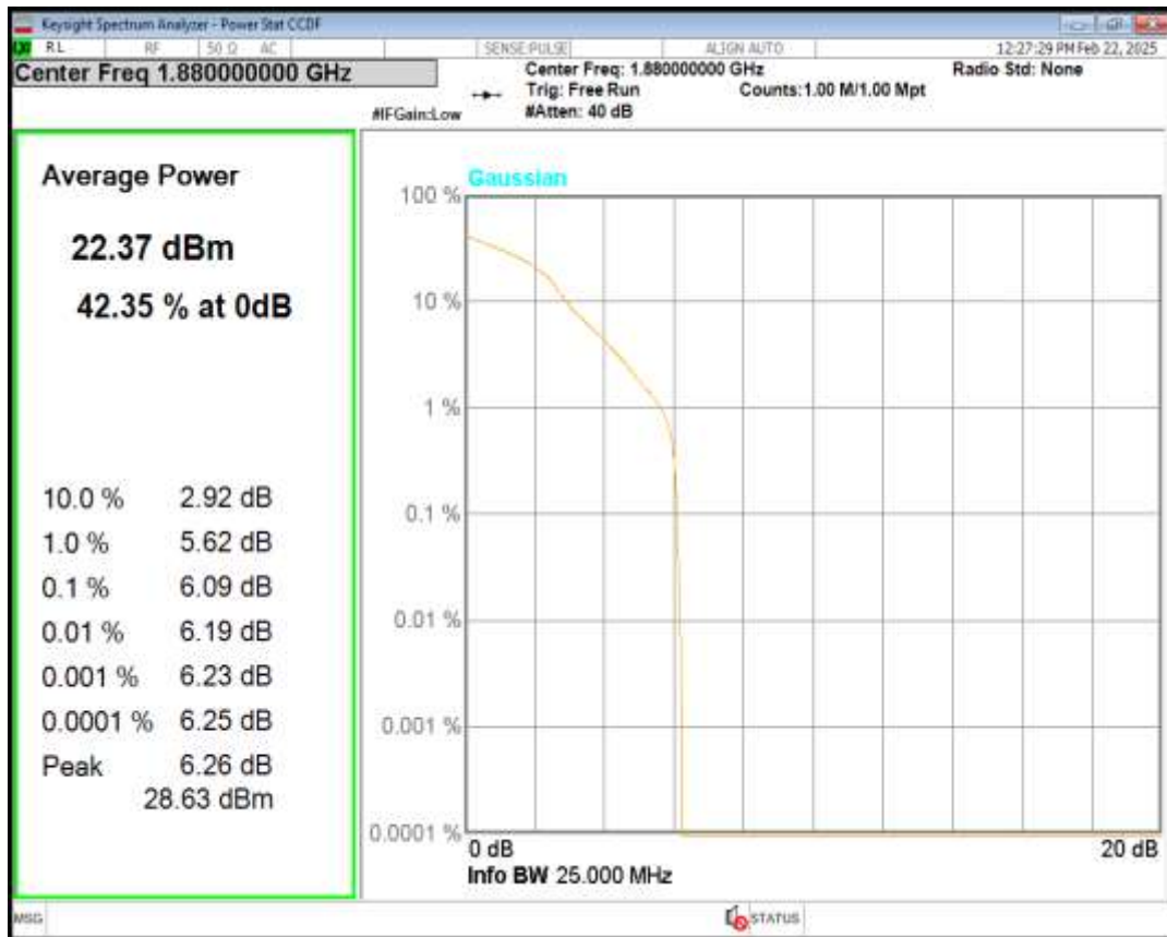
Band2 QPSK BW=1.4MHz Channel=19193 RB Size=1 Position=#0
