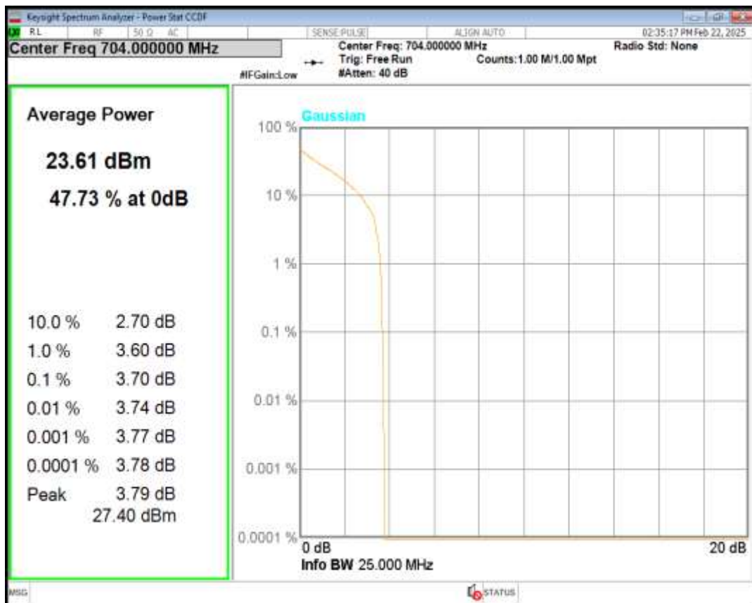
Band12 16QAM BW=10MHz Channel=23060 RB Size=1 Position=#0
