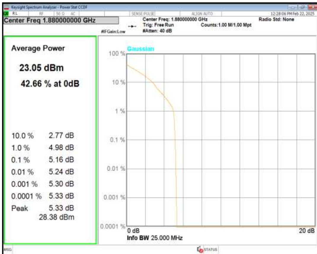
Band2 16QAM BW=5MHz Channel=18900 RB Size=1 Position=#0
