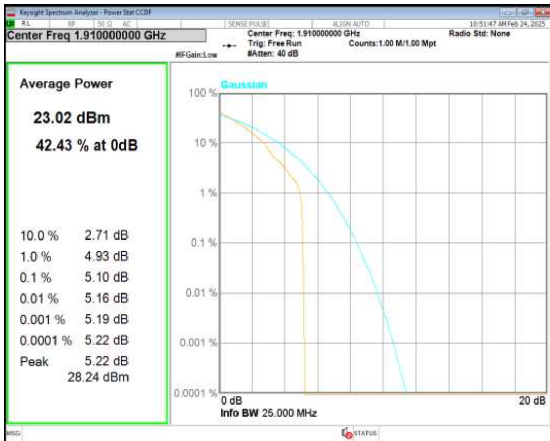
Band25 16QAM BW=10MHz Channel=26640 RB Size=1 Position=#0
