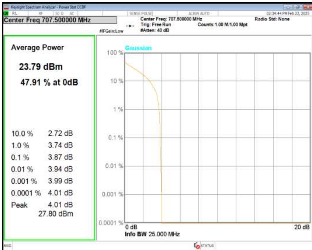
Band12 16QAM BW=3MHz Channel=23095 RB Size=1 Position=#0
