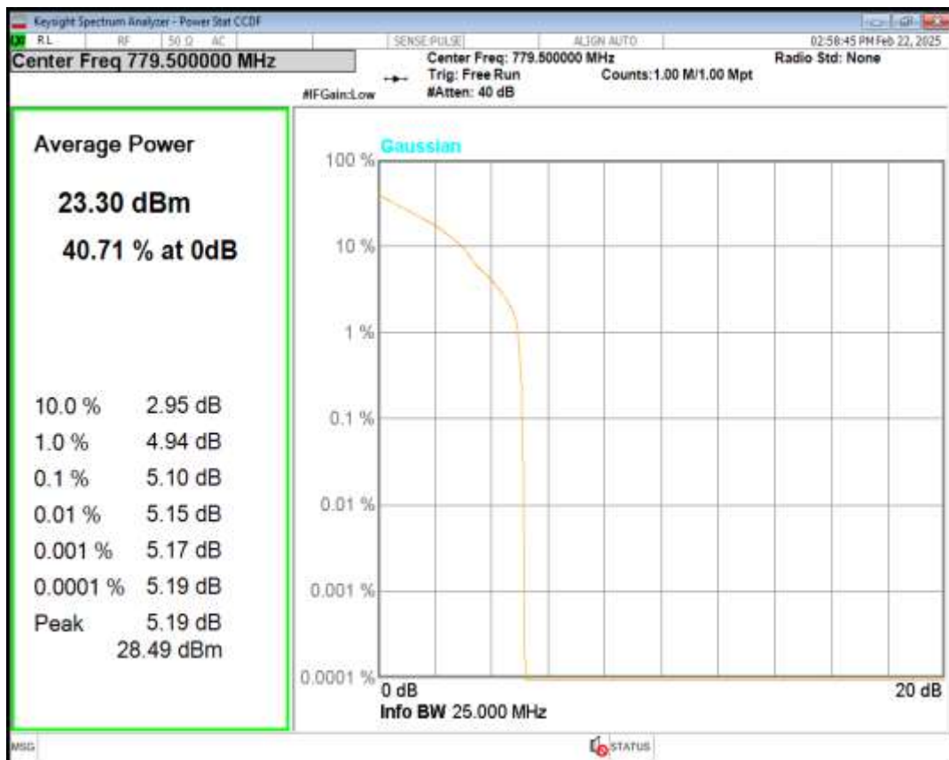
Band13 16QAM BW=5MHz Channel=23205 RB Size=1 Position=#0
