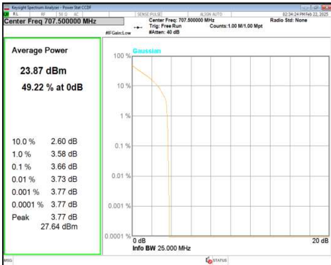
Band12 16QAM BW=1.4MHz Channel=23095 RB Size=1 Position=#0
