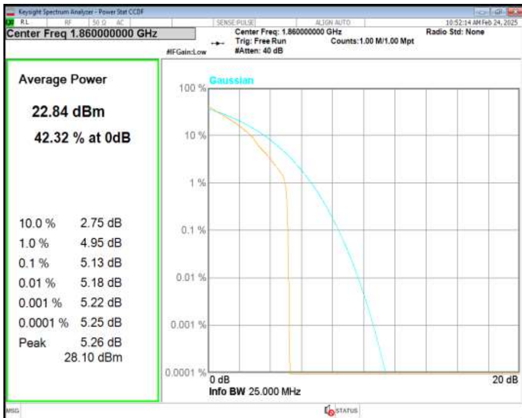
Band25 16QAM BW=20MHz Channel=26140 RB Size=1 Position=#0
