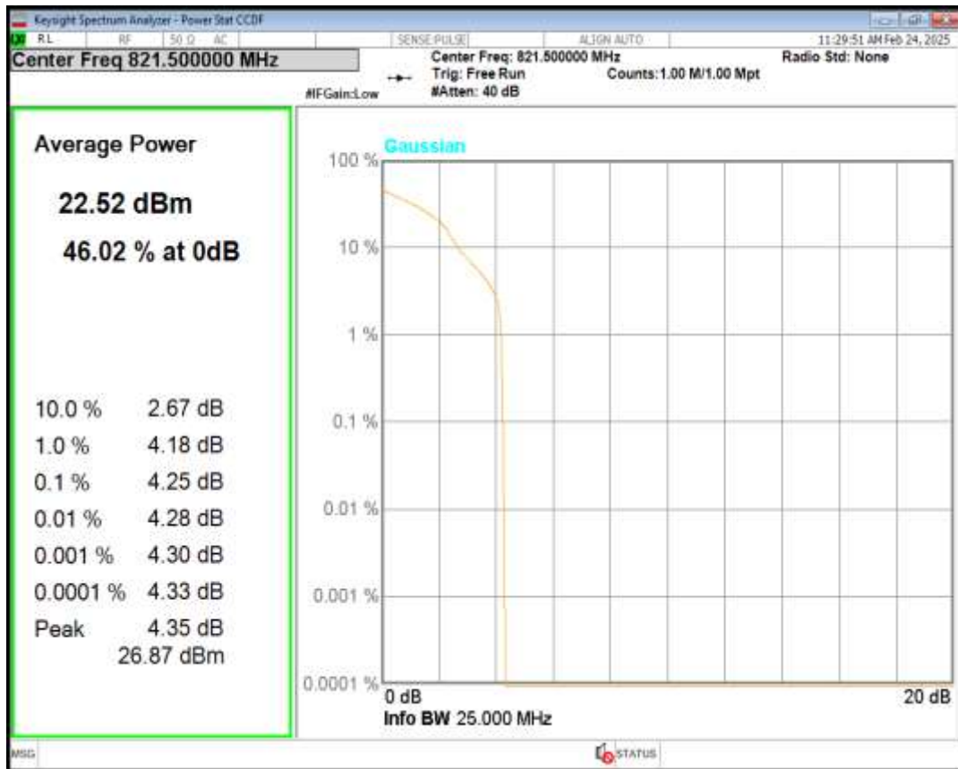
Band26(814-824) QPSK BW=10MHz Channel=26740 RB Size=1 Position=#0
