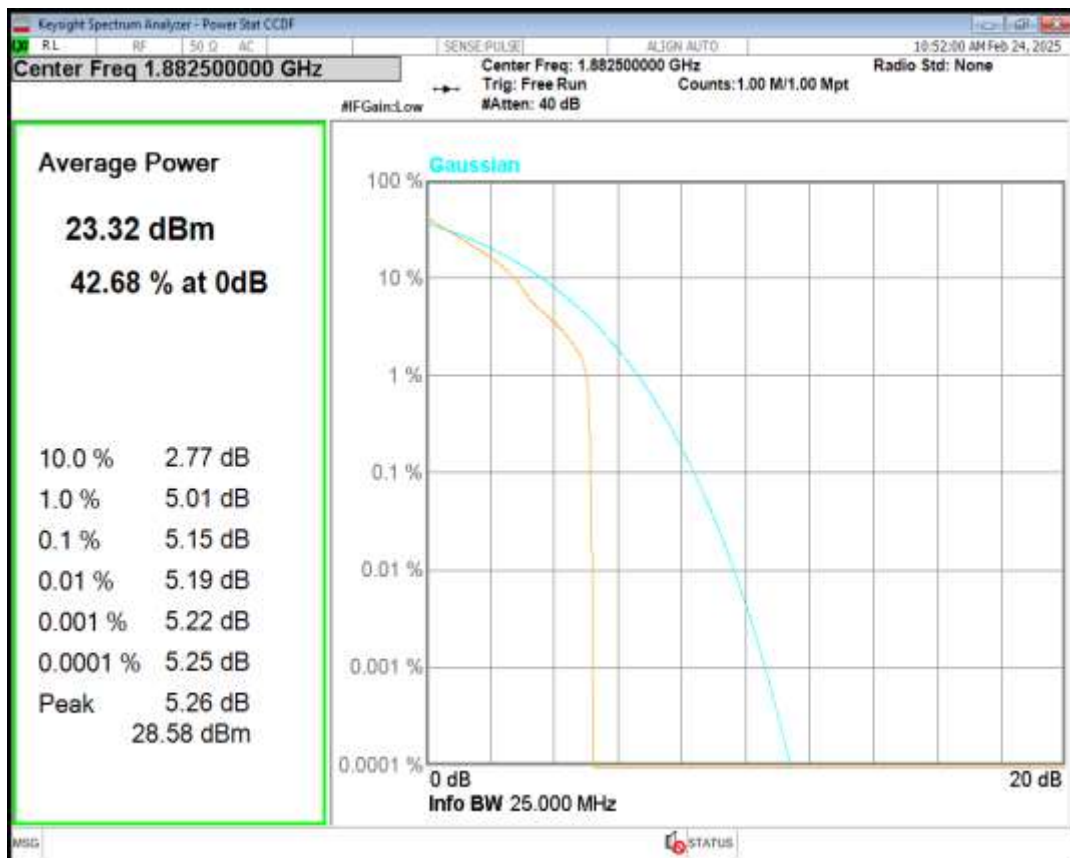
Band25 16QAM BW=15MHz Channel=26365 RB Size=1 Position=#0
