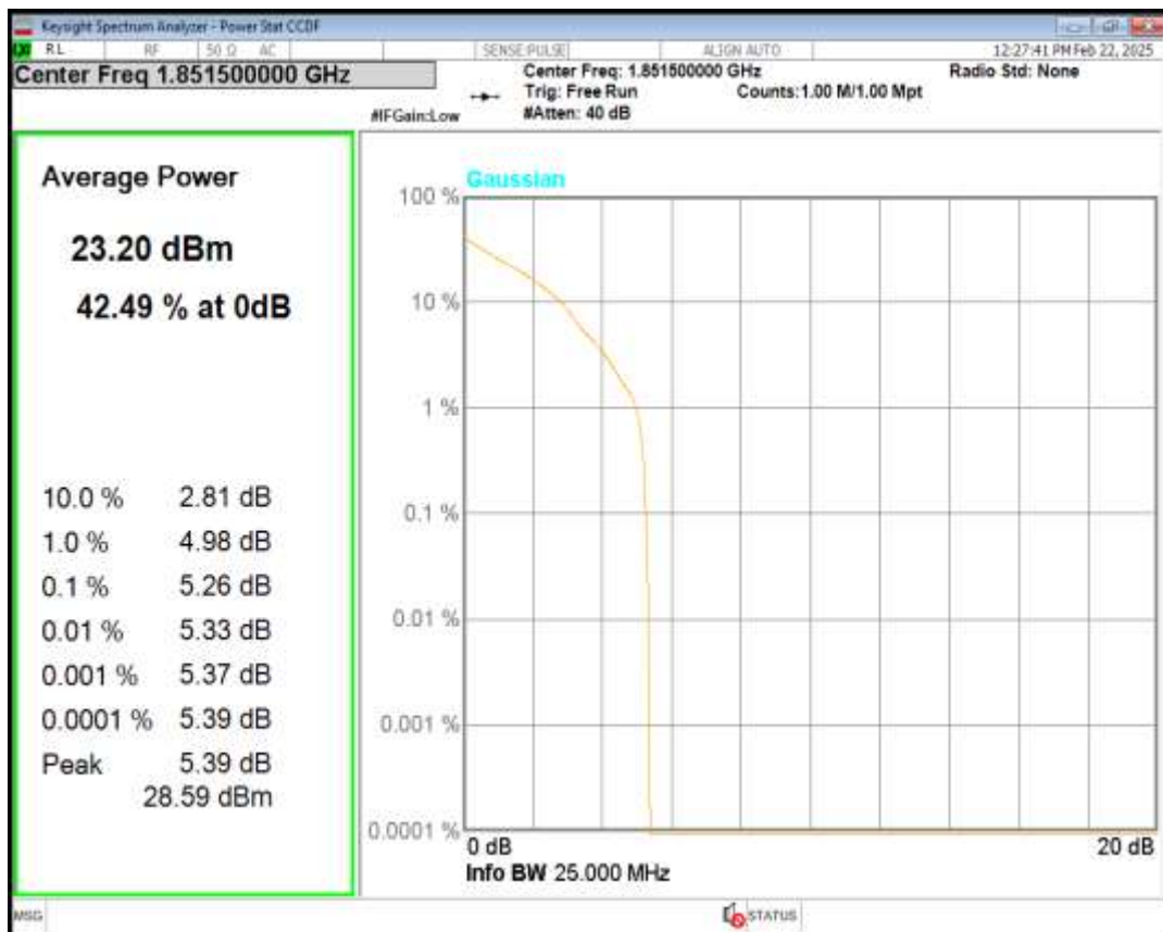
Band2 16QAM BW=3MHz Channel=18615 RB Size=1 Position=#0
