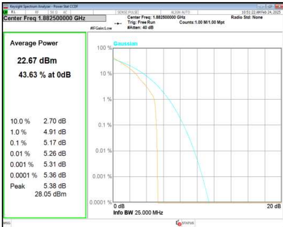
Band25 16QAM BW=5MHz Channel=26365 RB Size=1 Position=#0
