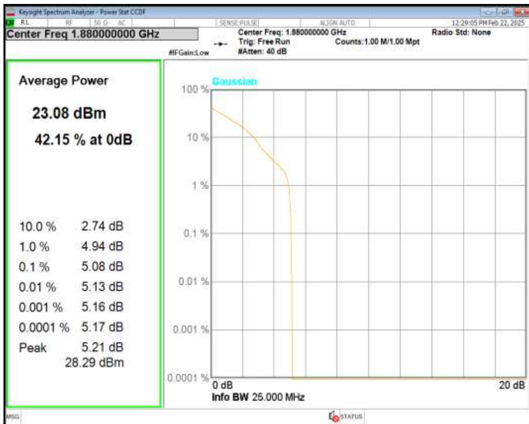
Band2 16QAM BW=20MHz Channel=18900 RB Size=1 Position=#0
