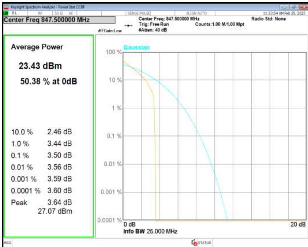
Band26(824-849) 16QAM BW=3MHz Channel=27025 RB Size=1 Position=#0
