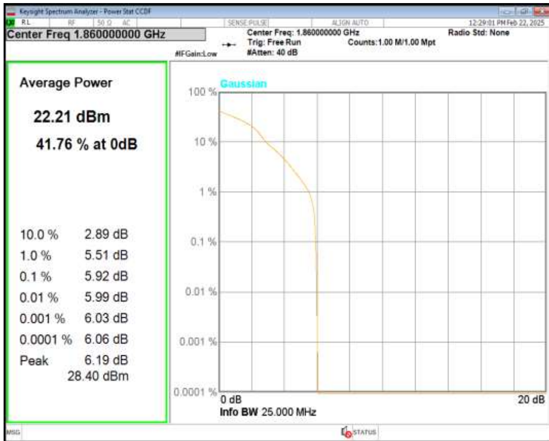
Band2 QPSK BW=20MHz Channel=18900 RB Size=1 Position=#0
