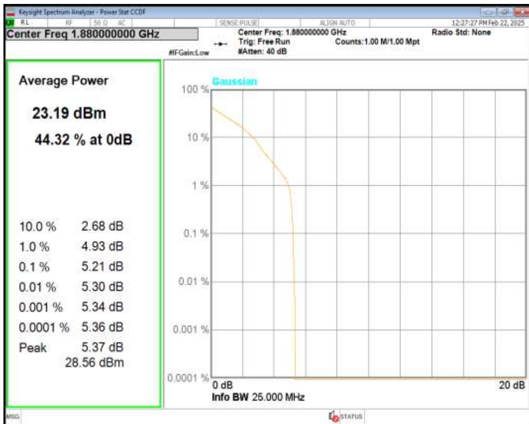
Band2 16QAM BW=1.4MHz Channel=18900 RB Size=1 Position=#0
