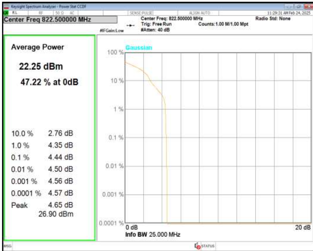
Band26(814-824) QPSK BW=5MHz Channel=26715 RB Size=1 Position=#0
