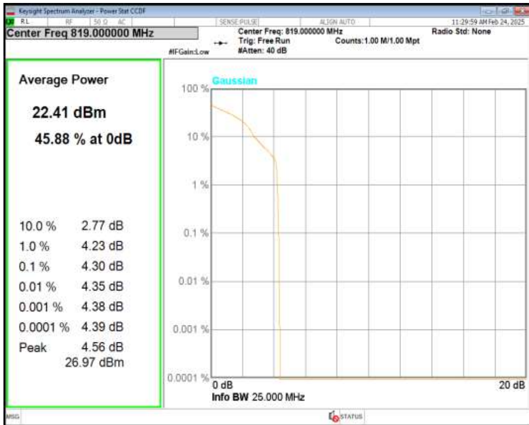
Band26(824-849) QPSK BW=1.4MHz Channel=26797 RB Size=1 Position=#0
