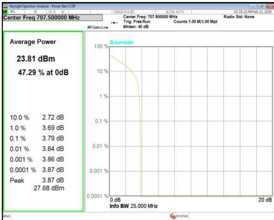
Band12 16QAM BW=10MHz Channel=23095 RB Size=1 Position=#0
