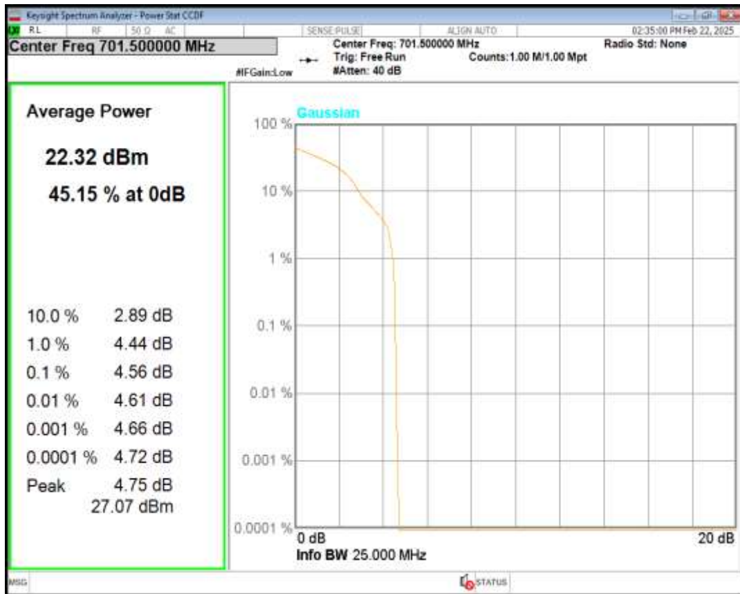
Band12 QPSK BW=5MHz Channel=23095 RB Size=1 Position=#0
