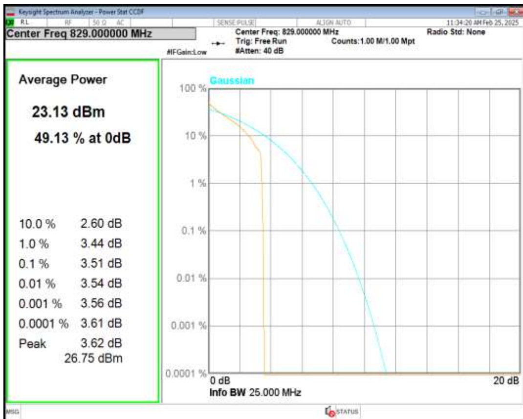
Band26(824-849) 16QAM BW=10MHz Channel=26840 RB Size=1 Position=#0
