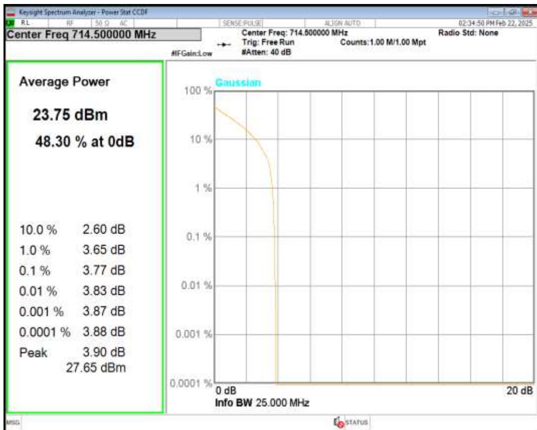
Band12 16QAM BW=3MHz Channel=23165 RB Size=1 Position=#0
