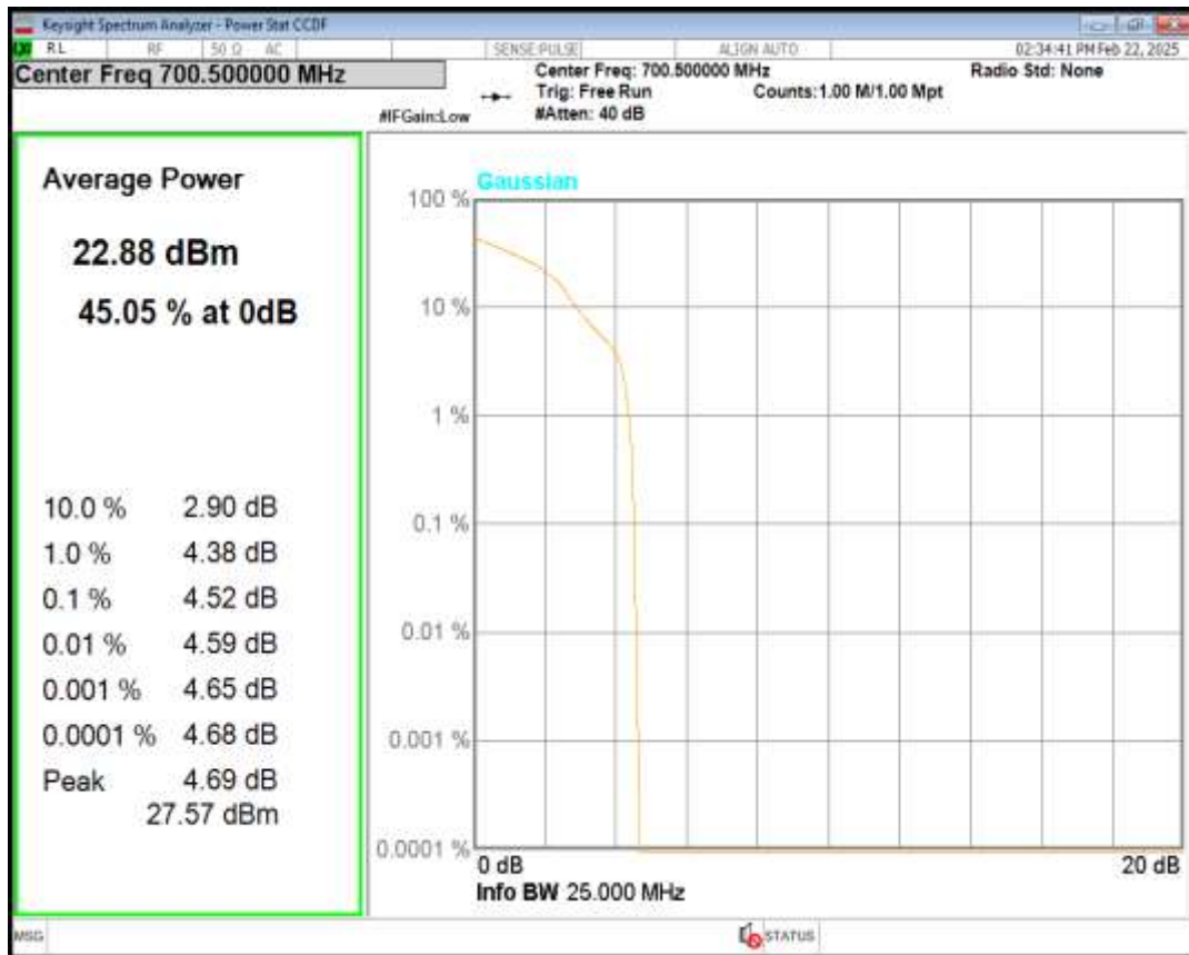
Band12 QPSK BW=3MHz Channel=23095 RB Size=1 Position=#0
