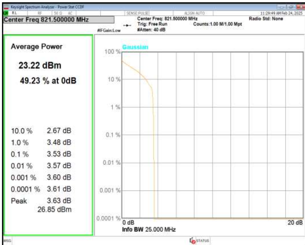
Band26(814-824) 16QAM BW=5MHz Channel=26765 RB Size=1 Position=#0
