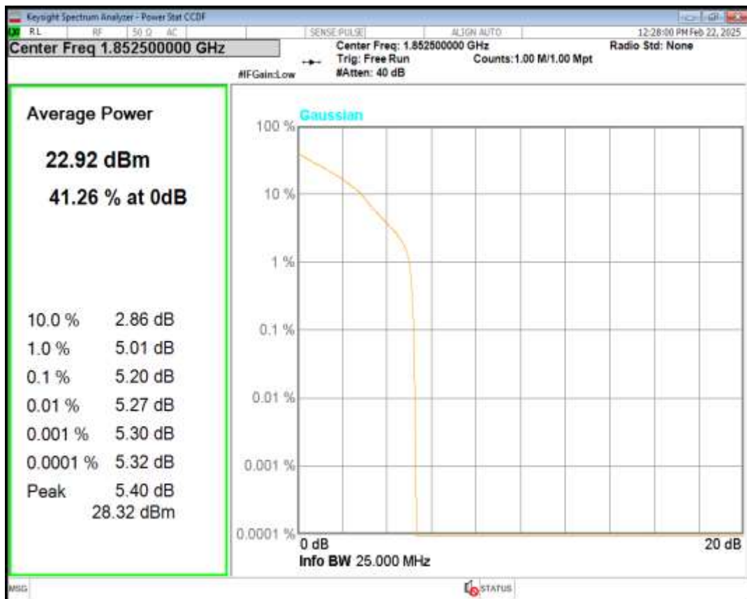
Band2 16QAM BW=5MHz Channel=18625 RB Size=1 Position=#0
