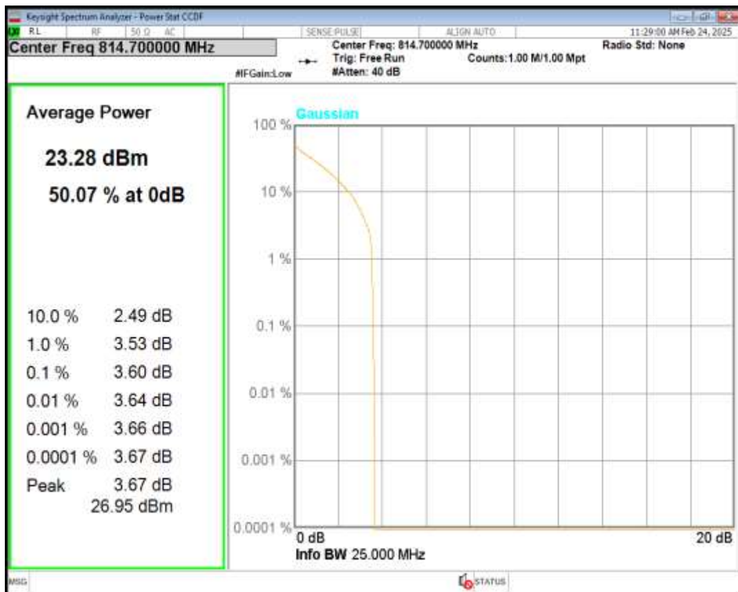
Band26(814-824) 16QAM BW=1.4MHz Channel=26697 RB Size=1 Position=#0
