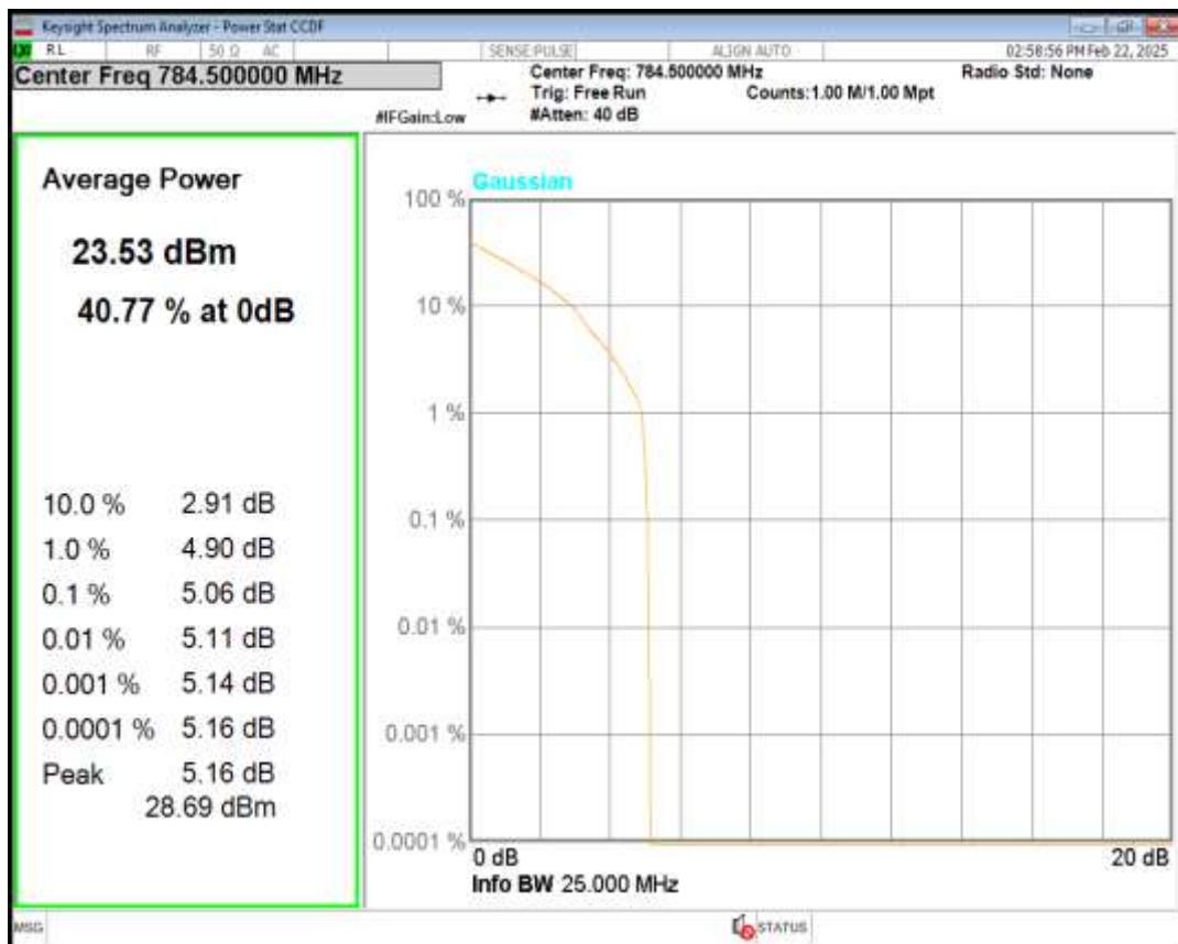
Band13 16QAM BW=5MHz Channel=23255 RB Size=1 Position=#0
