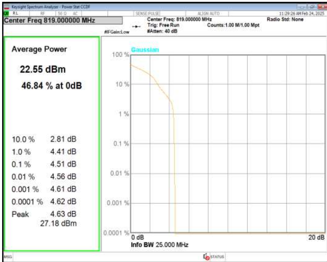
Band26(814-824) QPSK BW=3MHz Channel=26775 RB Size=1 Position=#0
