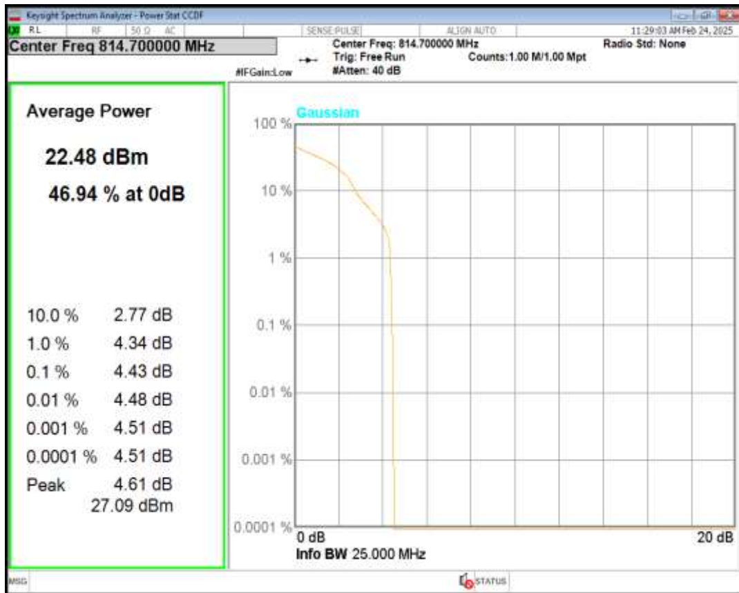
Band26(814-824) QPSK BW=1.4MHz Channel=26740 RB Size=1 Position=#0
