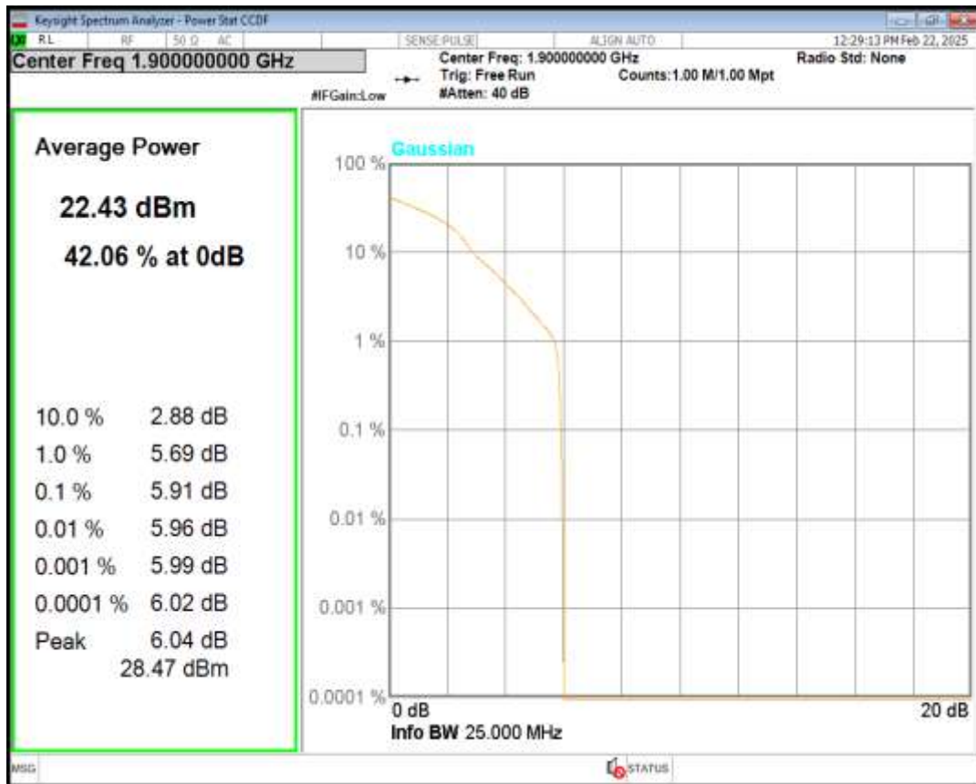
Band25 QPSK BW=1.4MHz Channel=26047 RB Size=1 Position=#0
