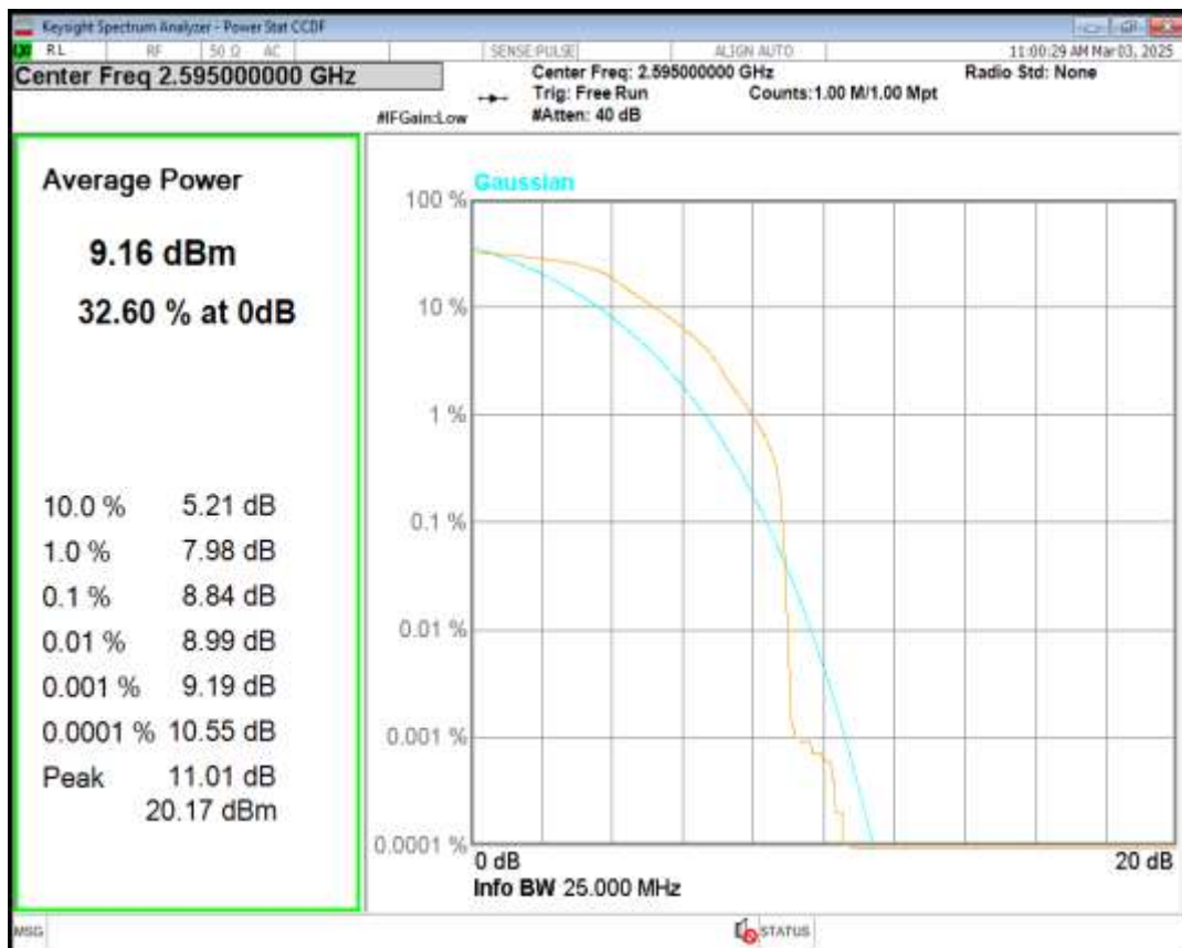
Band38 16QAM BW=5MHz Channel=38000 RB Size=1 Position=#0
