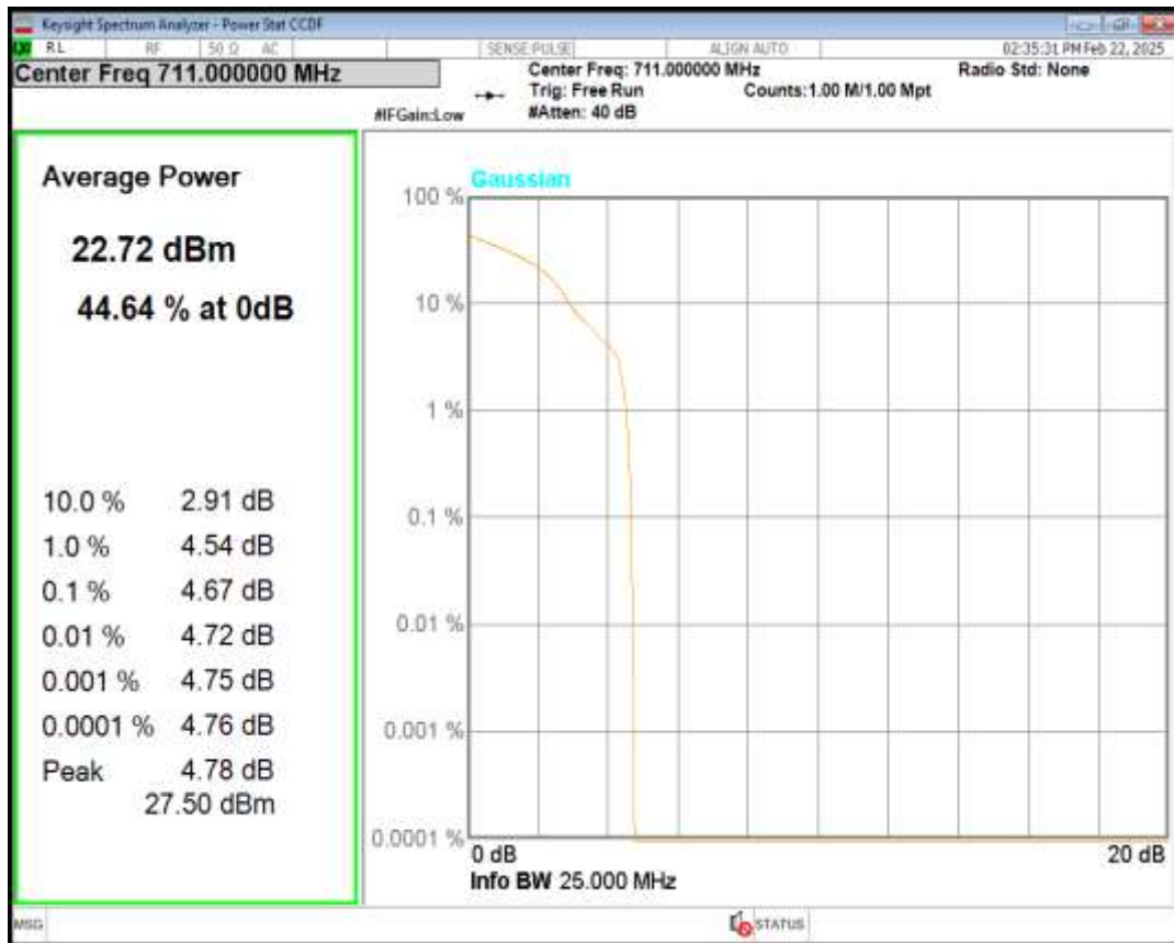
Band13 QPSK BW=5MHz Channel=23205 RB Size=1 Position=#0
