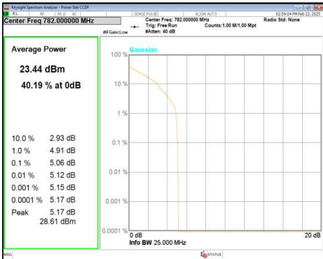
Band13 16QAM BW=10MHz Channel=23230 RB Size=1 Position=#0
