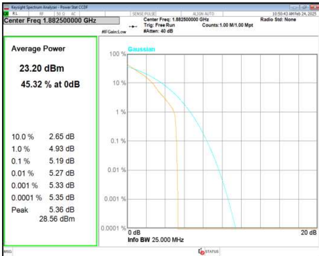
Band25 16QAM BW=1.4MHz Channel=26365 RB Size=1 Position=#0
