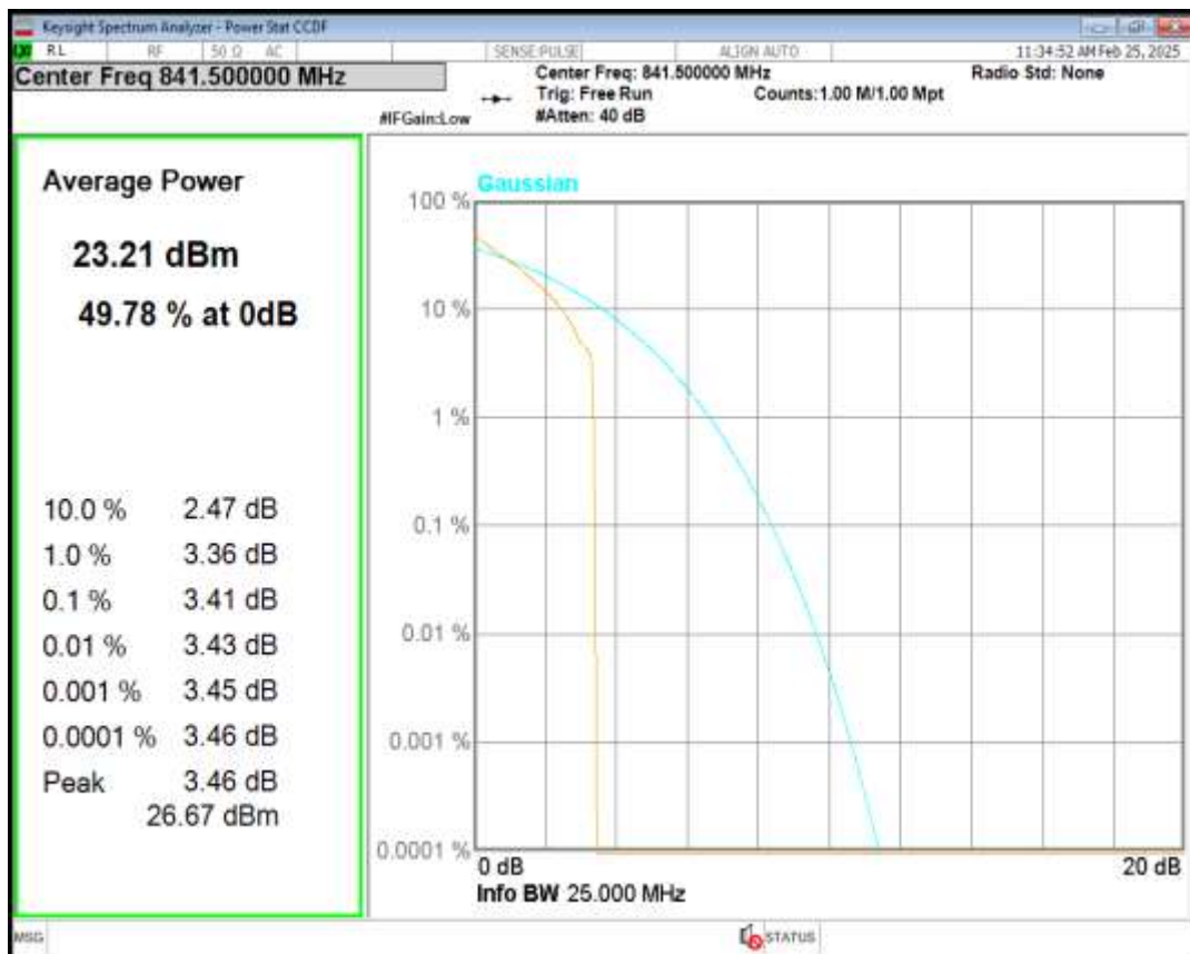
Band26(824-849) 16QAM BW=15MHz Channel=26965 RB Size=1 Position=#0
