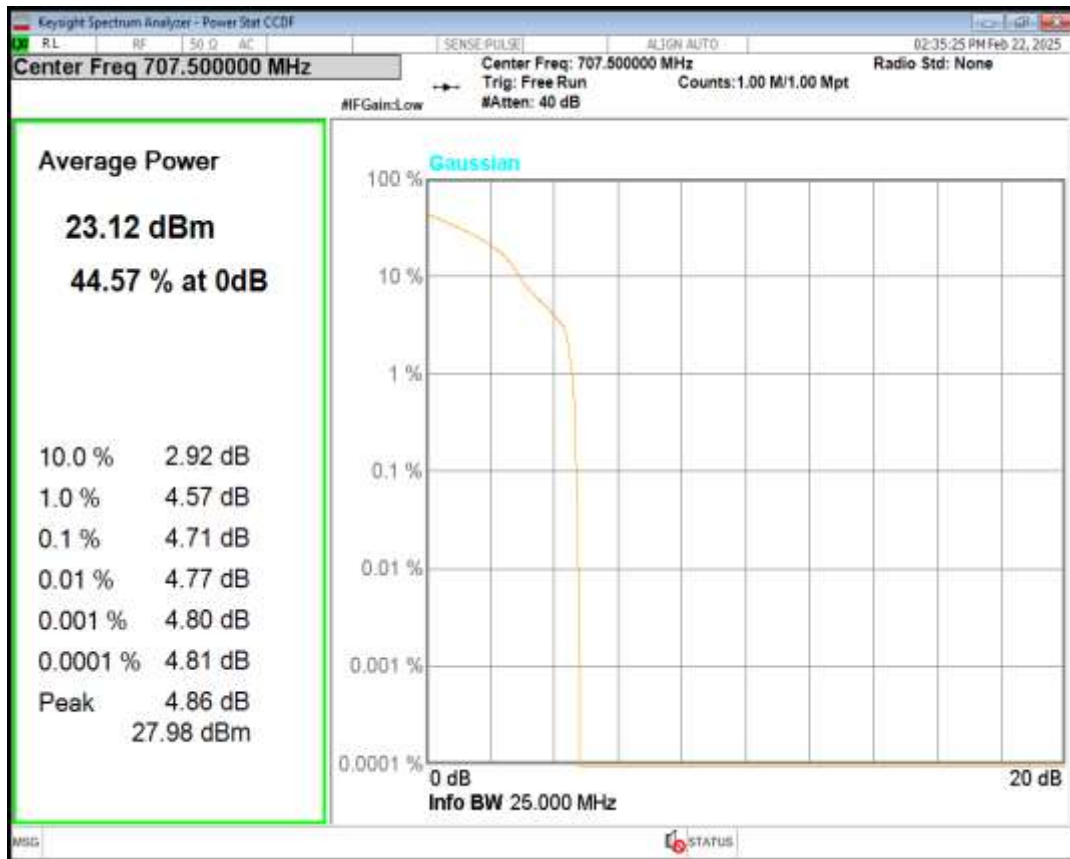
Band12 QPSK BW=10MHz Channel=23130 RB Size=1 Position=#0
