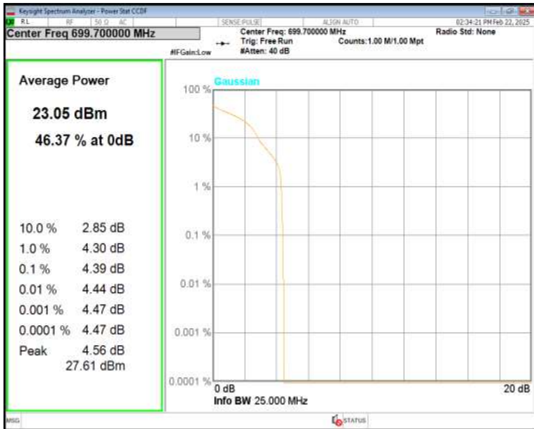
Band12 QPSK BW=1.4MHz Channel=23095 RB Size=1 Position=#0
