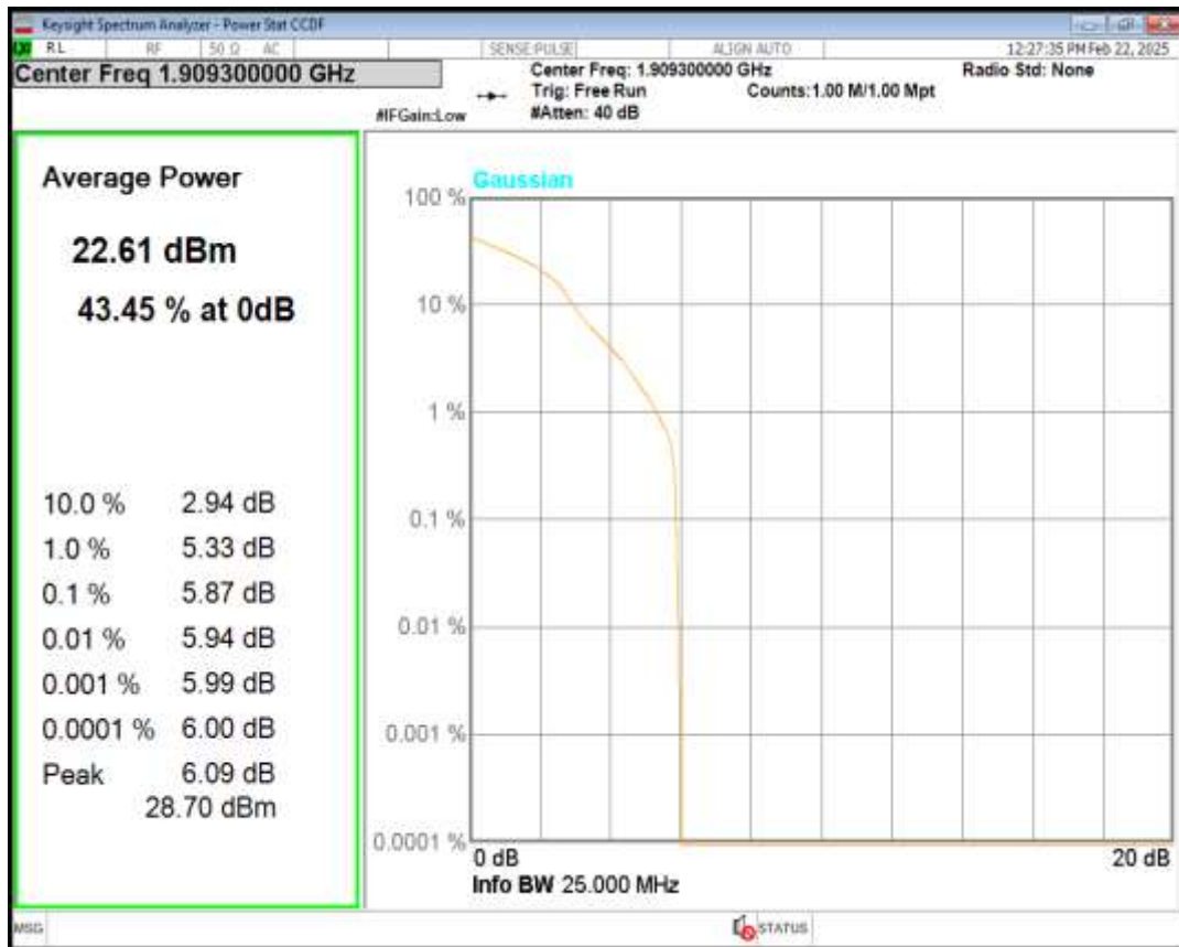
Band2 QPSK BW=3MHz Channel=18615 RB Size=1 Position=#0
