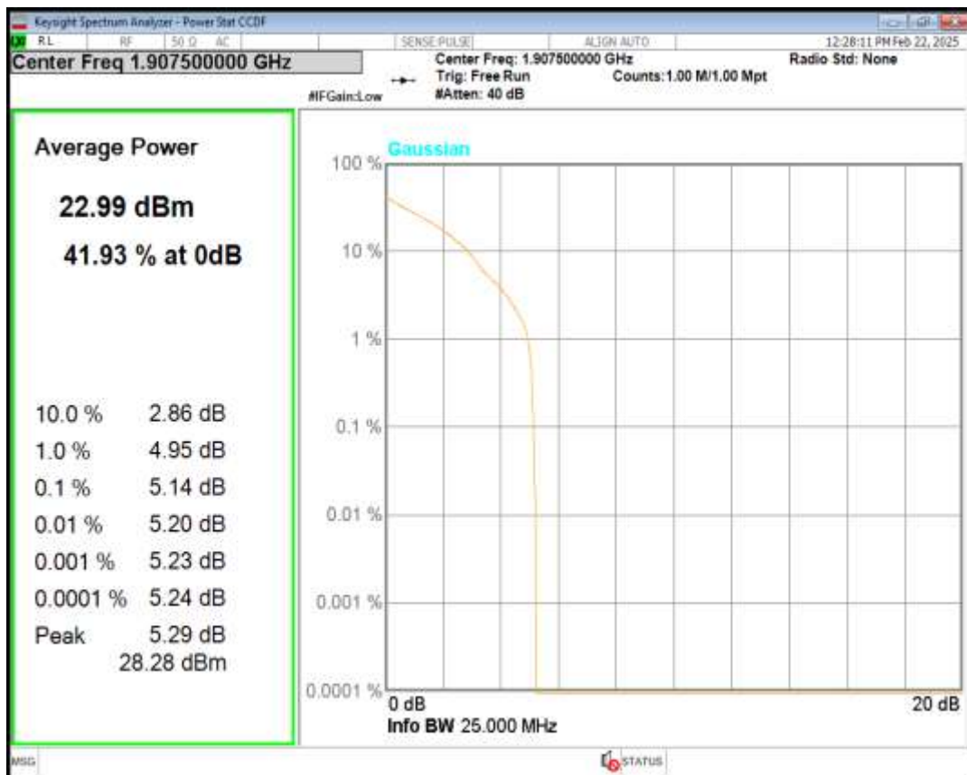
Band2 16QAM BW=5MHz Channel=19175 RB Size=1 Position=#0
