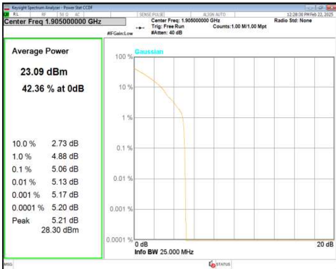
Band2 16QAM BW=10MHz Channel=19150 RB Size=1 Position=#0
