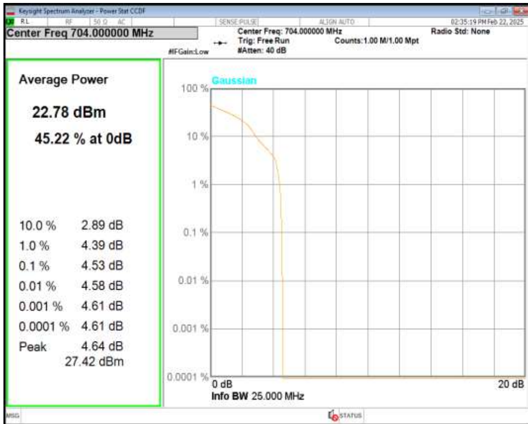
Band12 QPSK BW=10MHz Channel=23095 RB Size=1 Position=#0
