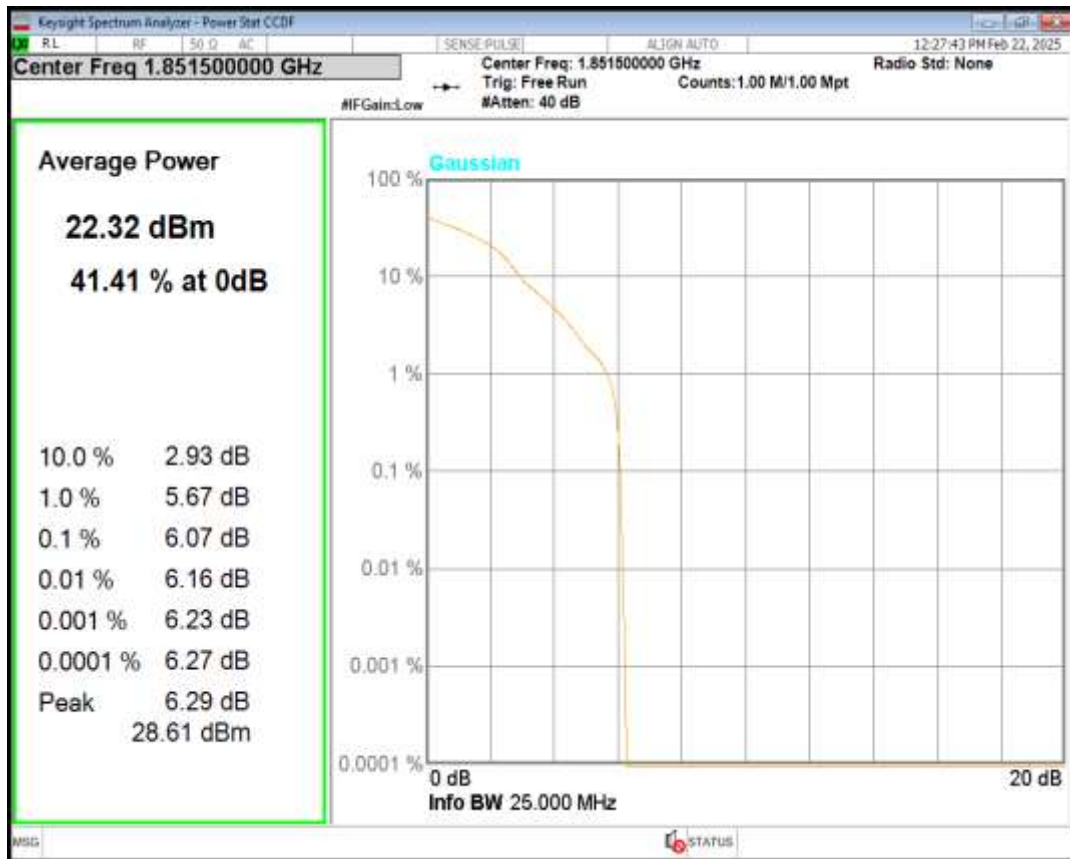
Band2 QPSK BW=3MHz Channel=18900 RB Size=1 Position=#0
