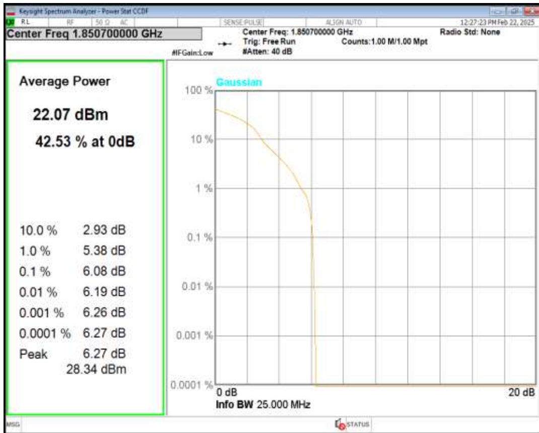
Band2 QPSK BW=1.4MHz Channel=18900 RB Size=1 Position=#0
