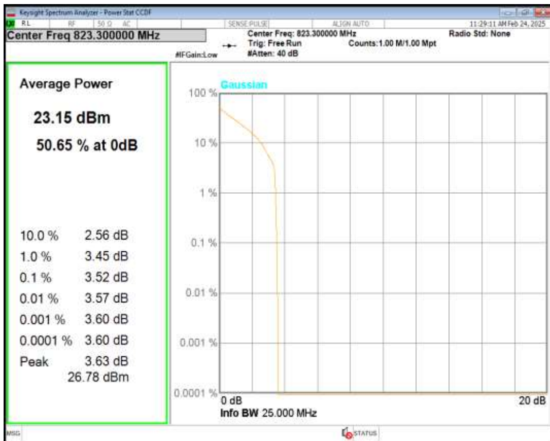
Band26(814-824) 16QAM BW=1.4MHz Channel=26783 RB Size=1 Position=#0
