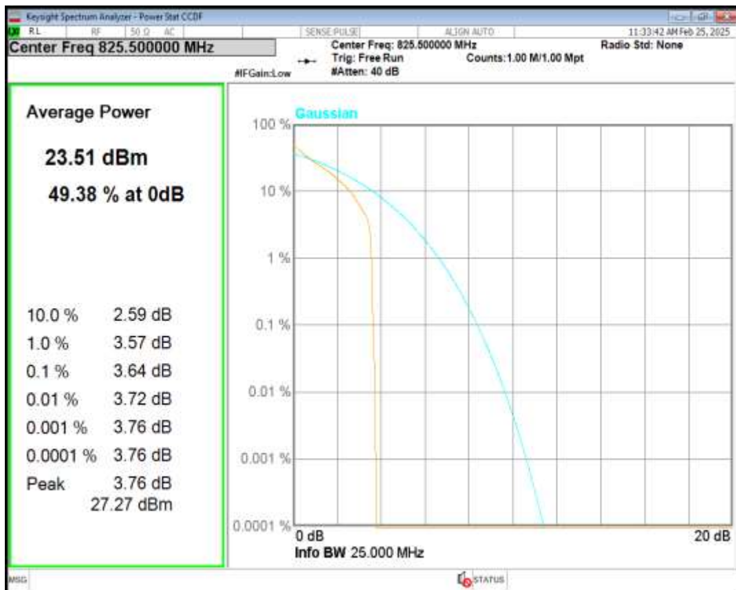
Band26(824-849) 16QAM BW=3MHz Channel=26805 RB Size=1 Position=#0
