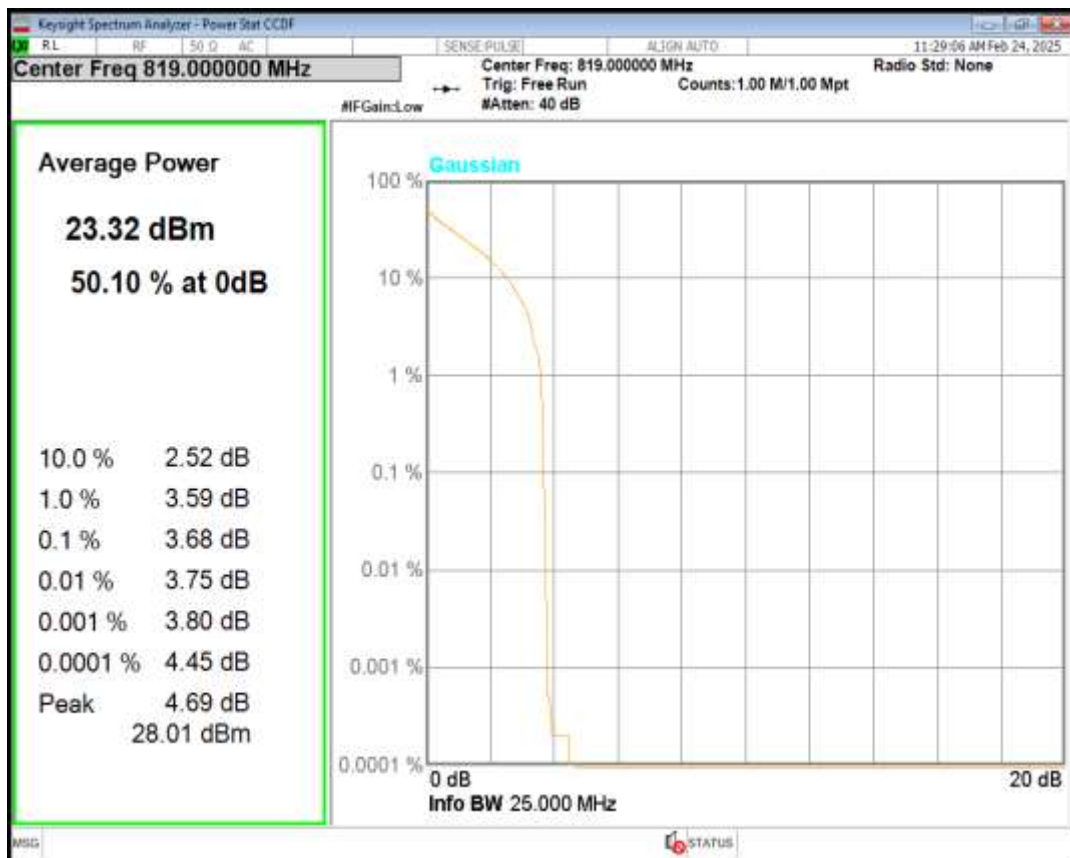
Band26(814-824) 16QAM BW=1.4MHz Channel=26740 RB Size=1 Position=#0
