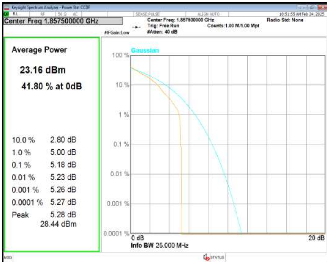
Band25 16QAM BW=15MHz Channel=26115 RB Size=1 Position=#0
