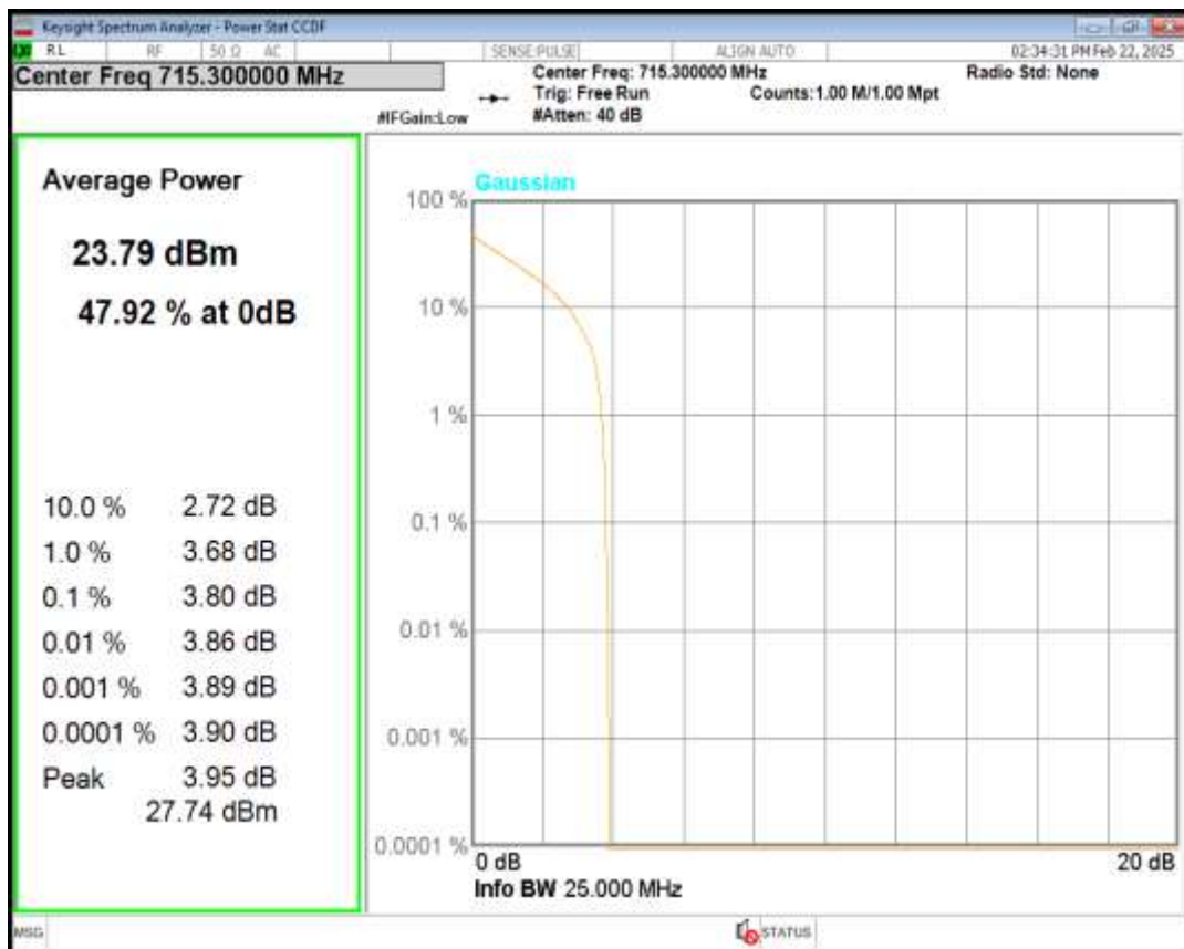
Band12 16QAM BW=1.4MHz Channel=23173 RB Size=1 Position=#0
