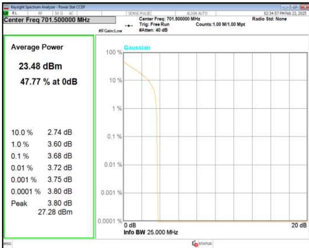
Band12 16QAM BW=5MHz Channel=23035 RB Size=1 Position=#0
