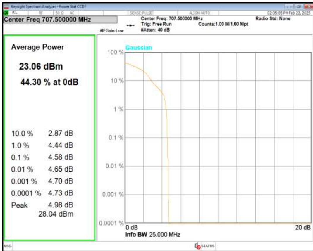
Band12 QPSK BW=5MHz Channel=23155 RB Size=1 Position=#0
