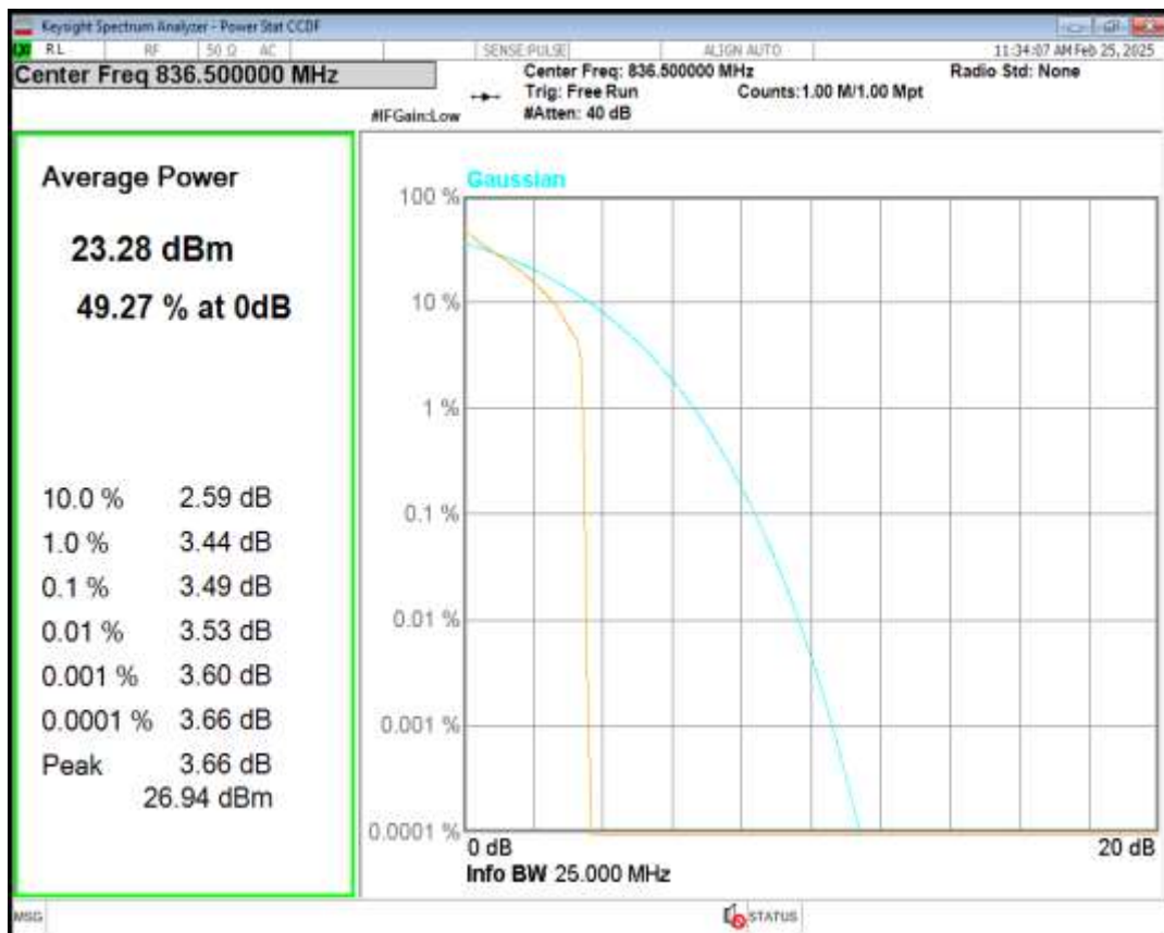
Band26(824-849) 16QAM BW=5MHz Channel=26915 RB Size=1 Position=#0
