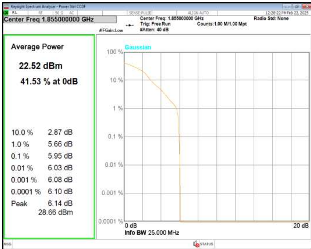
Band2 QPSK BW=10MHz Channel=18900 RB Size=1 Position=#0
