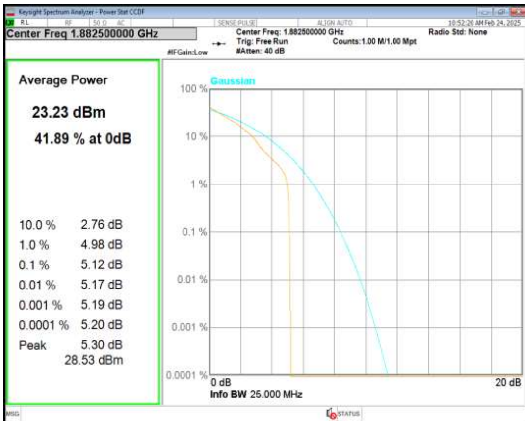
Band25 16QAM BW=20MHz Channel=26365 RB Size=1 Position=#0
