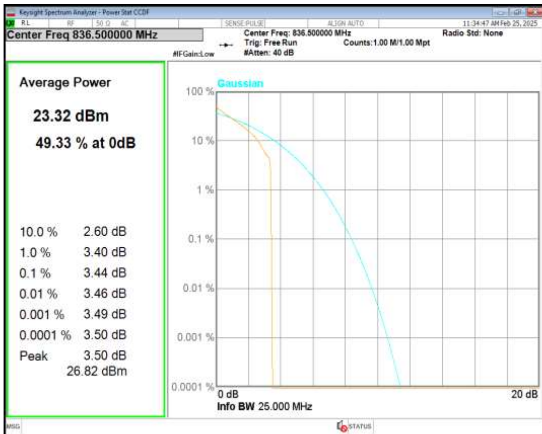
Band26(824-849) 16QAM BW=15MHz Channel=26915 RB Size=1 Position=#0
