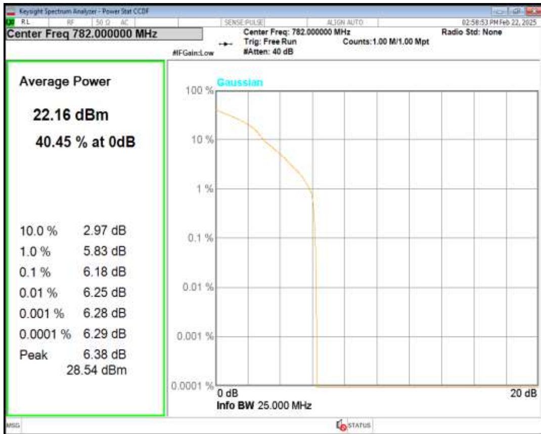
Band13 QPSK BW=5MHz Channel=23255 RB Size=1 Position=#0
