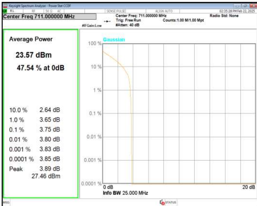
Band12 16QAM BW=10MHz Channel=23130 RB Size=1 Position=#0
