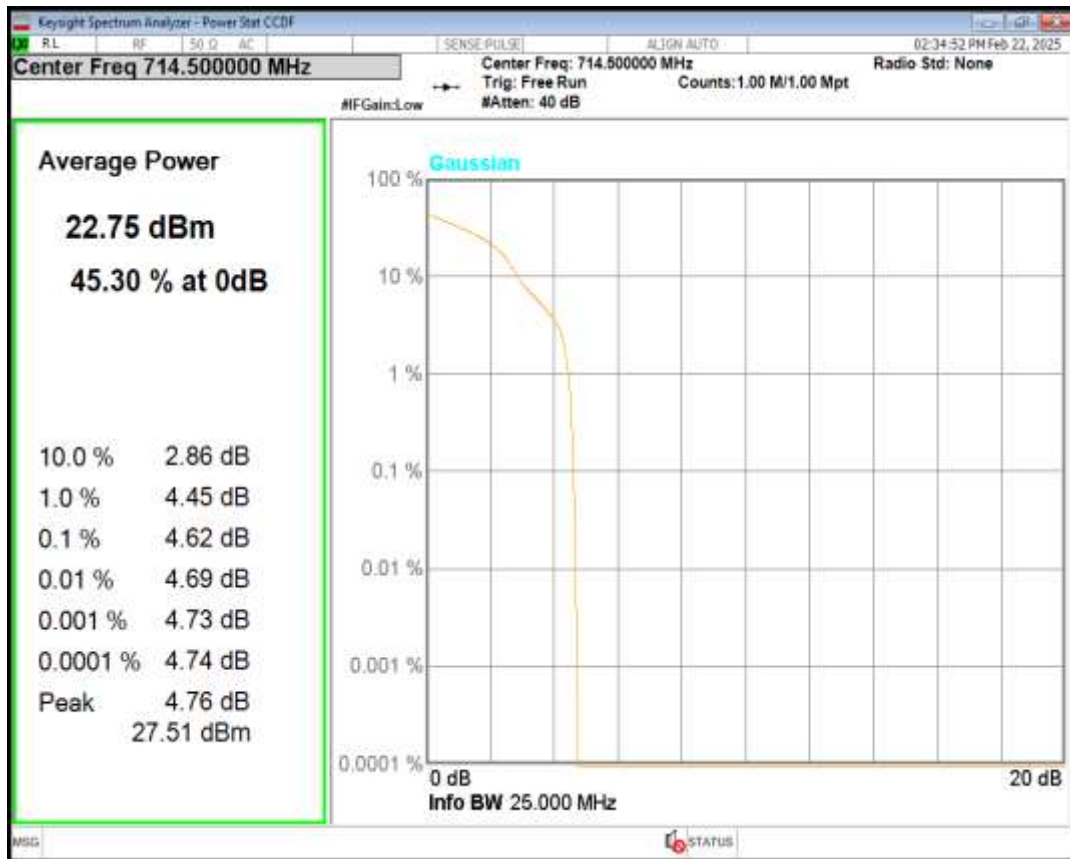
Band12 QPSK BW=5MHz Channel=23035 RB Size=1 Position=#0
