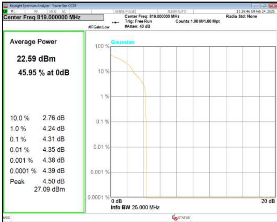
Band26(814-824) QPSK BW=5MHz Channel=26765 RB Size=1 Position=#0
