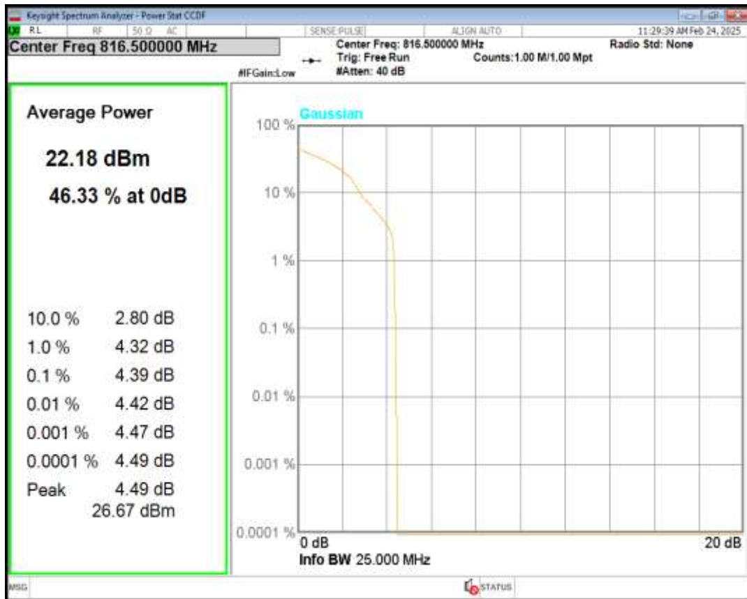
Band26(814-824) QPSK BW=5MHz Channel=26740 RB Size=1 Position=#0
