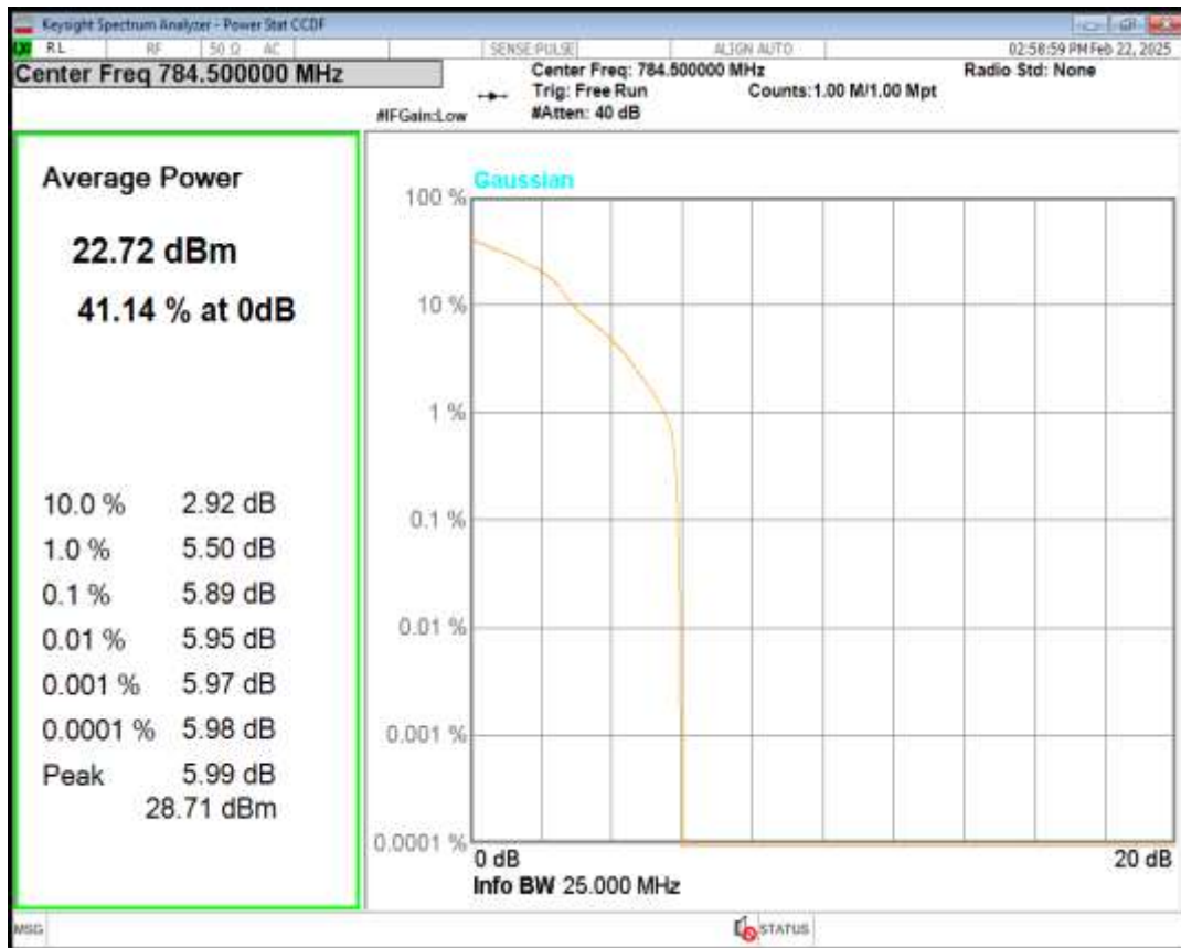
Band13 QPSK BW=10MHz Channel=23230 RB Size=1 Position=#0
