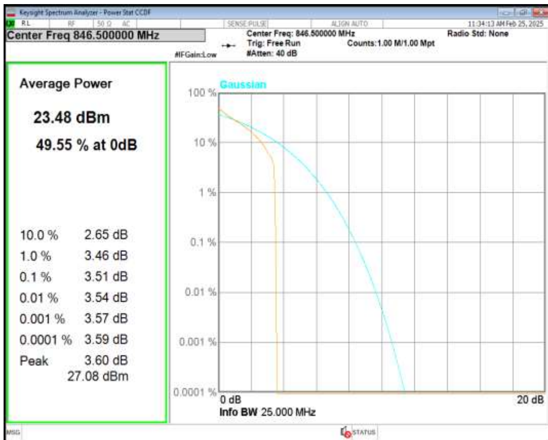
Band26(824-849) 16QAM BW=5MHz Channel=27015 RB Size=1 Position=#0
