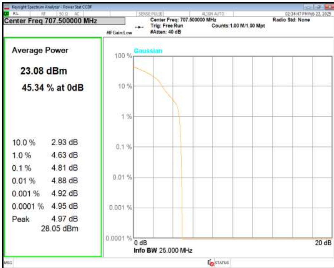
Band12 QPSK BW=3MHz Channel=23165 RB Size=1 Position=#0
