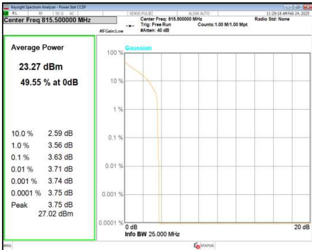
Band26(814-824) 16QAM BW=3MHz Channel=26705 RB Size=1 Position=#0
