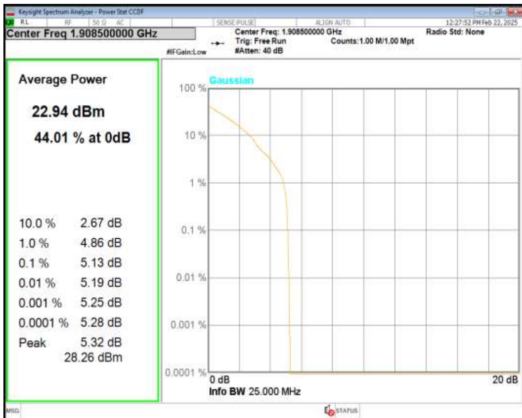
Band2 16QAM BW=3MHz Channel=19185 RB Size=1 Position=#0
