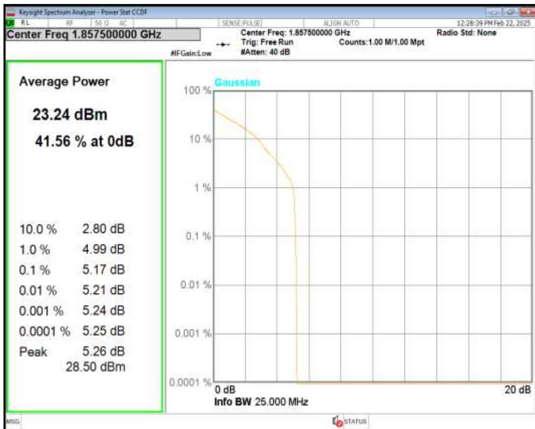
Band2 16QAM BW=15MHz Channel=18675 RB Size=1 Position=#0
