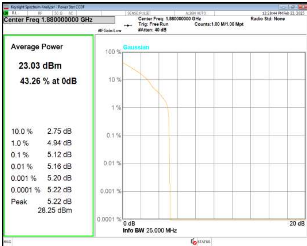
Band2 16QAM BW=15MHz Channel=18900 RB Size=1 Position=#0
