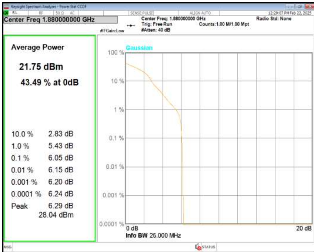
Band2 QPSK BW=20MHz Channel=19100 RB Size=1 Position=#0
