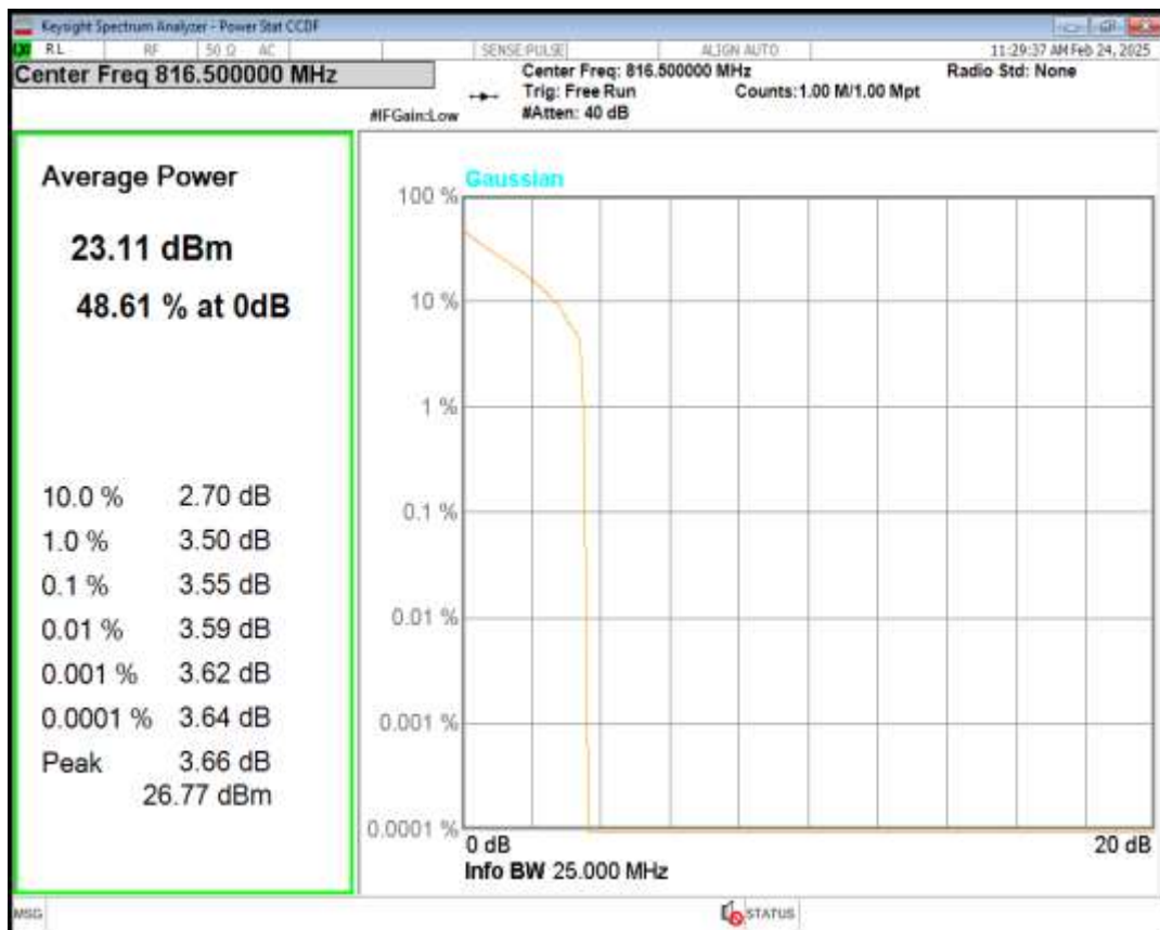
Band26(814-824) 16QAM BW=5MHz Channel=26715 RB Size=1 Position=#0
