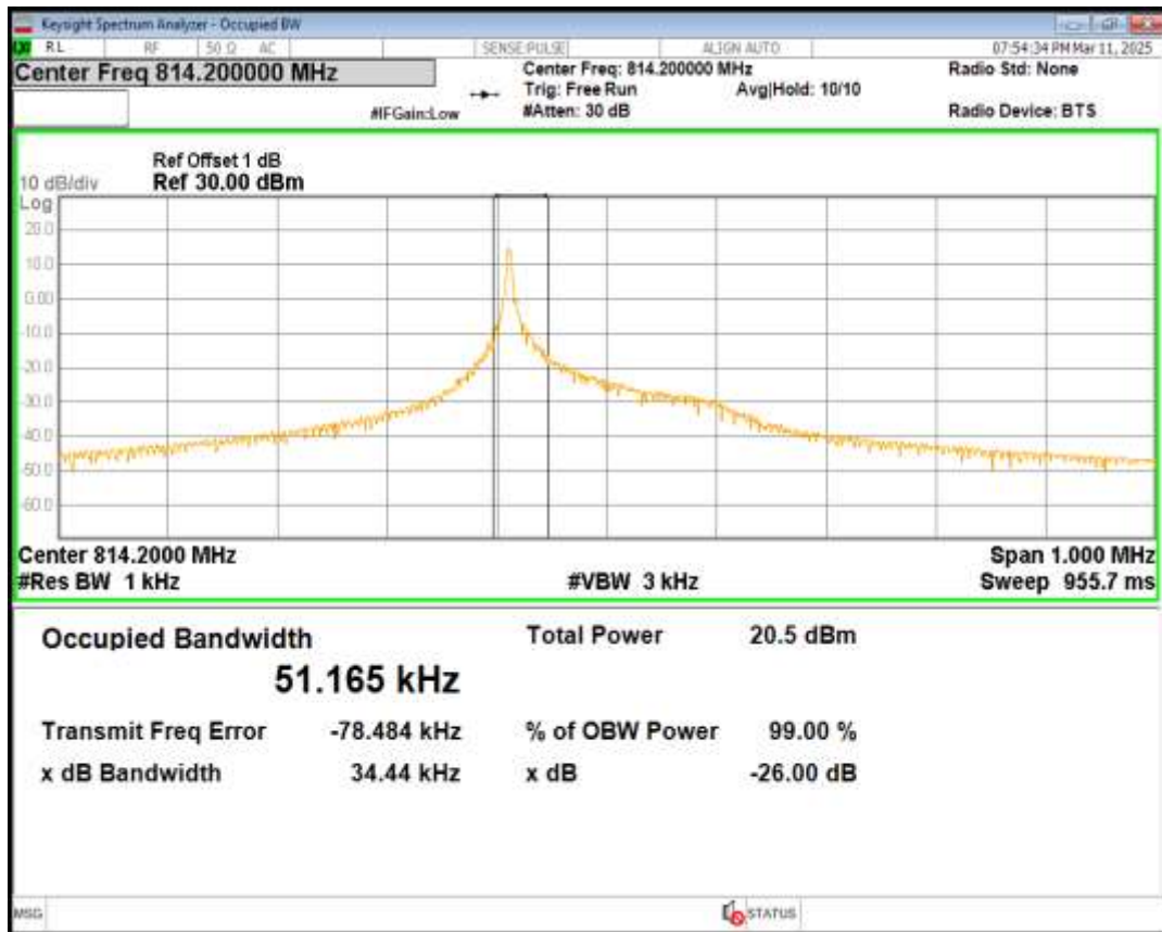
Band26 BPSK Channel=26865 nTones=1@0 Spacing=3.75kHz
