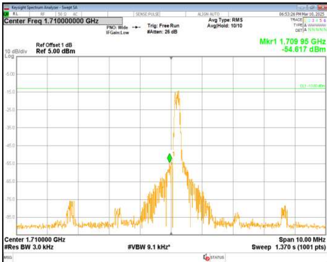
Band4 QPSK Channel=19952 nTones=1@0 Spacing=15kHz
