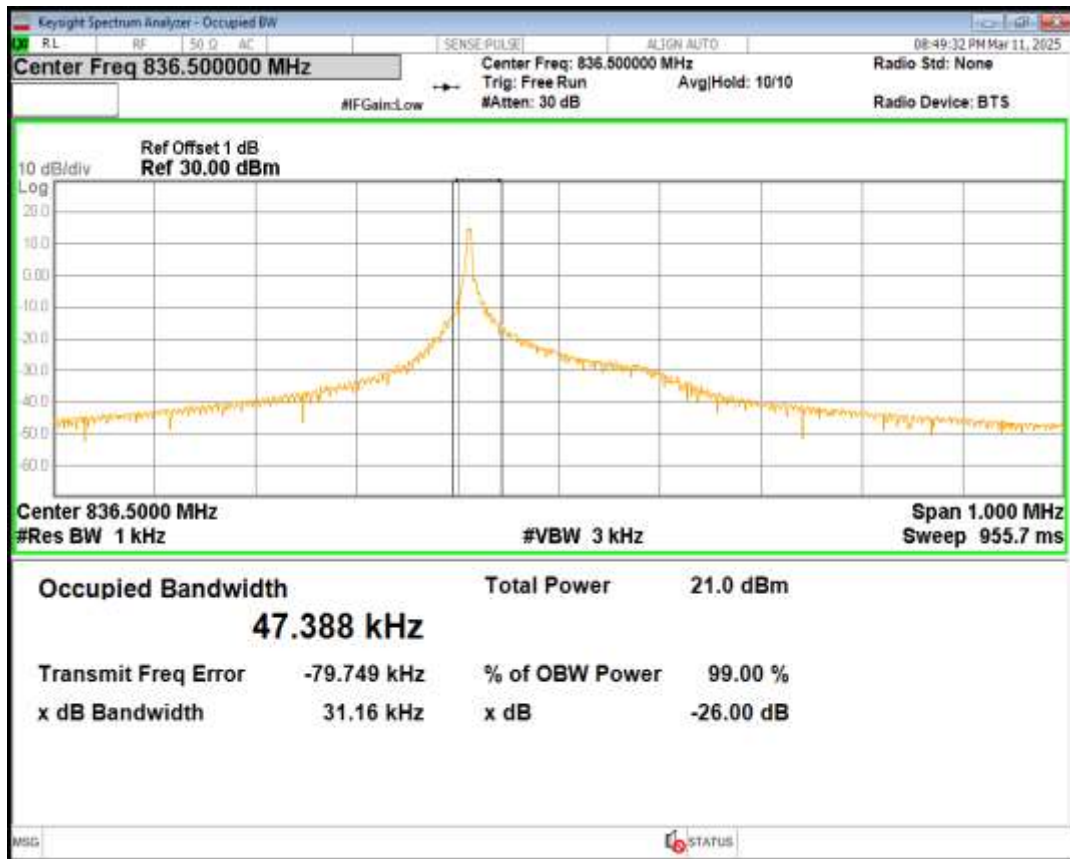
Band5 QPSK Channel=20648 nTones=1@0 Spacing=3.75kHz
