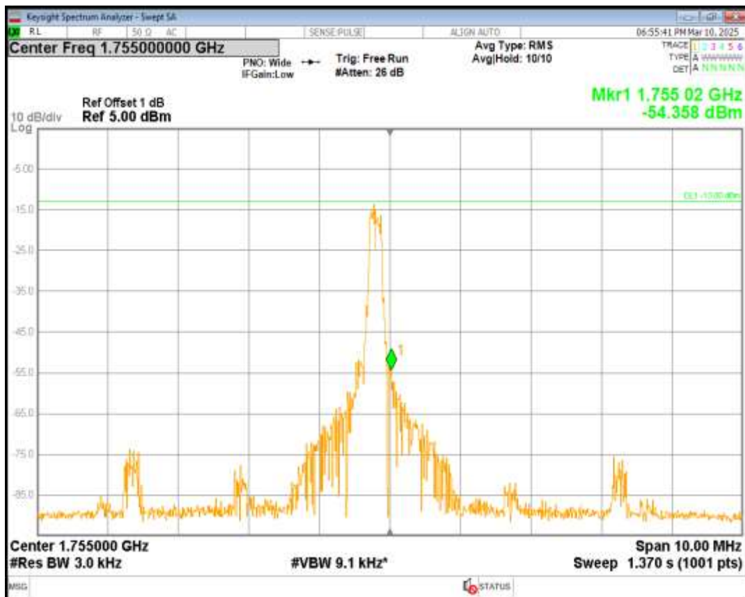
Band4 QPSK Channel=20398 nTones=1@11 Spacing=15kHz
