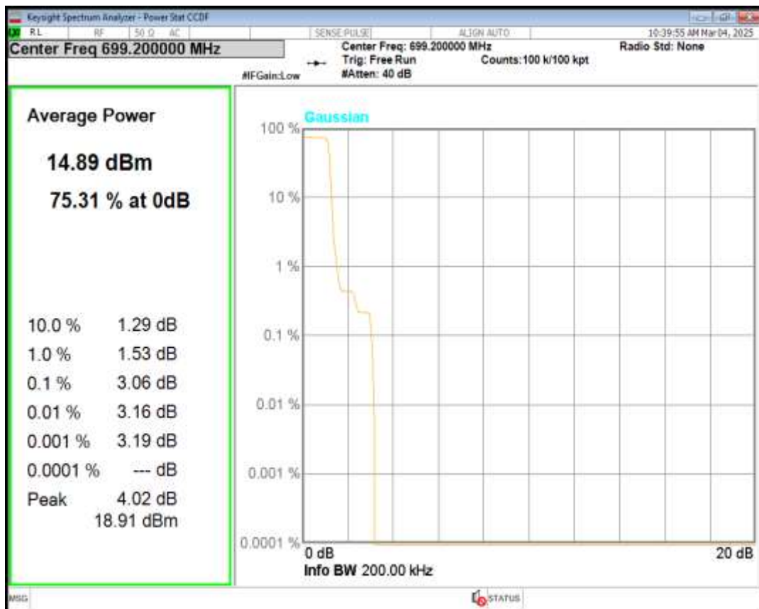
Band12 QPSK Channel=23095 nTones=1@0 Spacing=3.75kHz
