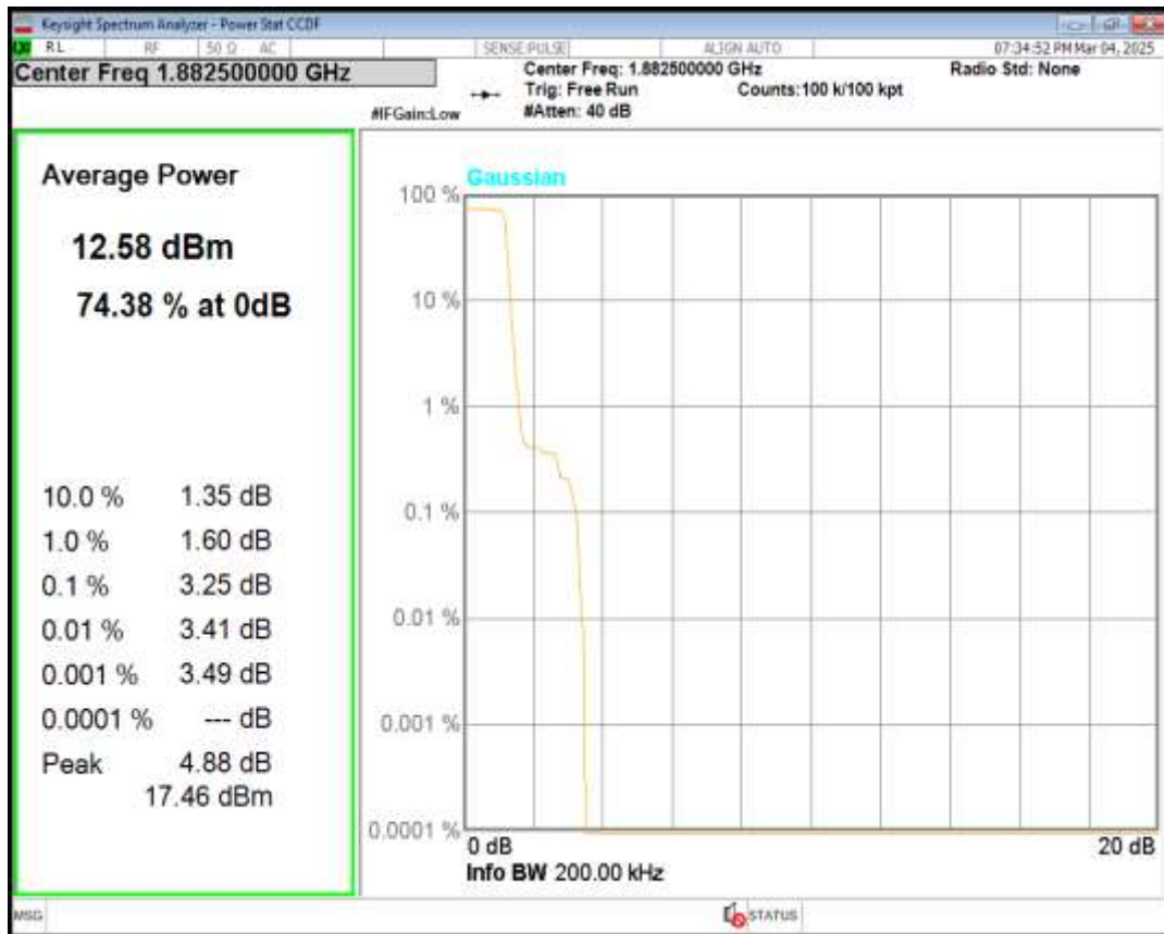
Band25 QPSK Channel=26688 nTones=1@0 Spacing=3.75kHz
