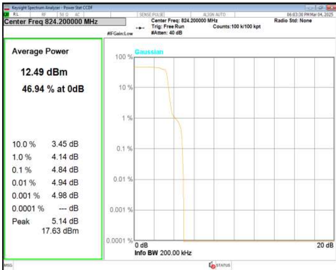
Band5 QPSK Channel=20525 nTones=1@0 Spacing=15kHz
