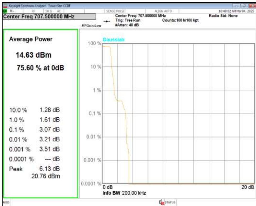
Band12 BPSK Channel=23178 nTones=1@0 Spacing=3.75kHz
