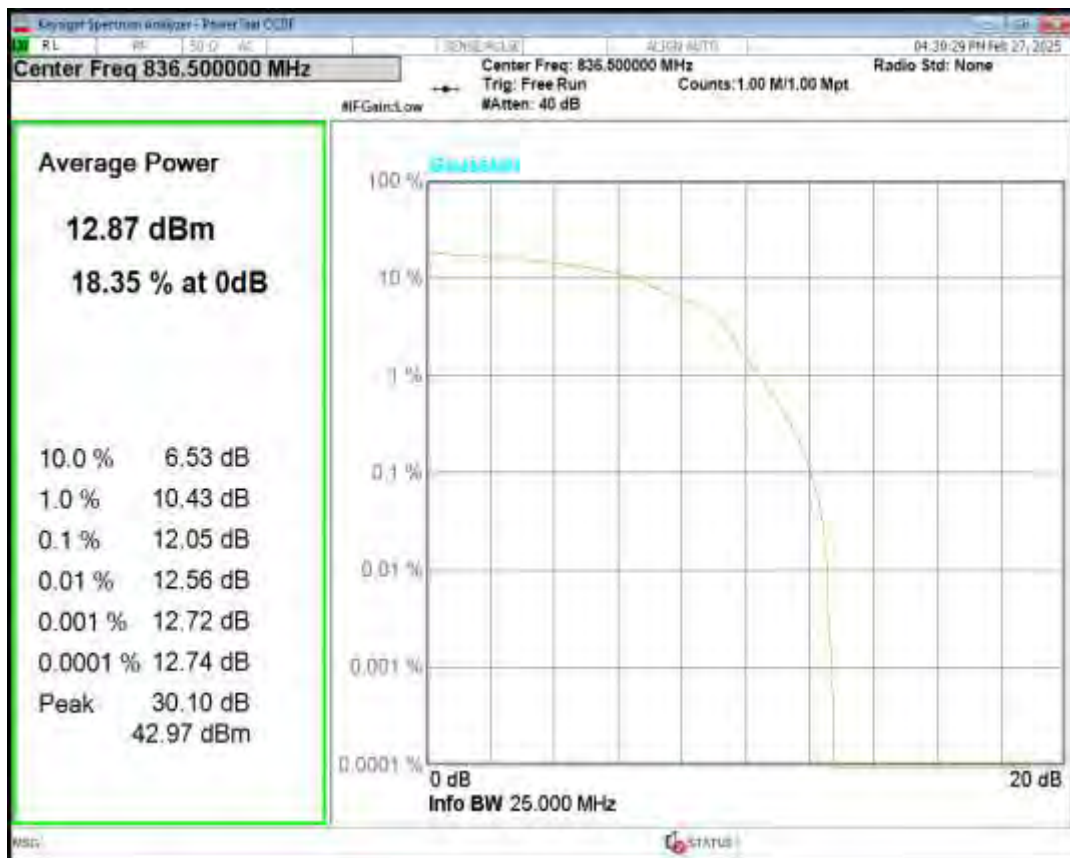
Band5 QPSK BW=3MHz Channel=20635 RB Size=6 Position=#0 NB Index=0
