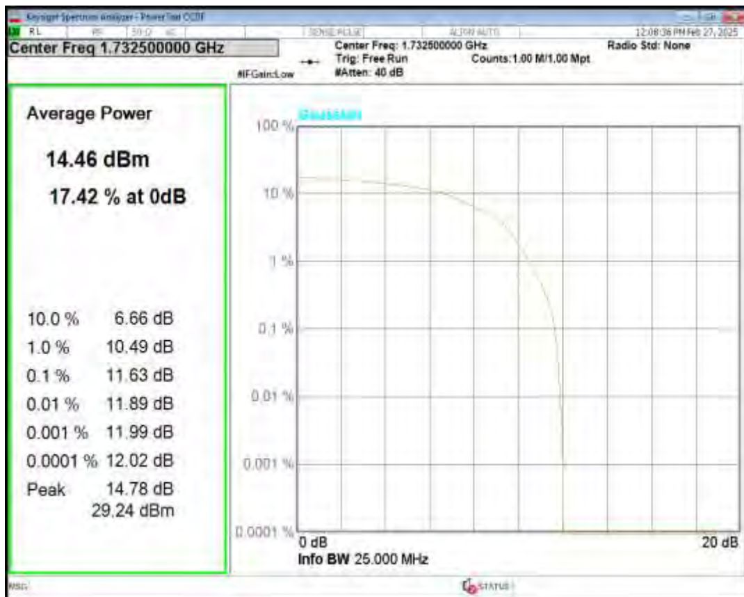
Band4 QPSK BW=20MHz Channel=20300 RB Size=6 Position=#0 NB Index=0
