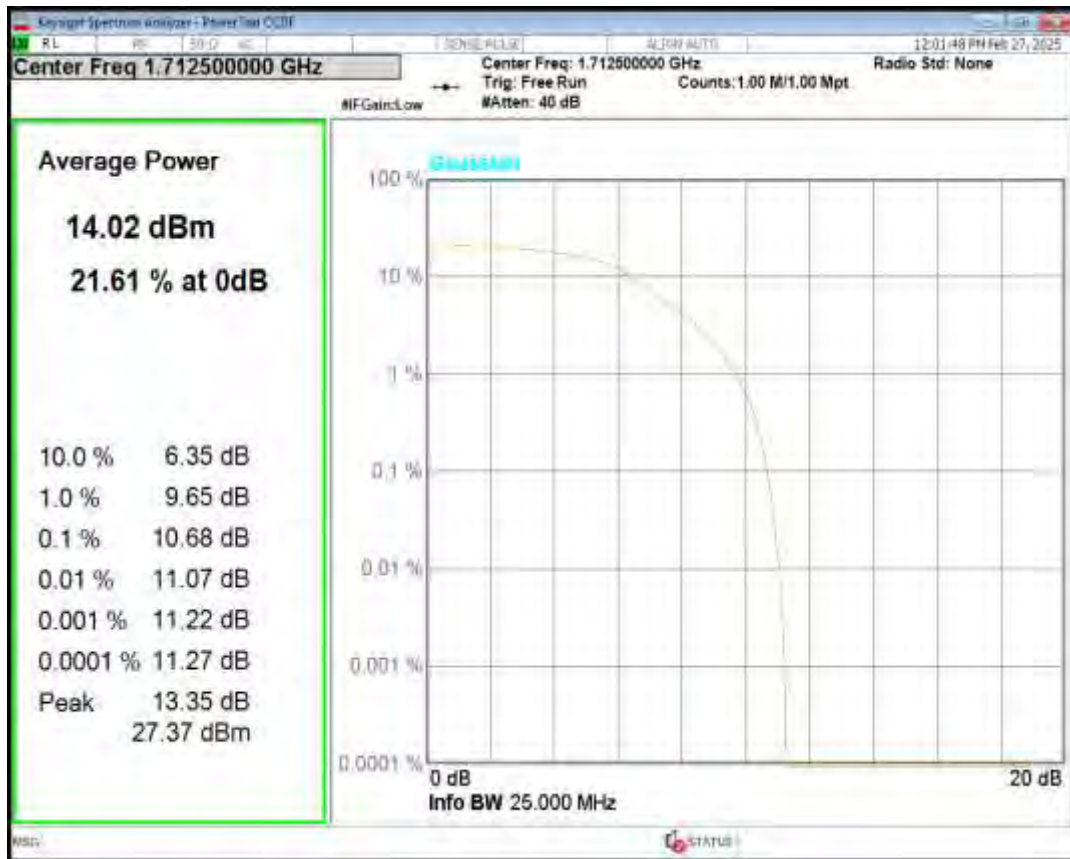
Band4 16QAM BW=5MHz Channel=19975 RB Size=5 Position=#0 NB Index=0
