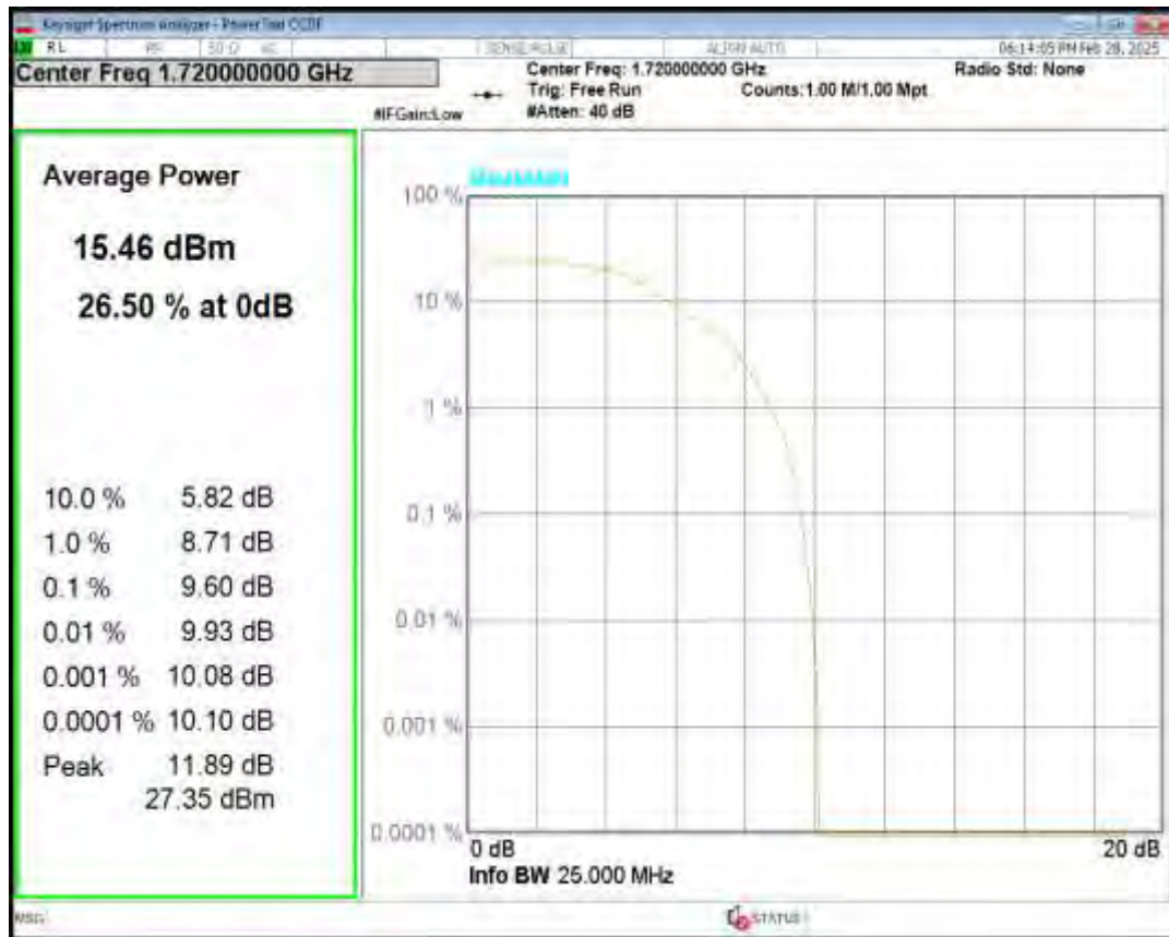
Band66 16QAM BW=20MHz Channel=132072 RB Size=5 Position=#0 NB Index=0
