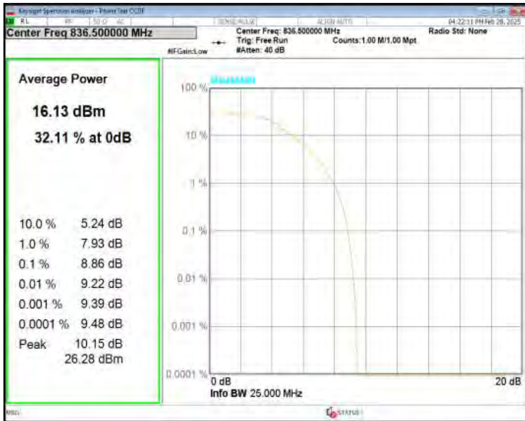
Band26(824-849) 16QAM BW=10MHz Channel=26915 RB Size=5 Position=#0 NB Index=0
