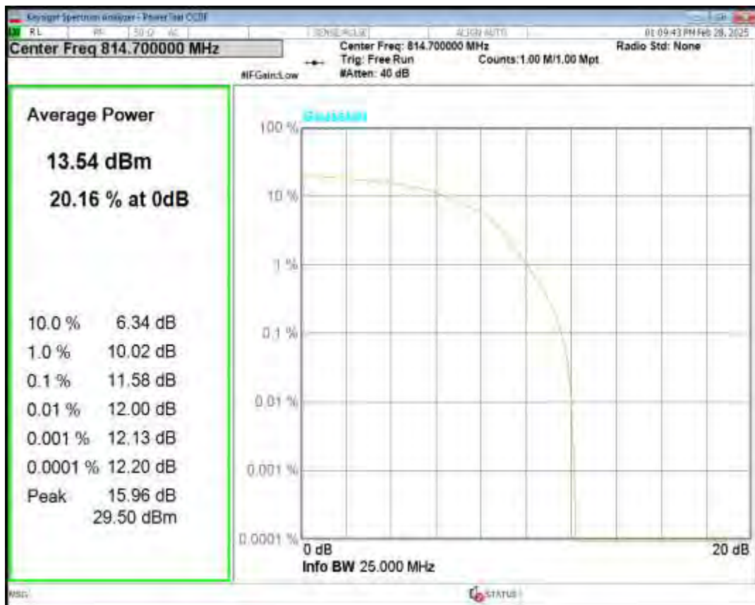
Band26(814-824) QPSK BW=1.4MHz Channel=26740 RB Size=6 Position=#0 NB Index=0
