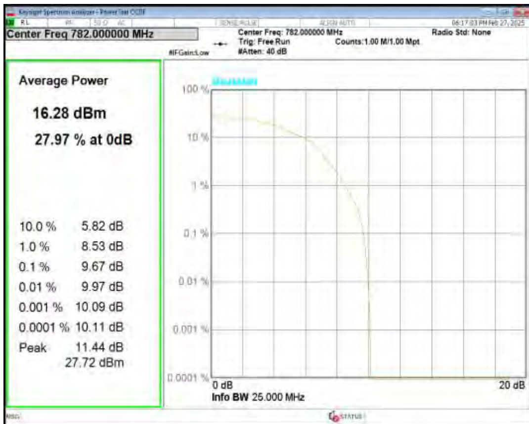
Band13 QPSK BW=5MHz Channel=23255 RB Size=6 Position=#0 NB Index=0
