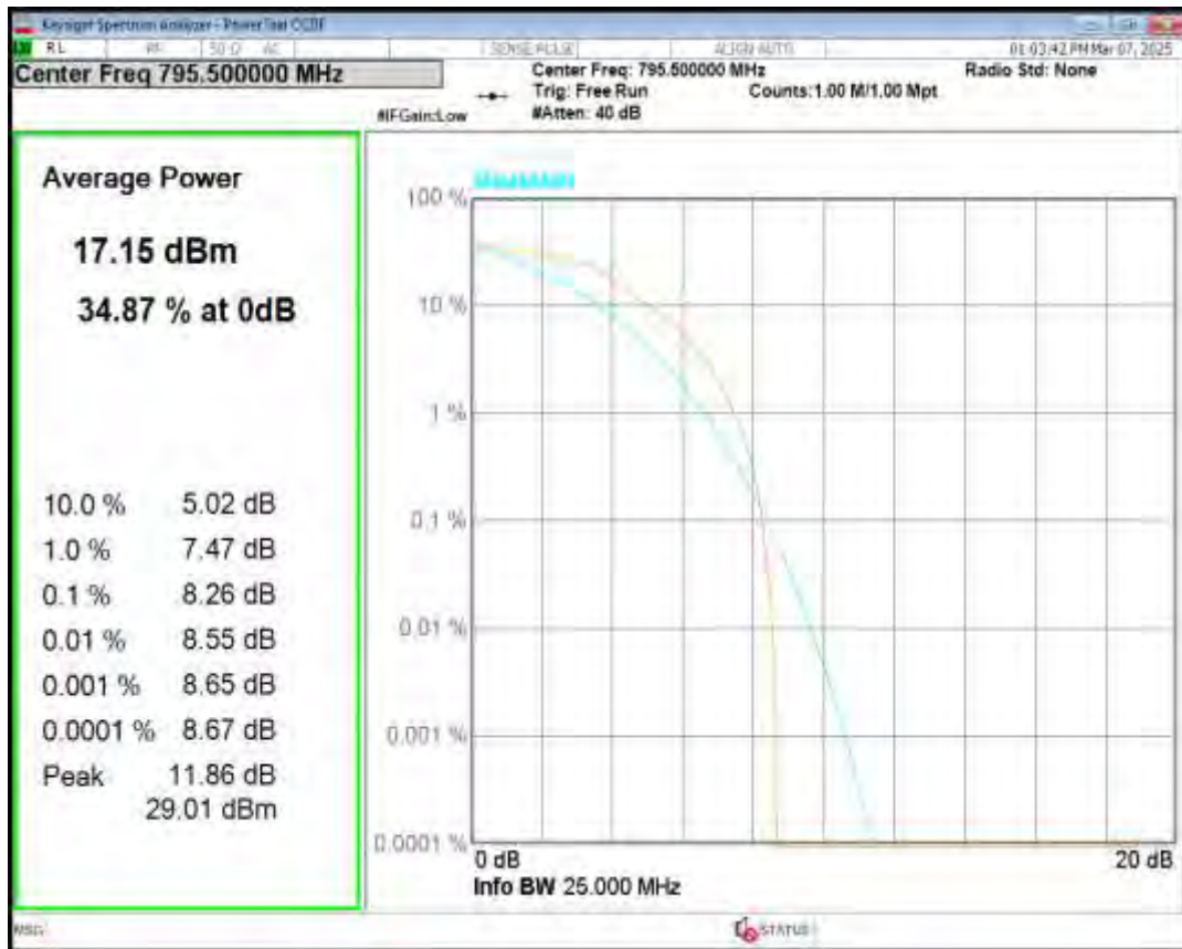
Band14 16QAM BW=5MHz Channel=23355 RB Size=5 Position=#0 NB Index=0
