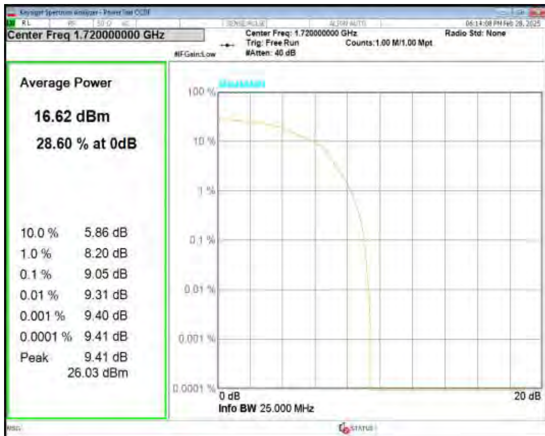
Band66 QPSK BW=20MHz Channel=132322 RB Size=6 Position=#0 NB Index=0
