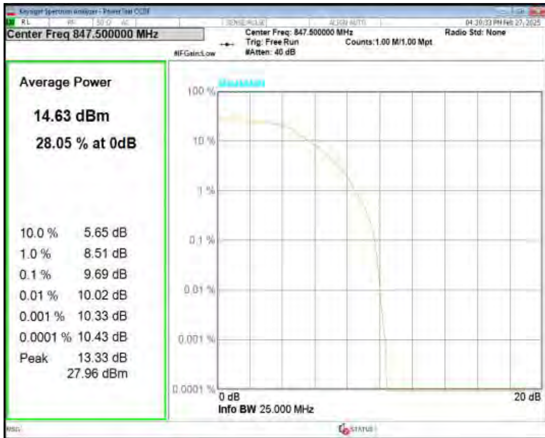
Band5 16QAM BW=3MHz Channel=20635 RB Size=5 Position=#0 NB Index=0
