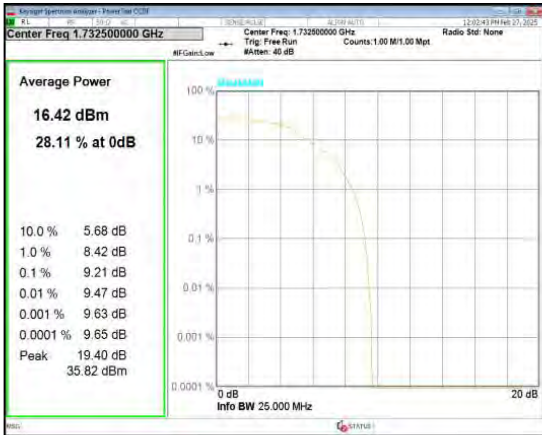
Band4 16QAM BW=15MHz Channel=20175 RB Size=5 Position=#0 NB Index=0
