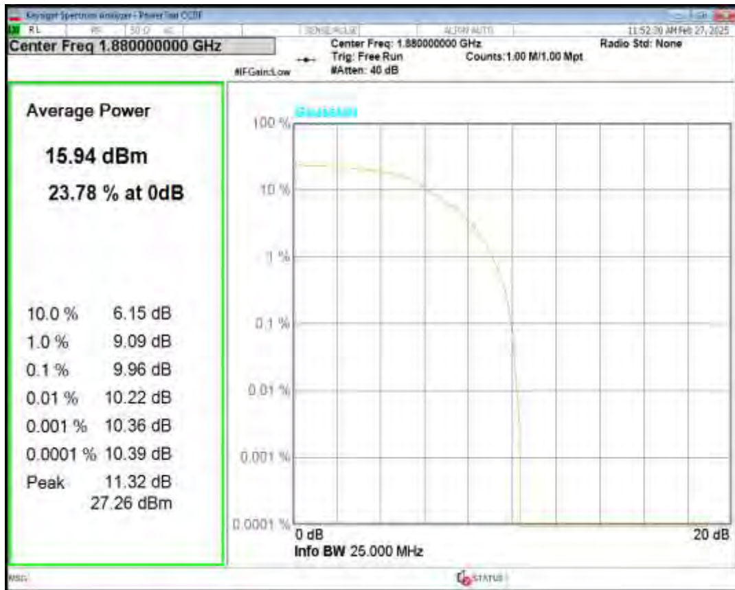
Band2 16QAM BW=15MHz Channel=18900 RB Size=5 Position=#0 NB Index=0
