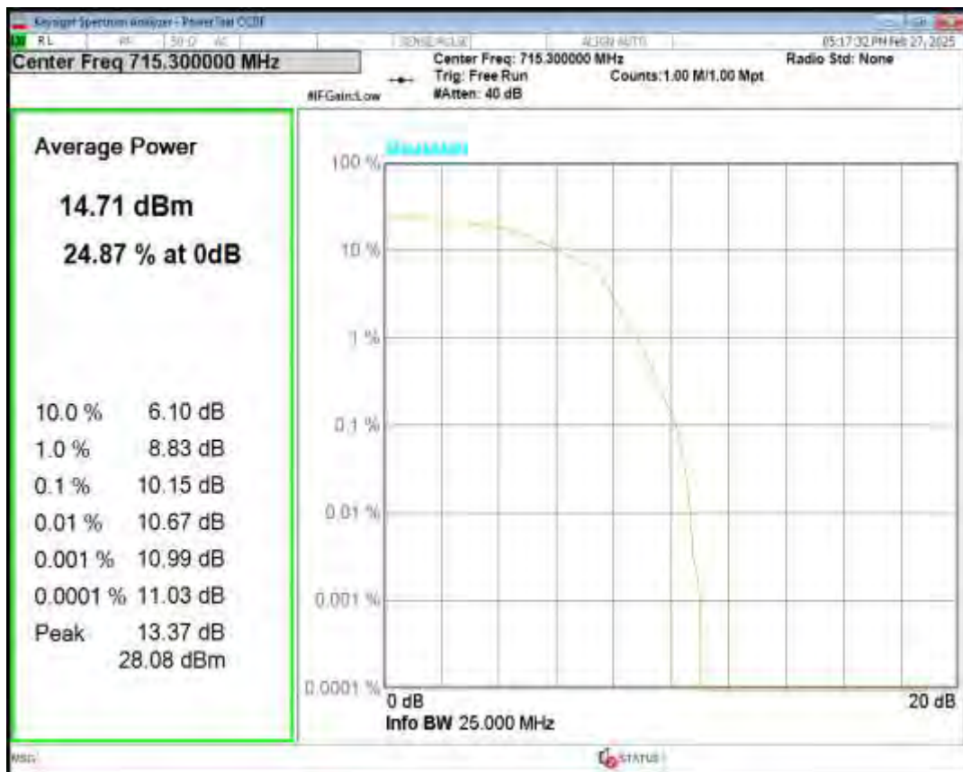
Band12 QPSK BW=3MHz Channel=23025 RB Size=6 Position=#0 NB Index=0
