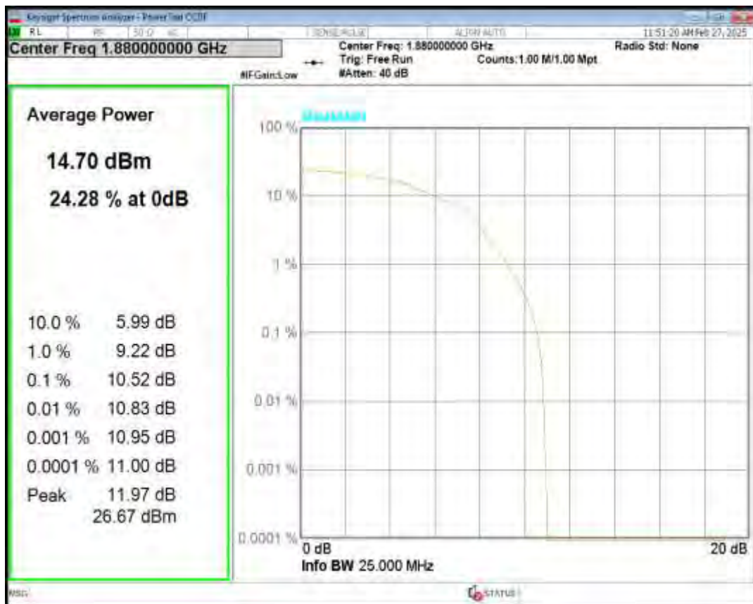
Band2 QPSK BW=3MHz Channel=19185 RB Size=6 Position=#0 NB Index=0
