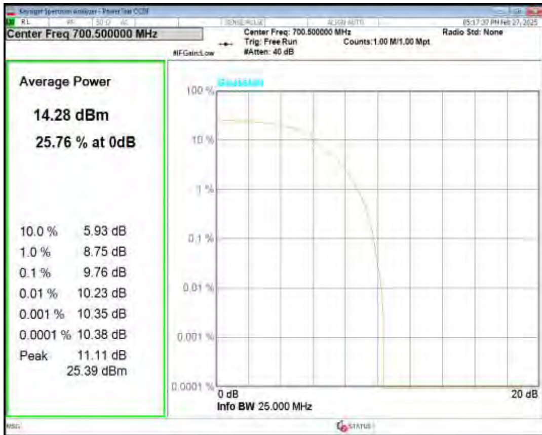
Band12 16QAM BW=3MHz Channel=23025 RB Size=5 Position=#0 NB Index=0
