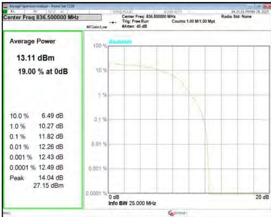
Band26(824-849) QPSK BW=1.4MHz Channel=27033 RB Size=6 Position=#0 NB Index=0
