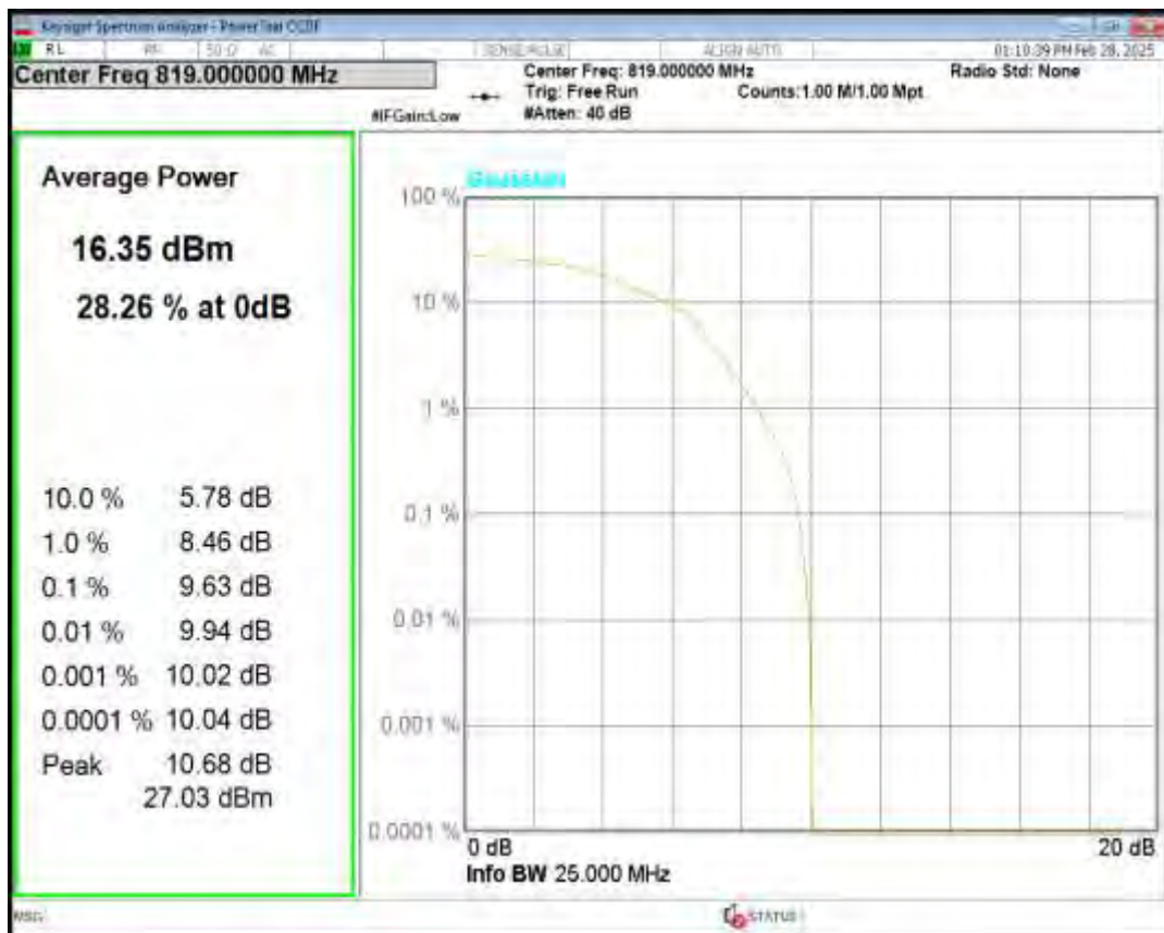
Band26(814-824) QPSK BW=5MHz Channel=26765 RB Size=6 Position=#0 NB Index=0
