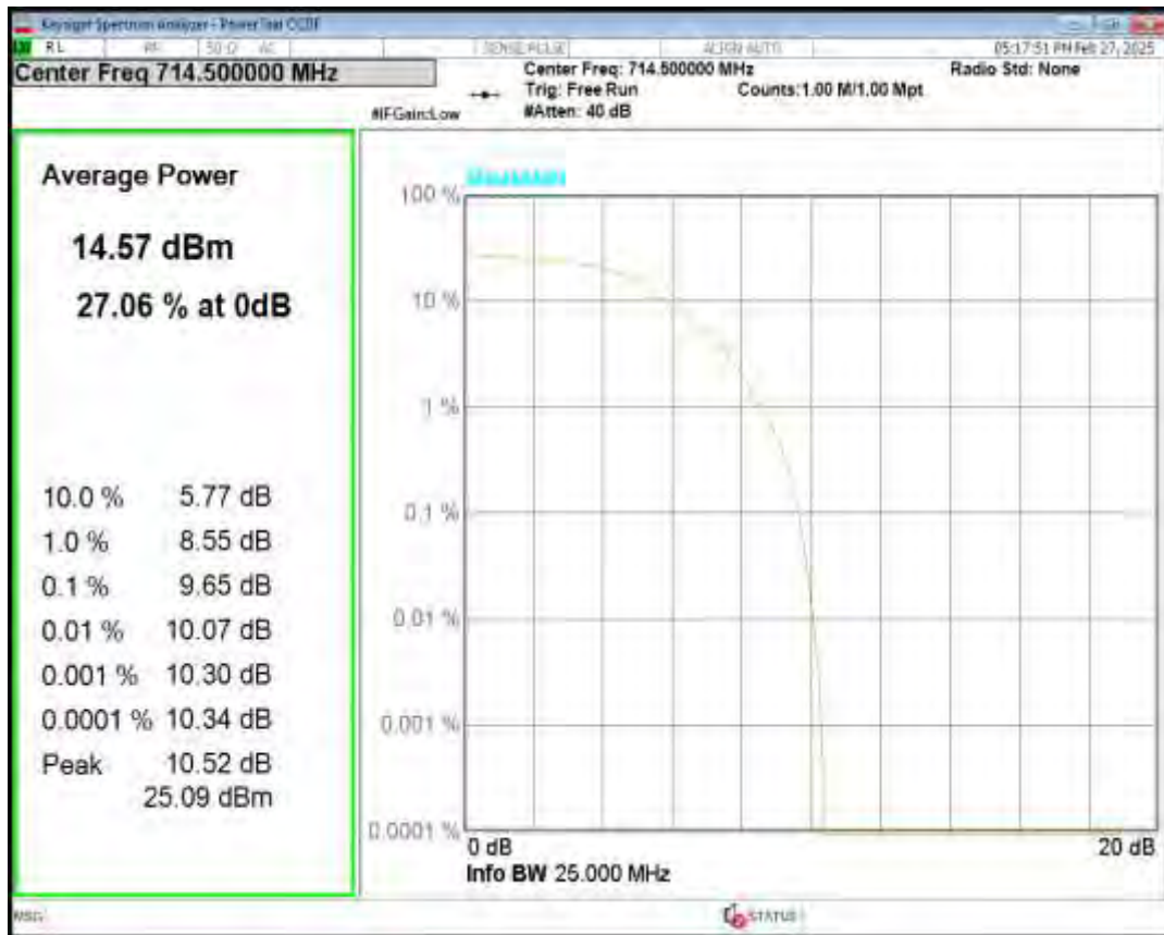
Band12 16QAM BW=3MHz Channel=23165 RB Size=5 Position=#0 NB Index=0
