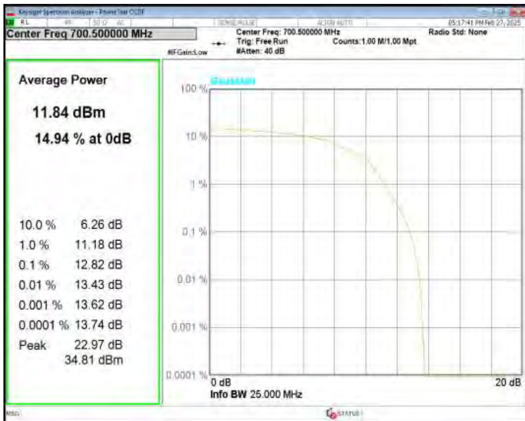
Band12 QPSK BW=3MHz Channel=23095 RB Size=6 Position=#0 NB Index=0
