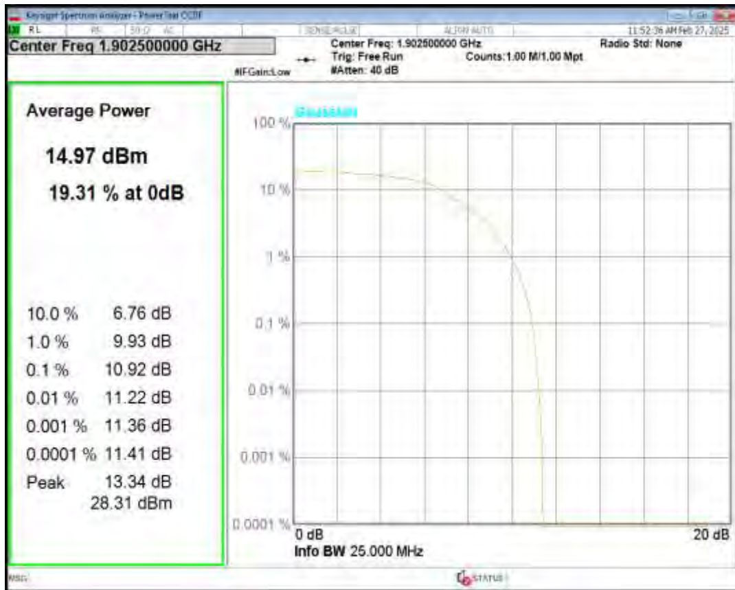
Band2 16QAM BW=15MHz Channel=19125 RB Size=5 Position=#0 NB Index=0
