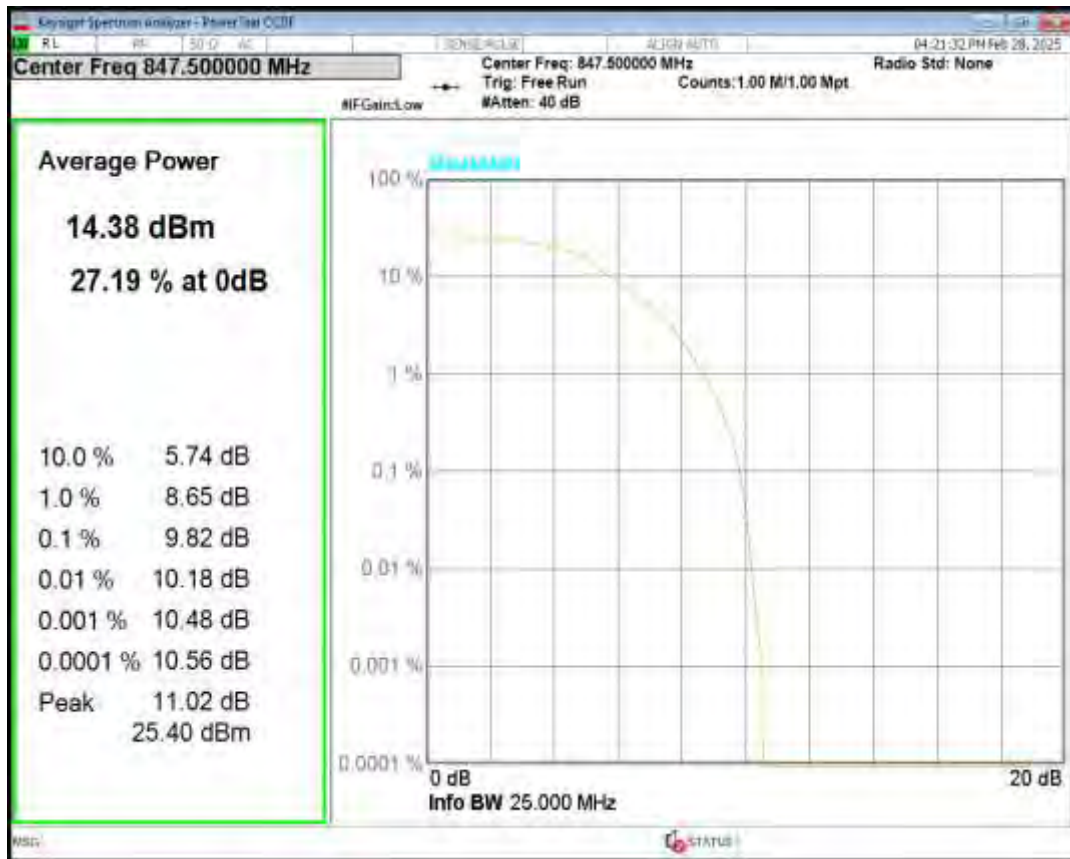
Band26(824-849) 16QAM BW=3MHz Channel=27025 RB Size=5 Position=#0 NB Index=0
