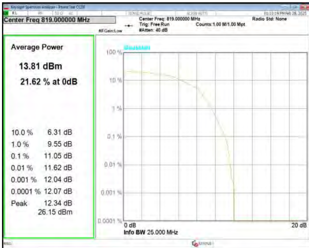
Band26(814-824) QPSK BW=3MHz Channel=26775 RB Size=6 Position=#0 NB Index=0
