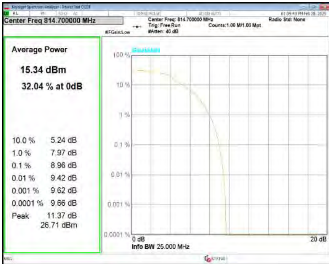
Band26(814-824) 16QAM BW=1.4MHz Channel=26697 RB Size=5 Position=#0 NB Index=0
