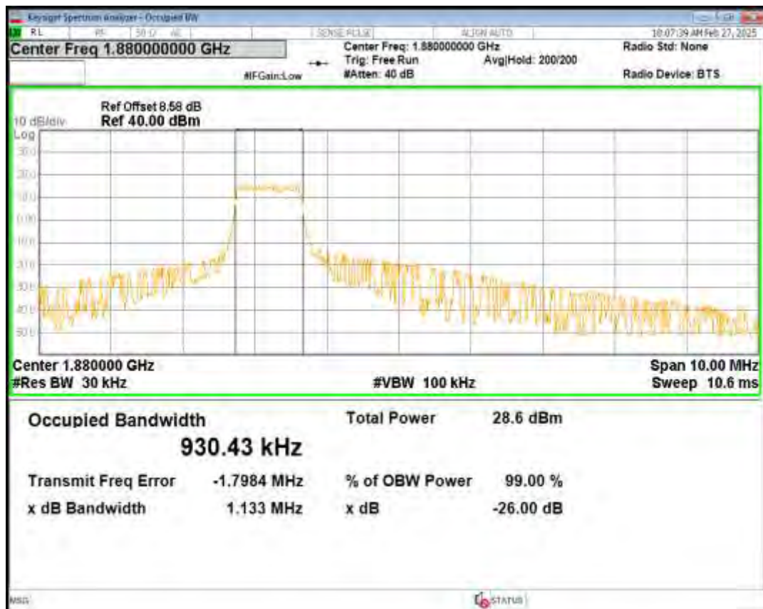
Band2 QPSK BW=5MHz Channel=19175 RB Size=6 Position=#0 NB Index=0
