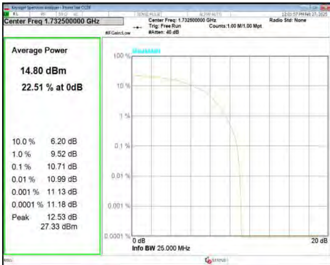
Band4 QPSK BW=5MHz Channel=20375 RB Size=6 Position=#0 NB Index=0
