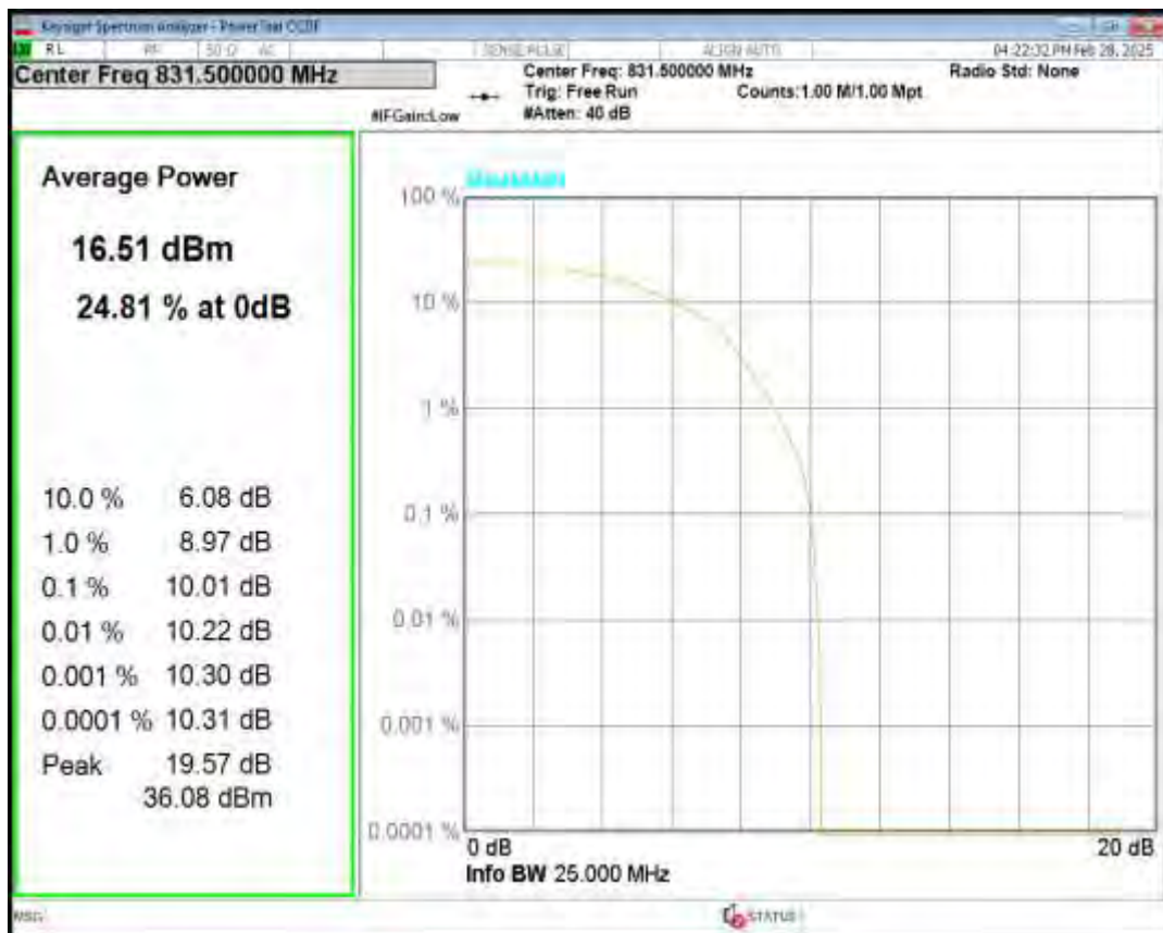
Band26(824-849) QPSK BW=15MHz Channel=26915 RB Size=6 Position=#0 NB Index=0
