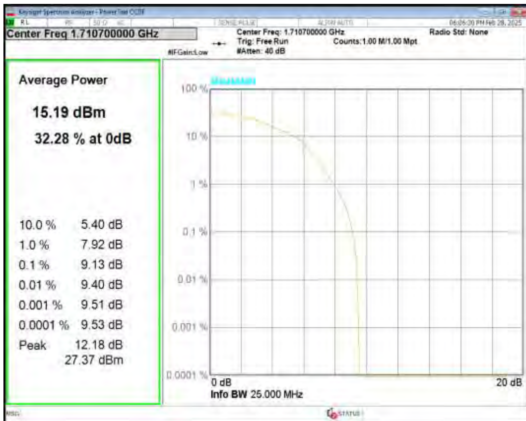
Band66 QPSK BW=1.4MHz Channel=132322 RB Size=6 Position=#0 NB Index=0
