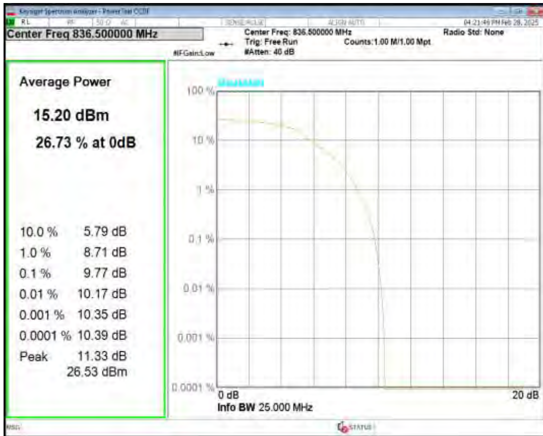
Band26(824-849) 16QAM BW=5MHz Channel=26915 RB Size=5 Position=#0 NB Index=0
