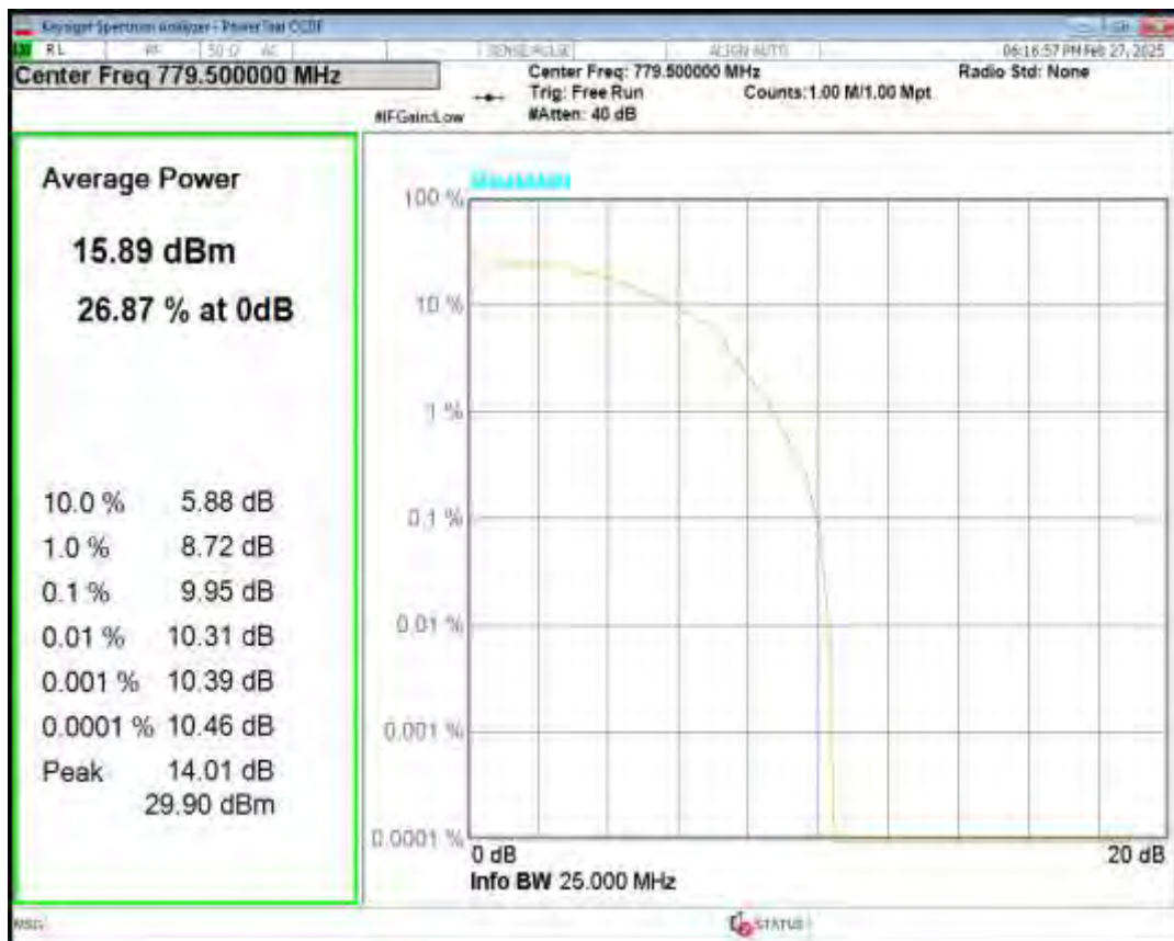
Band13 QPSK BW=5MHz Channel=23230 RB Size=6 Position=#0 NB Index=0
