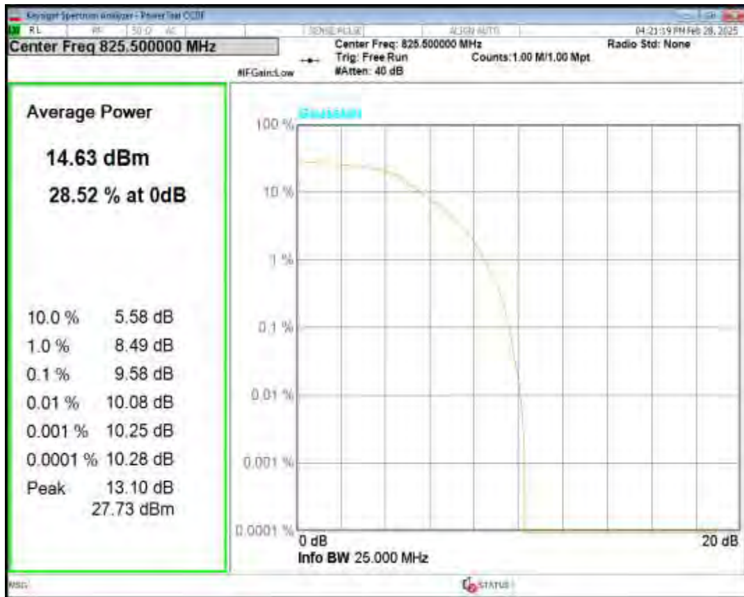
Band26(824-849) 16QAM BW=3MHz Channel=26805 RB Size=5 Position=#0 NB Index=0
