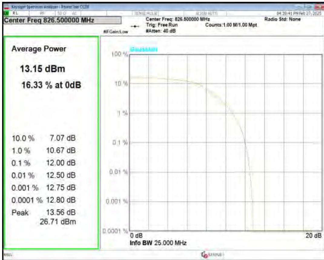
Band5 16QAM BW=5MHz Channel=20425 RB Size=5 Position=#0 NB Index=0
