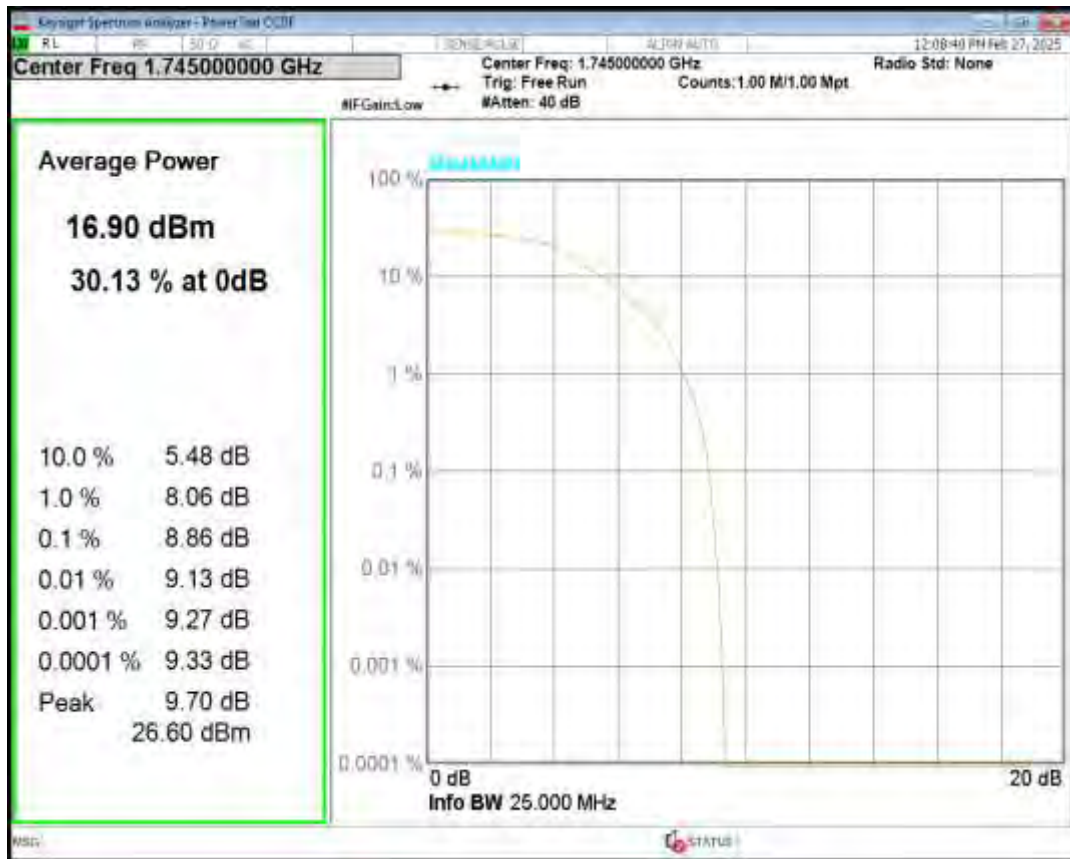
Band4 16QAM BW=20MHz Channel=20300 RB Size=5 Position=#0 NB Index=0
