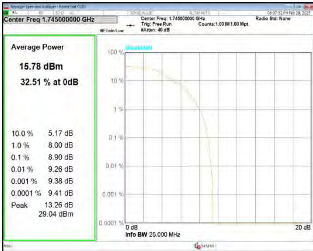
Band66 16QAM BW=10MHz Channel=132322 RB Size=5 Position=#0 NB Index=0
