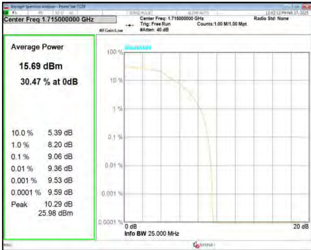
Band4 16QAM BW=10MHz Channel=20000 RB Size=5 Position=#0 NB Index=0
