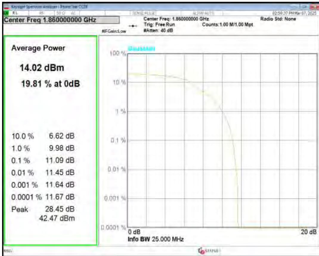
Band25 16QAM BW=20MHz Channel=26140 RB Size=5 Position=#0 NB Index=0
