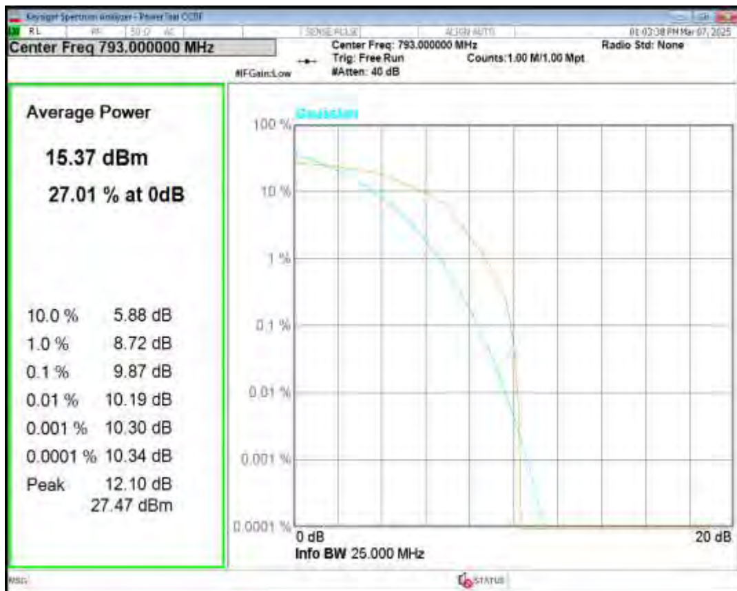
Band14 QPSK BW=5MHz Channel=23355 RB Size=6 Position=#0 NB Index=0
