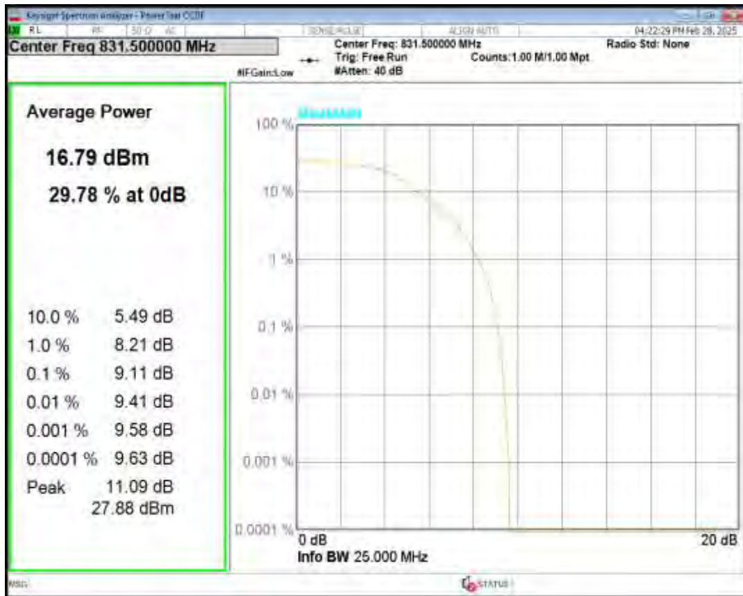
Band26(824-849) 16QAM BW=15MHz Channel=26865 RB Size=5 Position=#0 NB Index=0
