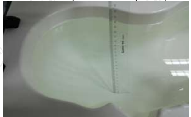
The Head Liquid of 1800MHz (15.2cm)
