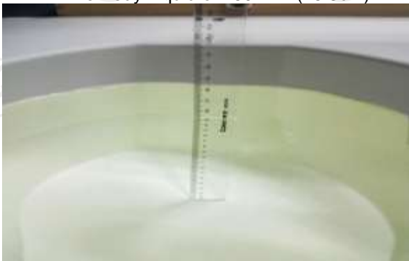
The Body Liquid of 1800MHz (15.2 cm)
