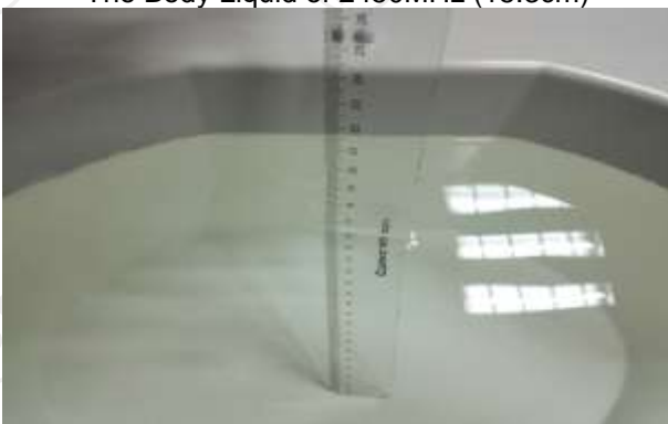
The Body Liquid of 5000-6000MHz (16.5cm)
