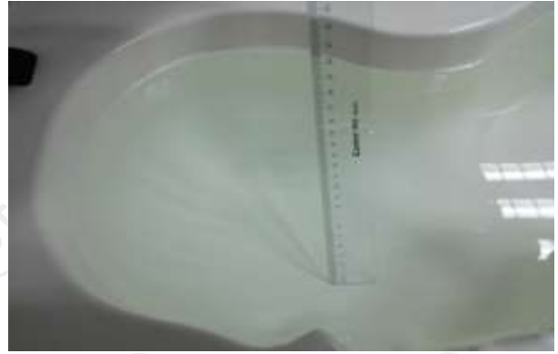
The Head Liquid of 2450MHz (15.6cm)
