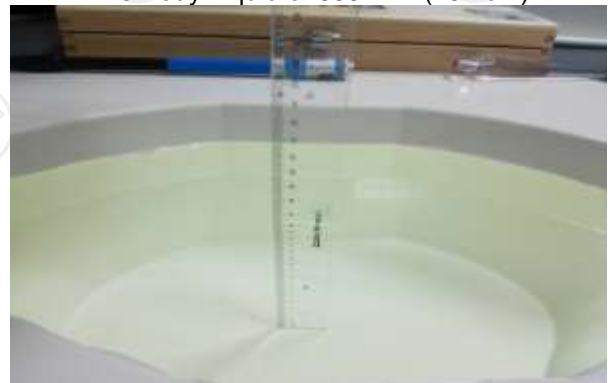
The Body Liquid of 1900MHz (16.4 cm)
