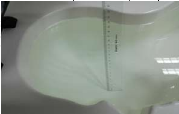
The Head Liquid of 2600MHz (15.1cm)
