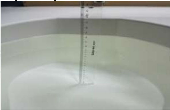
The Body Liquid of 750MHz (15.3cm)
