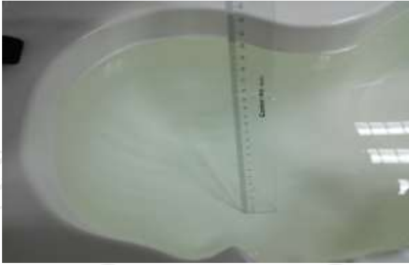
The Head Liquid of 1900MHz (15.5cm)
