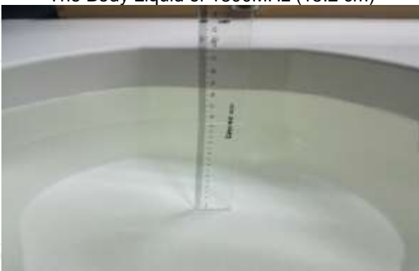
The Body Liquid of 2450MHz (15.3cm)
