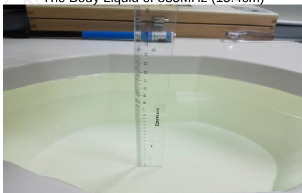
The Body Liquid of 1900MHz (16.4 cm)
