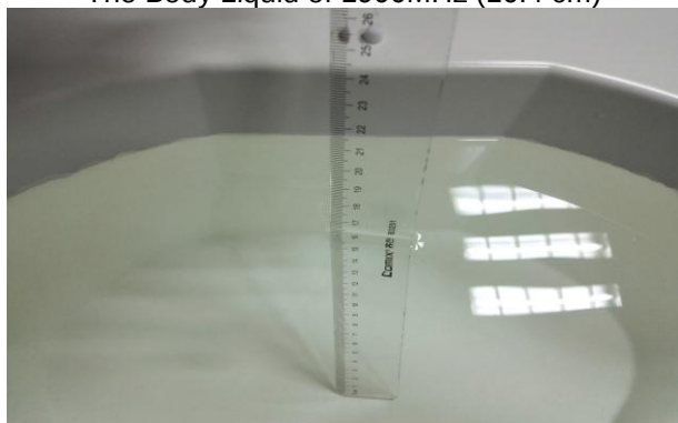
The Body Liquid of 2600MHz (16.5cm)
