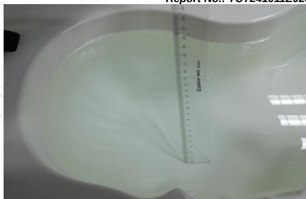
The Head Liquid of 2450MHz (15.6cm)
