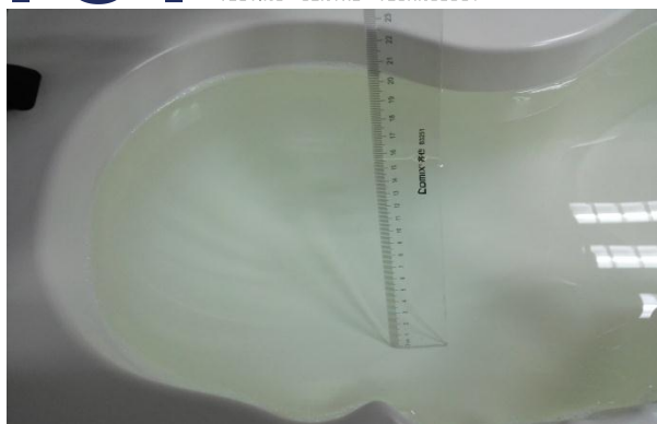
The Head Liquid of 1900MHz (15.5cm)
