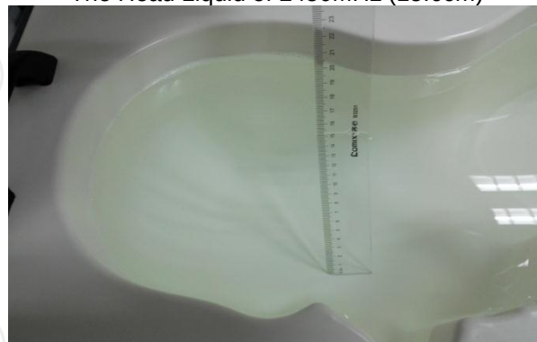
The Head Liquid of 1800MHz (15.2cm)
