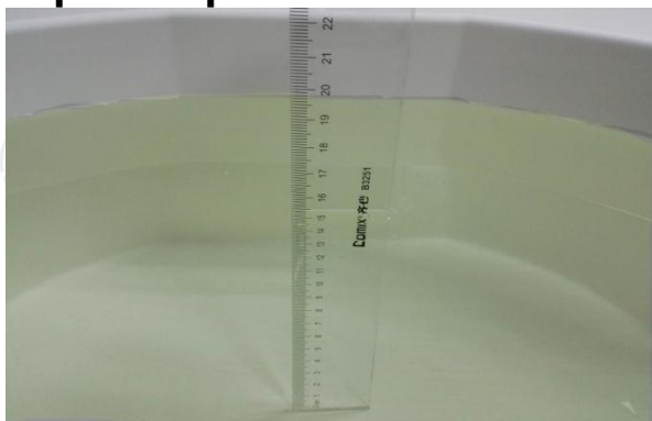
The Body Liquid of 835MHz (15.4cm)
