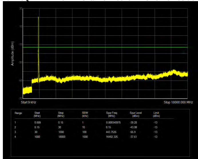
Band4 16QAM BW=15MHz Channel=20175 RB Size=75 Position=#0
