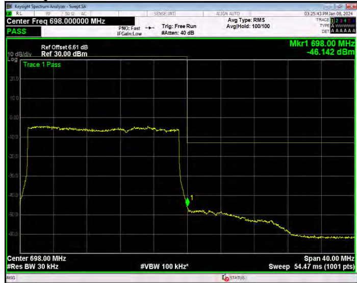
Band71 16QAM BW=20MHz Channel=133372 RB Size=100 Position=#0
