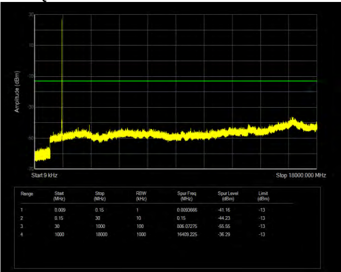
Band4 16QAM BW=1.4MHz Channel=20393 RB Size=6 Position=#0
