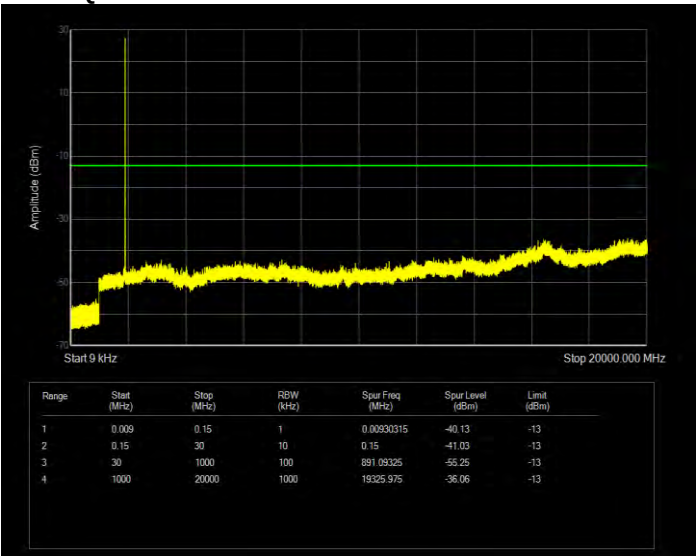
Band2 16QAM BW=1.4MHz Channel=19193 RB Size=6 Position=#0
