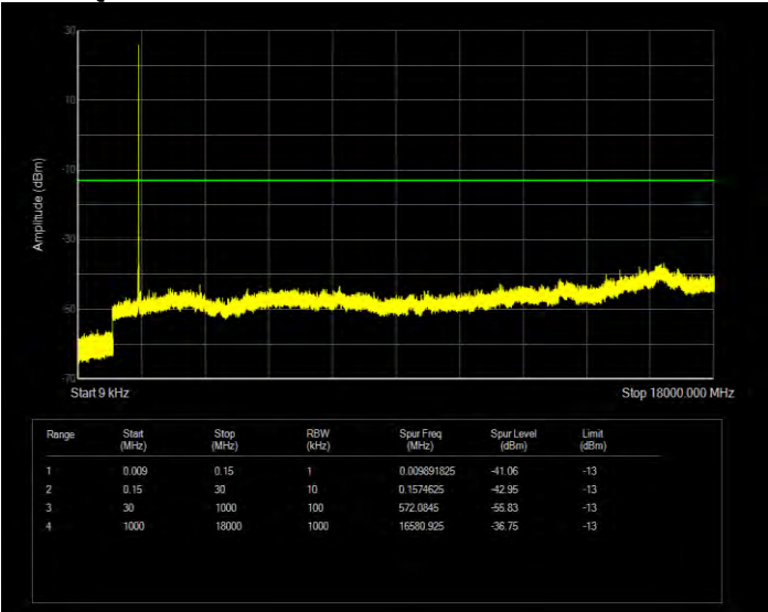
Band4 16QAM BW=1.4MHz Channel=20393 RB Size=6 Position=#0
