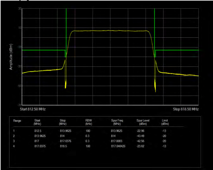
Band26(814-824) QPSK BW=3MHz Channel=26775 RB Size=1 Position=#0 Extended
