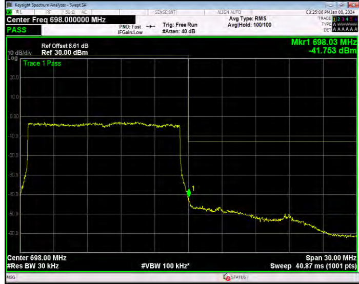
Band71 16QAM BW=20MHz Channel=133222 RB Size=100 Position=#0
