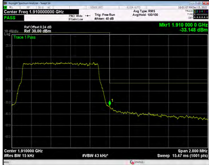
Band2 16QAM BW=10MHz Channel=18650 RB Size=50 Position=#0
