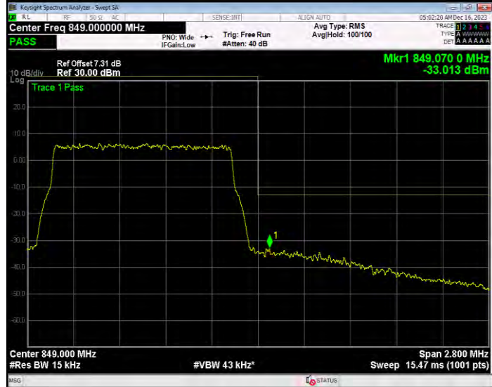
Band5 16QAM BW=10MHz Channel=20450 RB Size=50 Position=#0
