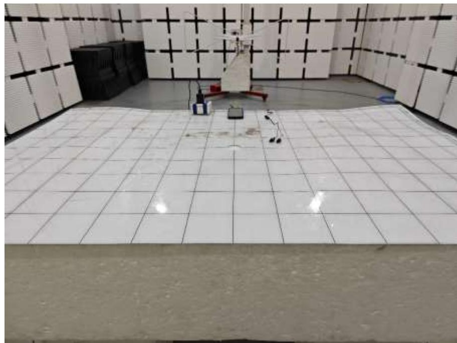
**Set-up for Radiated Emission (RE), Above 1GHz**
