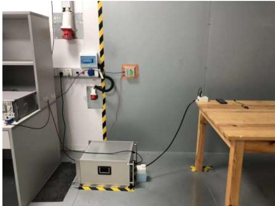
**Set-up for Radiated Emission (RE), Below 1GHz**
