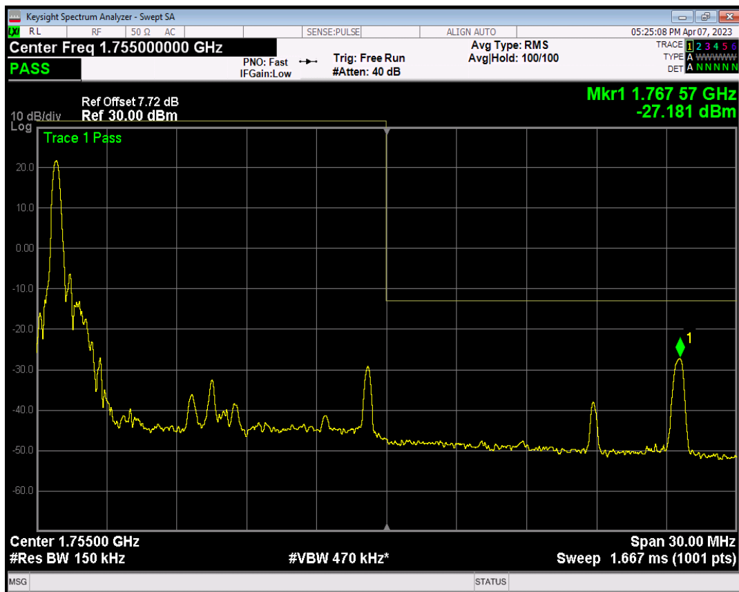
Band4 QAM16 BW=15MHz Channel=20325 RB Size=1 Position=#Max
