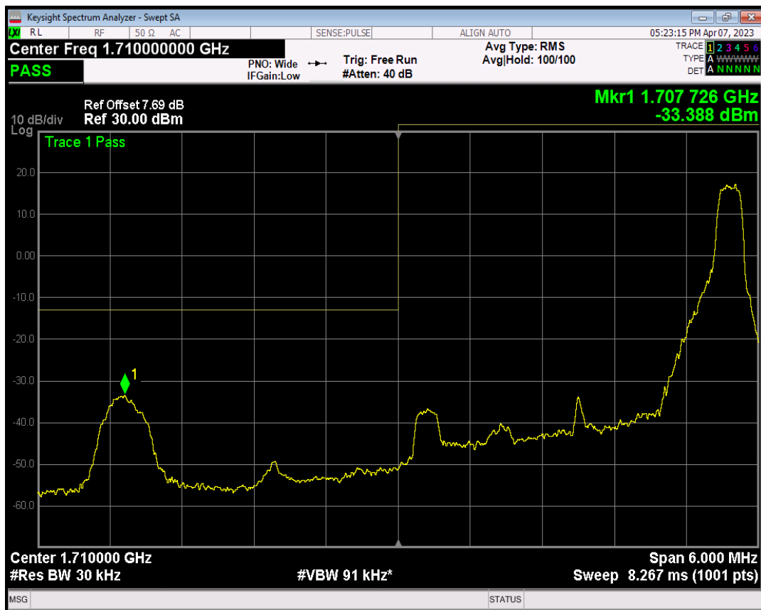
Band4 QPSK BW=3MHz Channel=19965 RB Size=15 Position=#0
