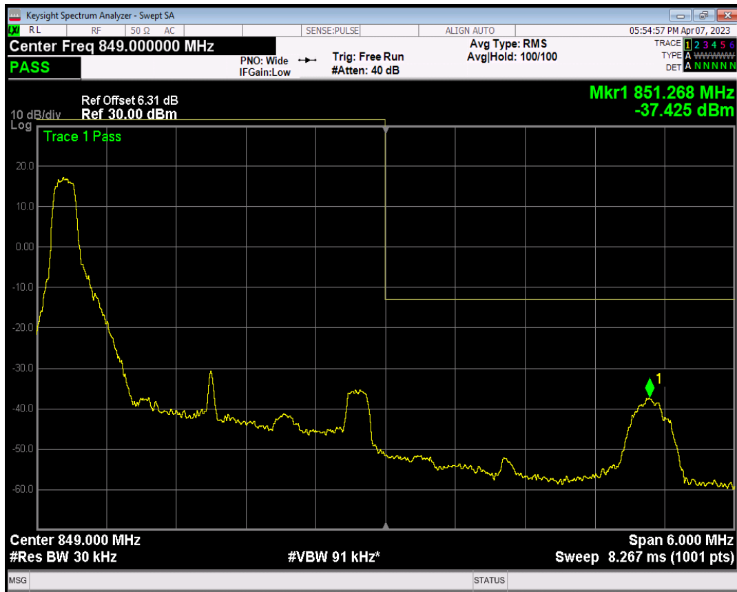
Band5 QPSK BW=3MHz Channel=20635 RB Size=1 Position=#Max
