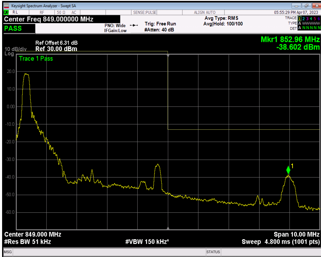
Band5 QPSK BW=5MHz Channel=20625 RB Size=1 Position=#Max
