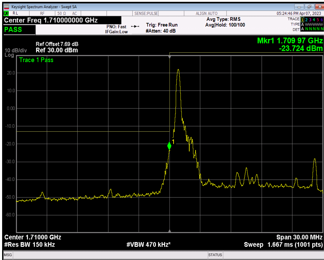
Band4 QPSK BW=15MHz Channel=20025 RB Size=1 Position=#Max
