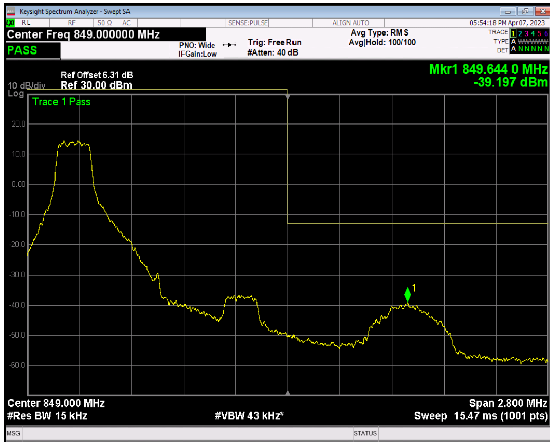
Band5 QPSK BW=1.4MHz Channel=20643 RB Size=1 Position=#Max
