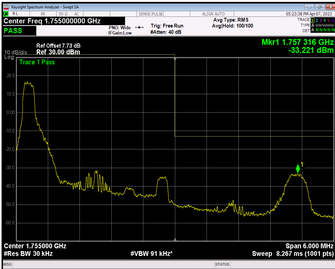
Band4 QAM16 BW=3MHz Channel=20385 RB Size=1 Position=#Max
