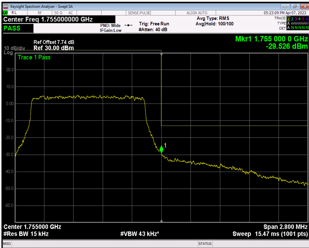
Band4 QPSK BW=3MHz Channel=19965 RB Size=1 Position=#0
