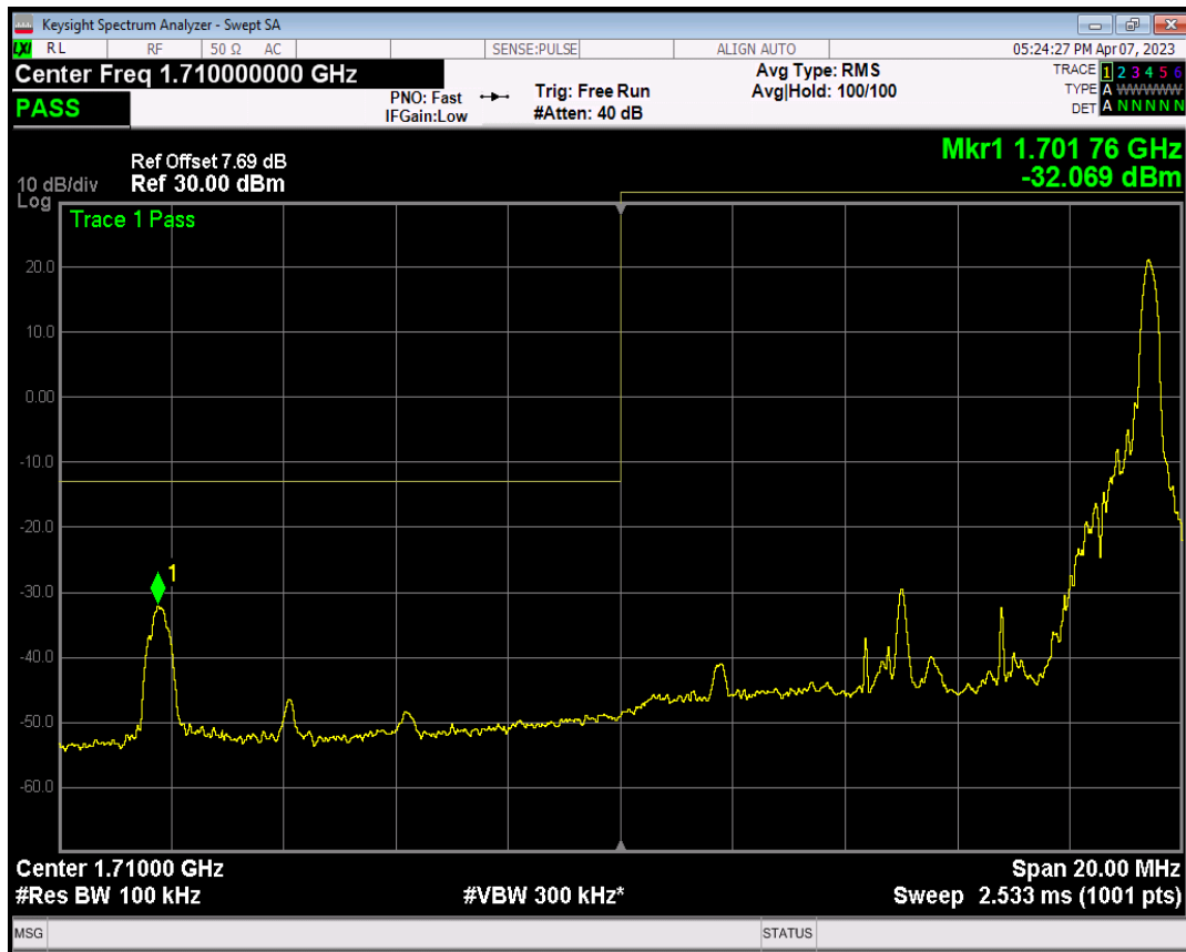
Band4 QAM16 BW=10MHz Channel=20000 RB Size=50 Position=#0
