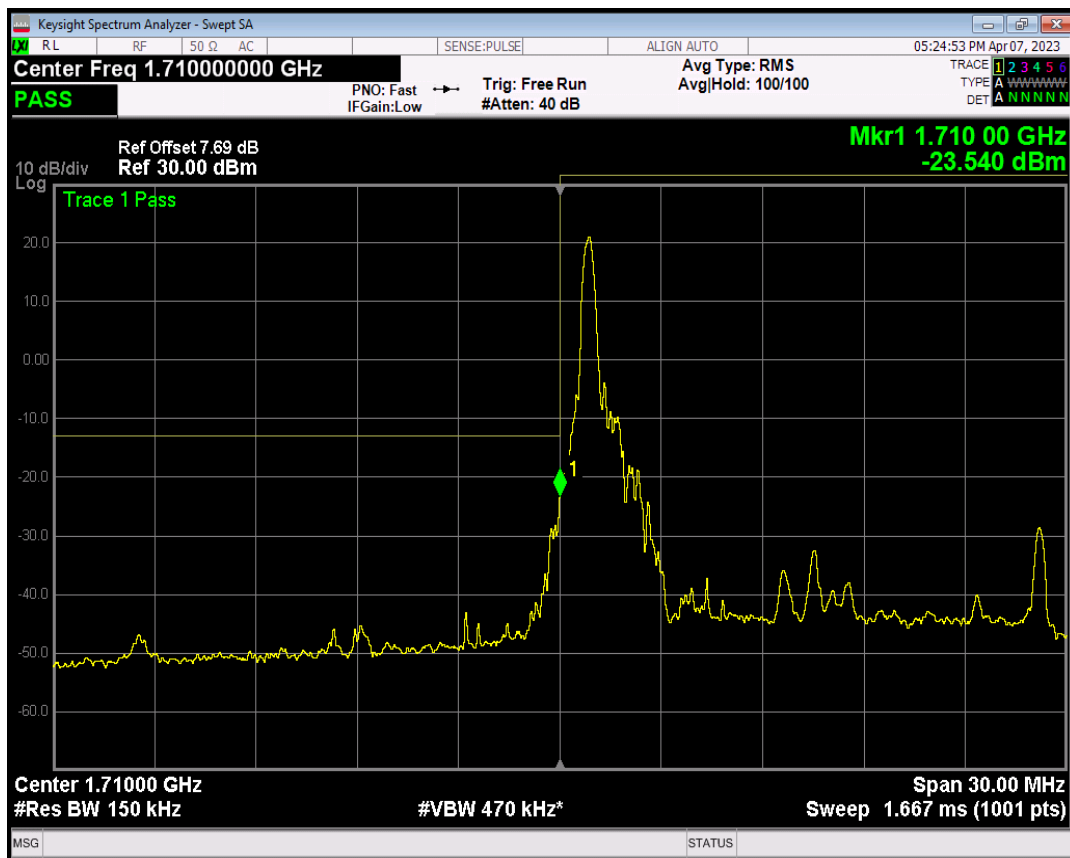
Band4 QAM16 BW=15MHz Channel=20025 RB Size=1 Position=#Max
