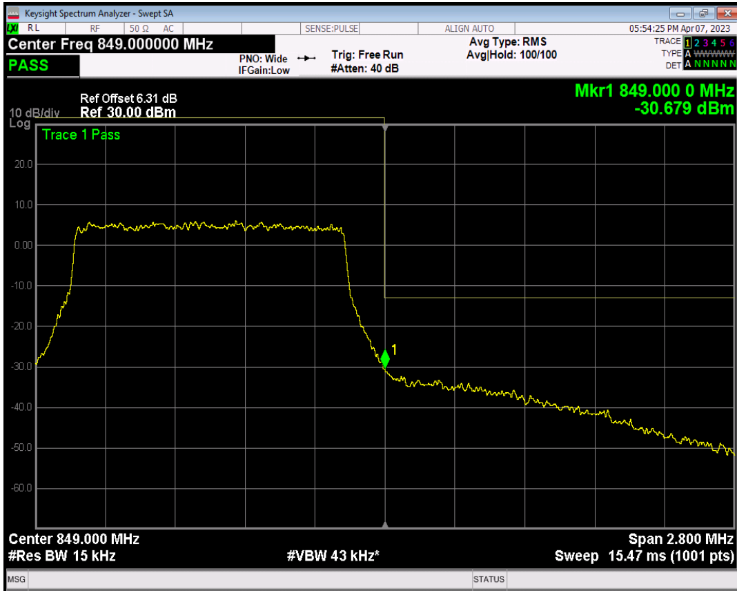
Band5 QAM16 BW=1.4MHz Channel=20643 RB Size=1 Position=#0
