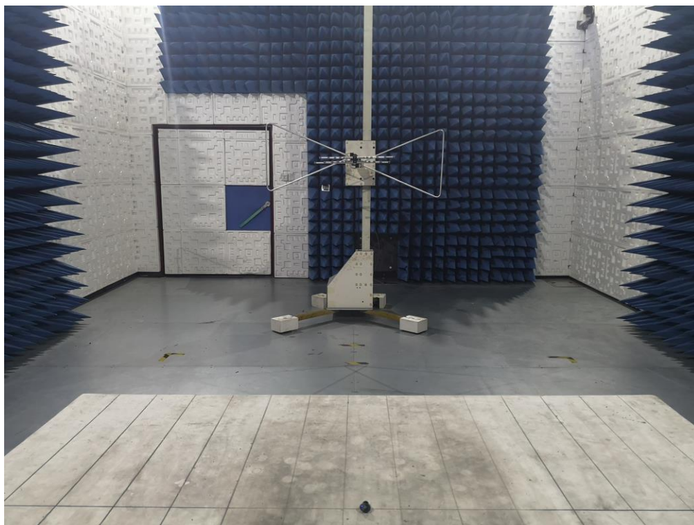
RADIATED EMISSION TEST SETUP ABOVE 1GHZ
