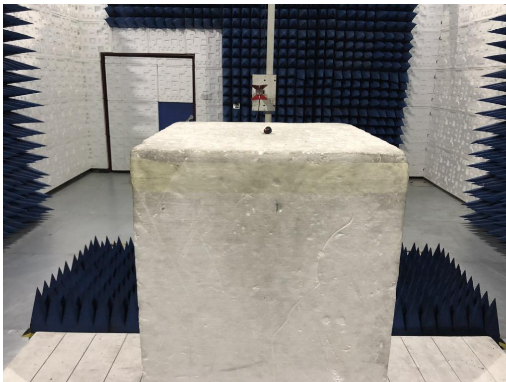
RADIATED EMISSION TEST SETUP ABOVE 1GHZ
