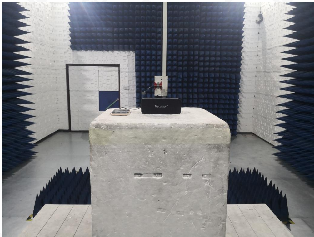
RADIATED EMISSION TEST SETUP ABOVE 1GHZ
