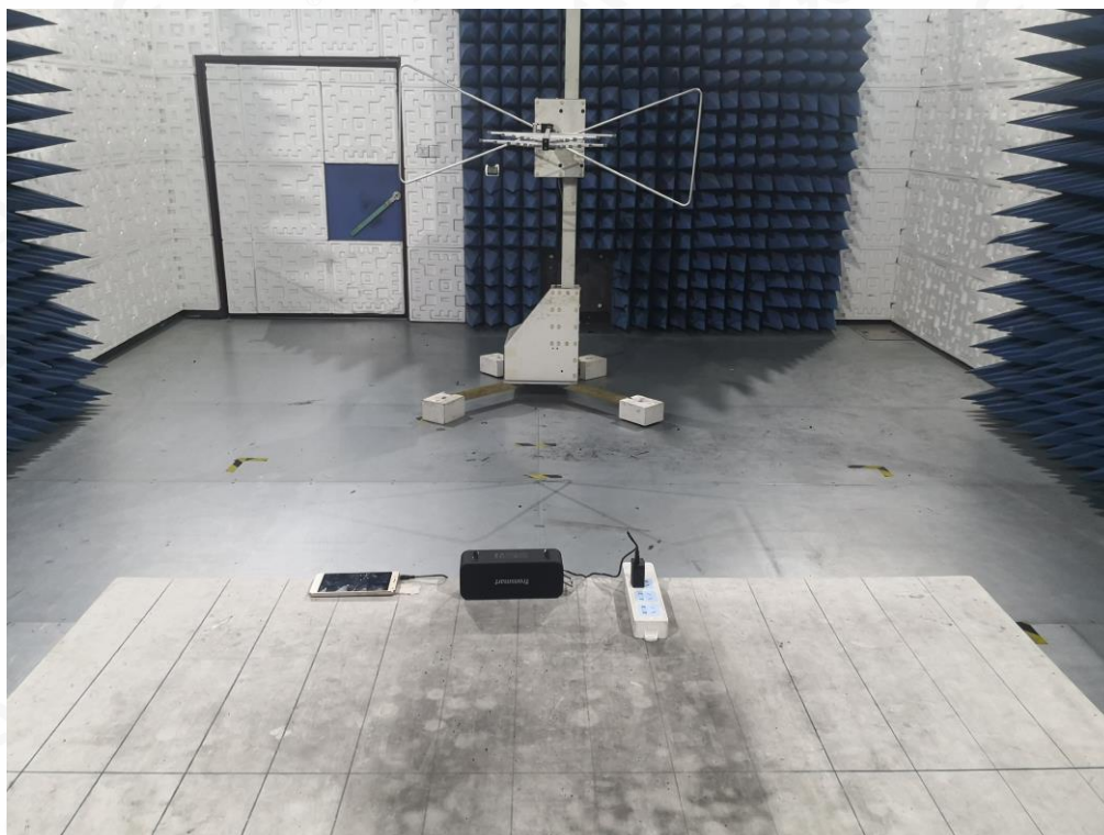
RADIATED EMISSION TEST SETUP ABOVE 1GHZ
