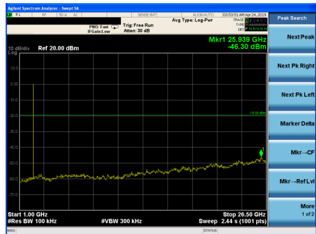
GFSK on channel 39
