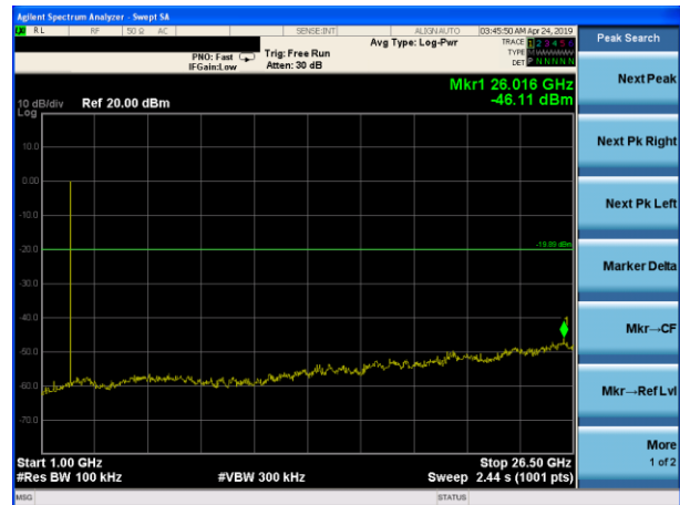
GFSK on channel 00
