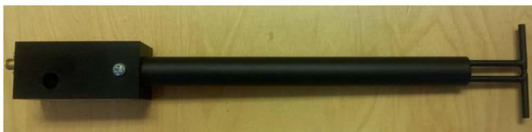
Figure 1 – MVG COMOSAR Validation Dipole
