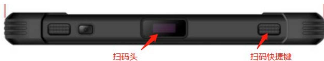
Center the green beam on the barcode. Please adjust the distance between the lens and the barcode as appropriate; barcode The smaller the barcode is, the closer it is; the larger the barcode is, the farther away it is.
