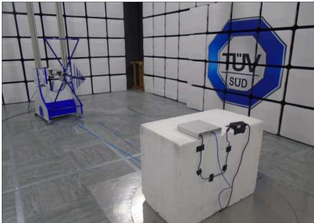
Figure 12 - Test Setup - Below 1 GHz
