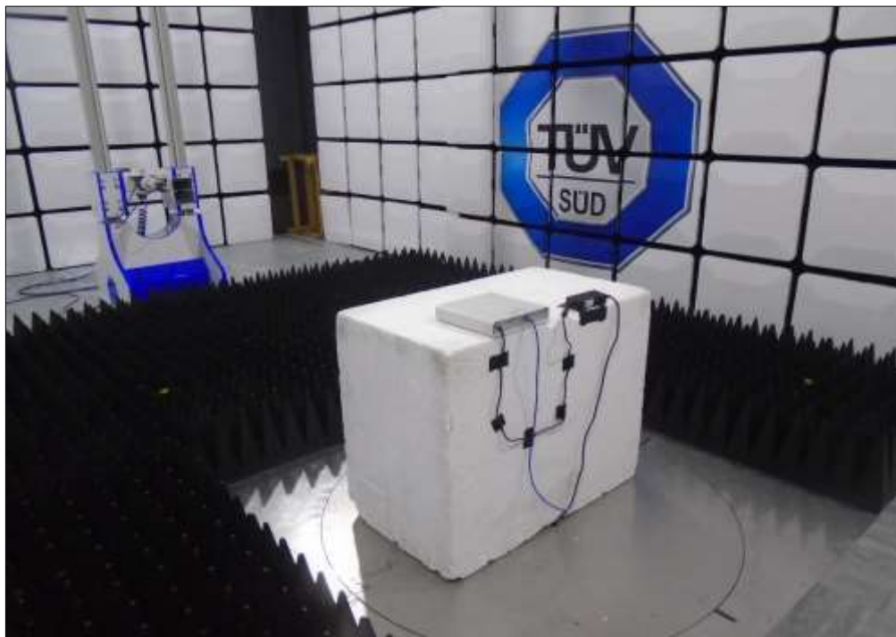
Figure 13 - Test Setup - Above 1 GHz
