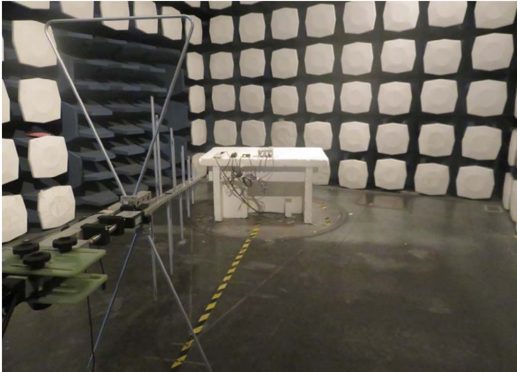
FCC Part15C Radiated Emission Test Setup
