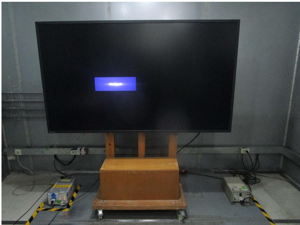
**Radiated Emissions Test Photos****9 kHz to 30 MHz**
