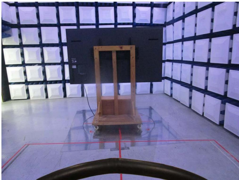
**Radiated Emissions Test Photos****30 MHz to 1000 MHz**
