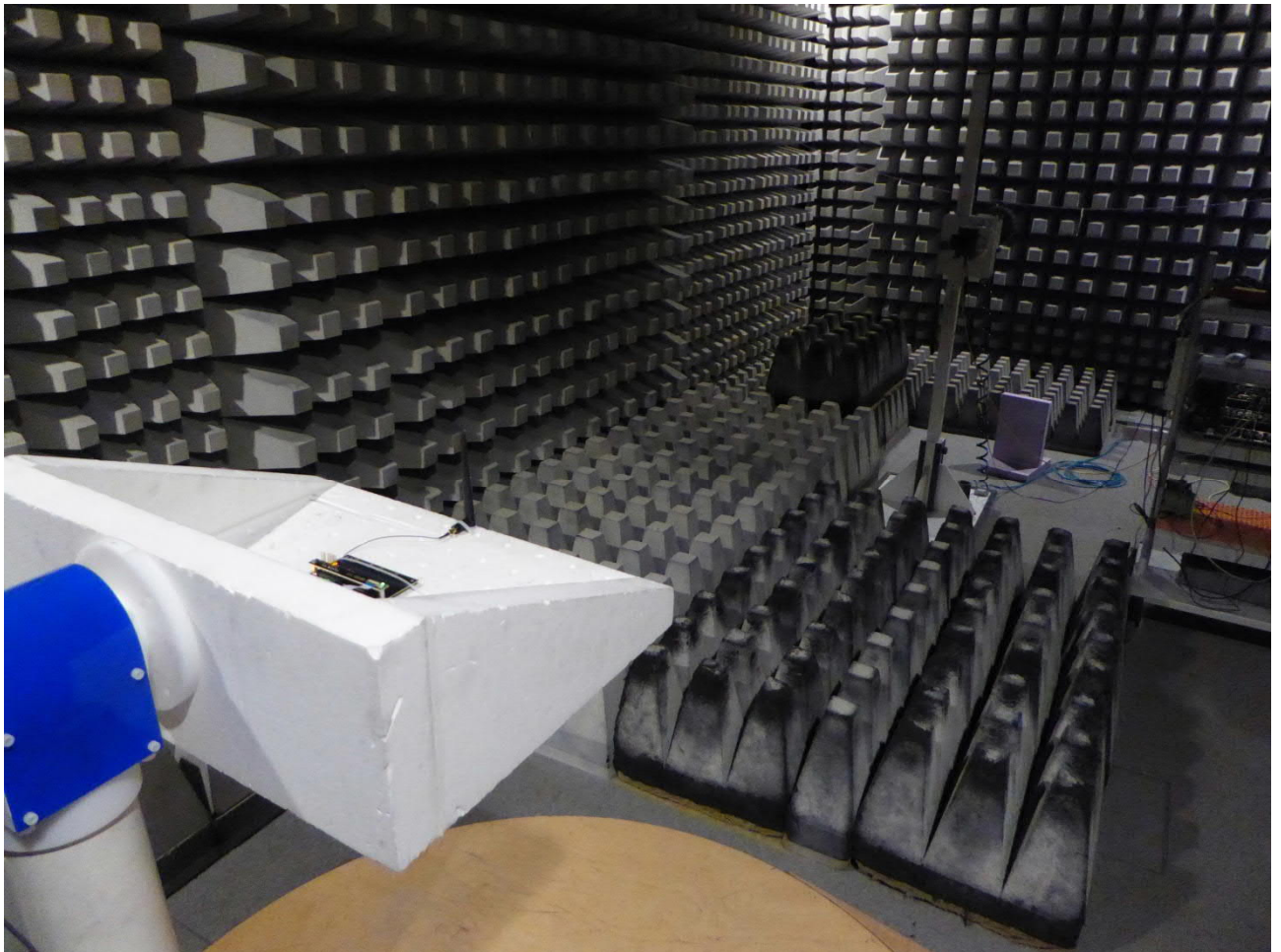
Test setup fully anechoic chamber 12 – 18 GHz
