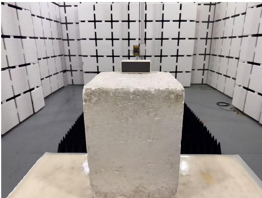
Set-up for Radiated Spurious Emission, Above 1GHz
