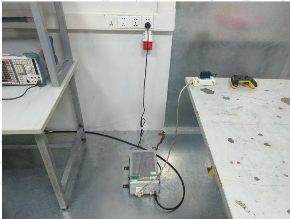
Photo of Conducted Emission Measurement
