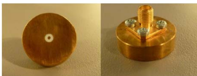
Figure 1 – MVG LIMESAR Dielectric Probe
