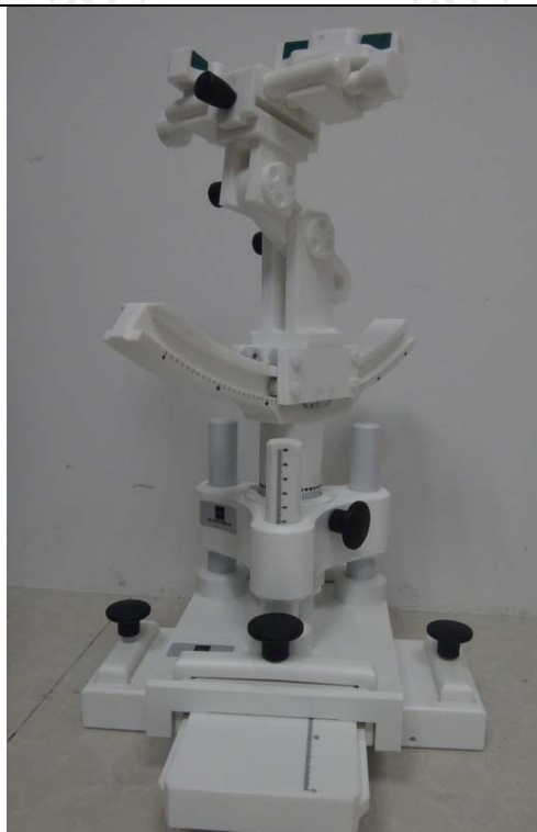
COMOSAR Mobile phone positioning system
