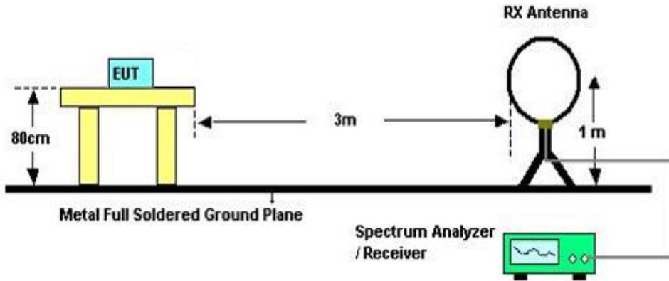
The setting of the spectrum analyzer
