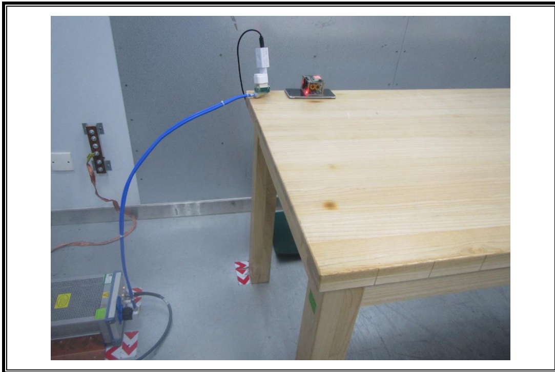
POWERLINE CONDUCTED EMISSIONS MEASUREMENT SETUP
