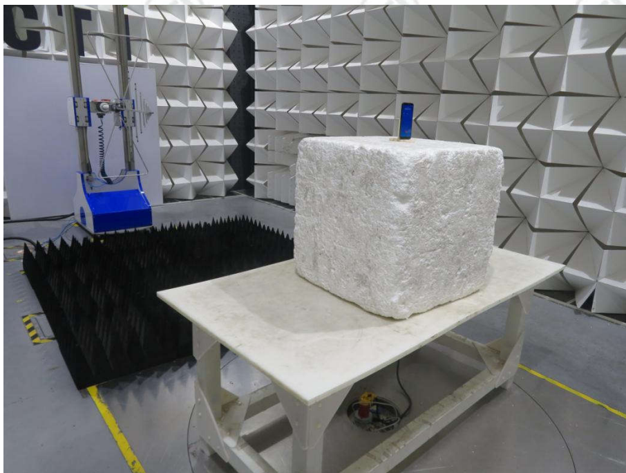
Radiated spurious emission Test Setup-1(Below 1GHz)
