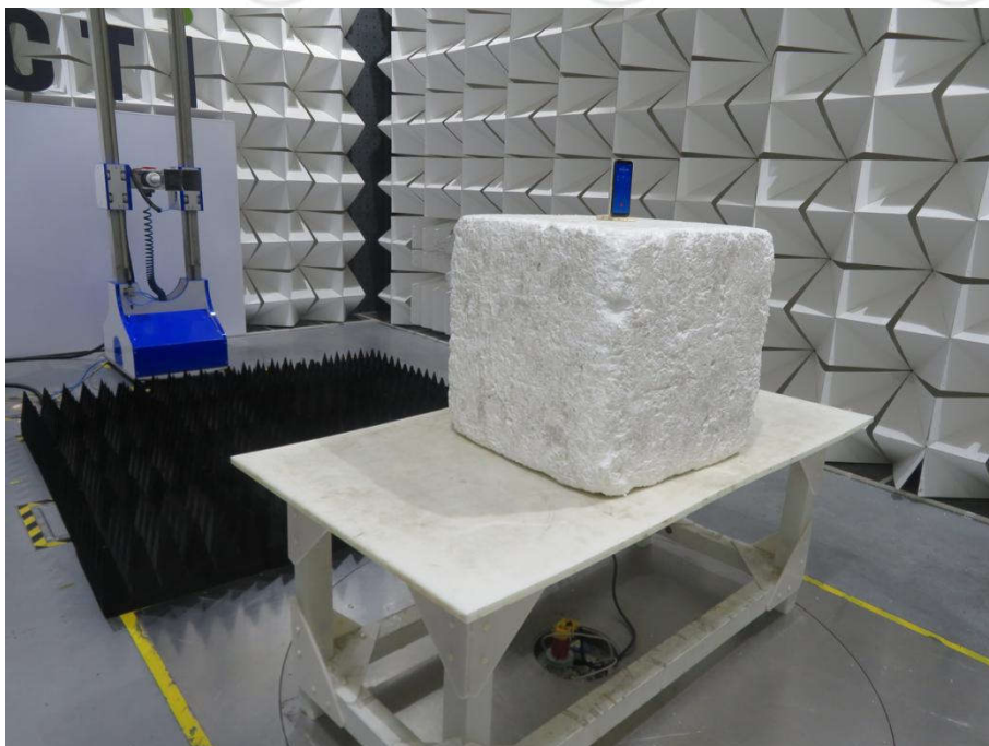
Radiated spurious emission Test Setup-2(Above 1GHz)
