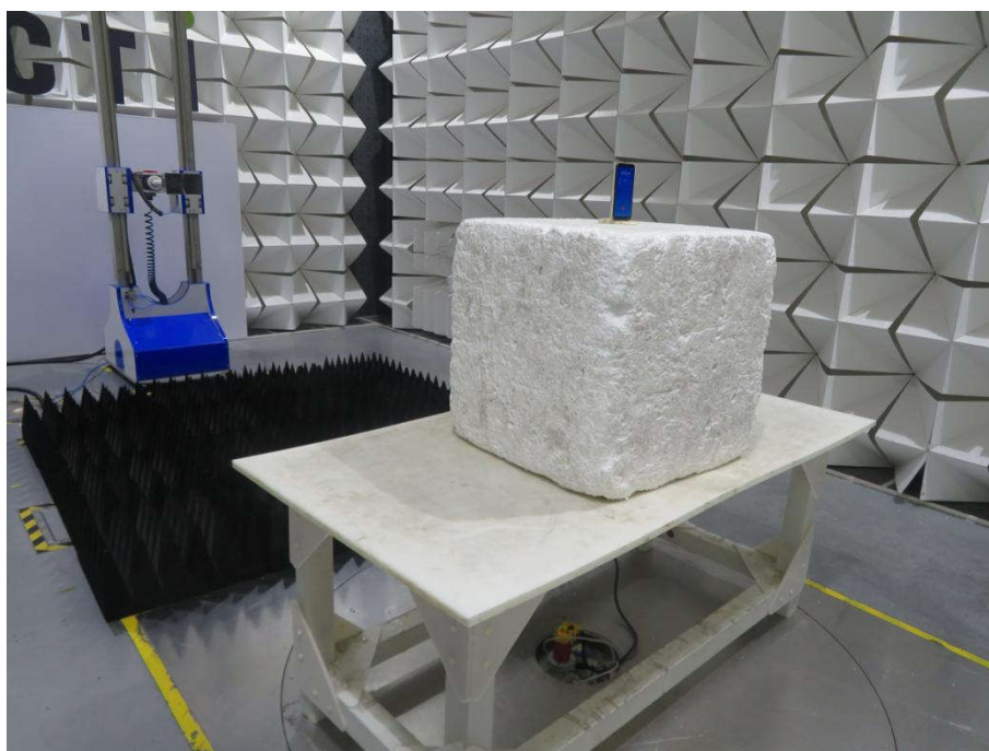
Radiated spurious emission Test Setup-2(Above 1GHz)
