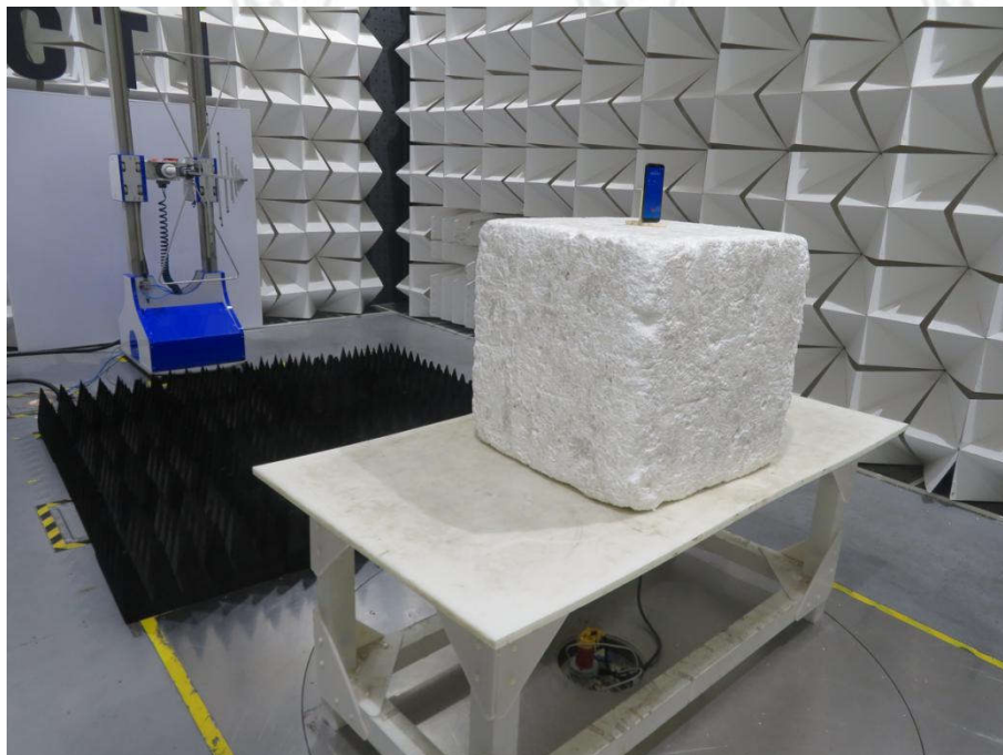
Radiated spurious emission Test Setup-1(Below 1GHz)
