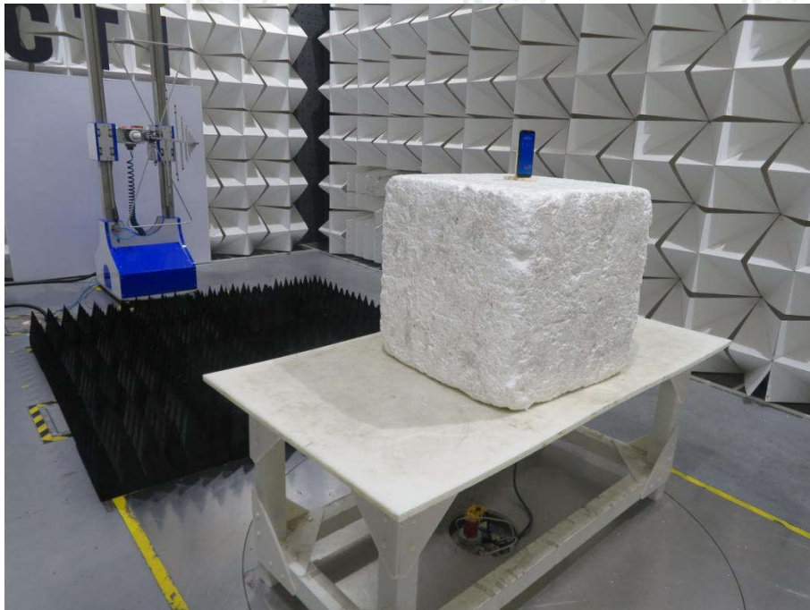
Radiated spurious emission Test Setup-1(Below 1GHz)
