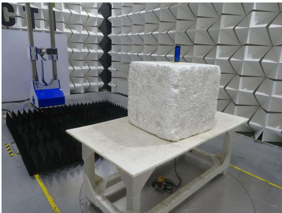
Radiated spurious emission Test Setup-2(Above 1GHz)
