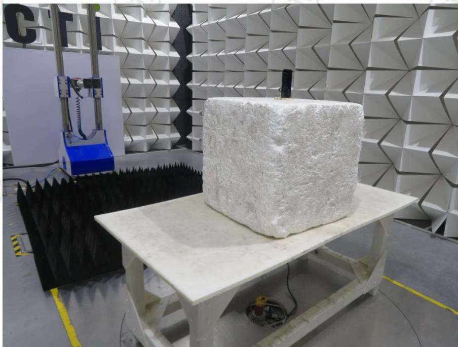
Radiated spurious emission Test Setup-3(Above 1GHz)
