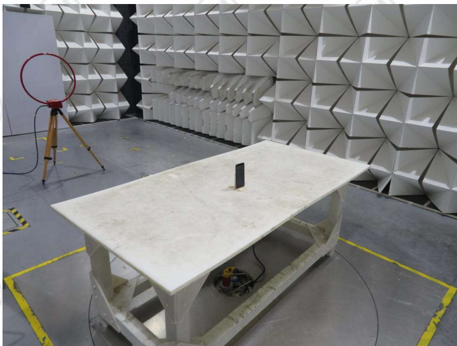
Radiated spurious emission Test Setup-2(Below 30M)
