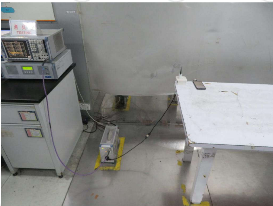
Conducted Emissions Test Setup
