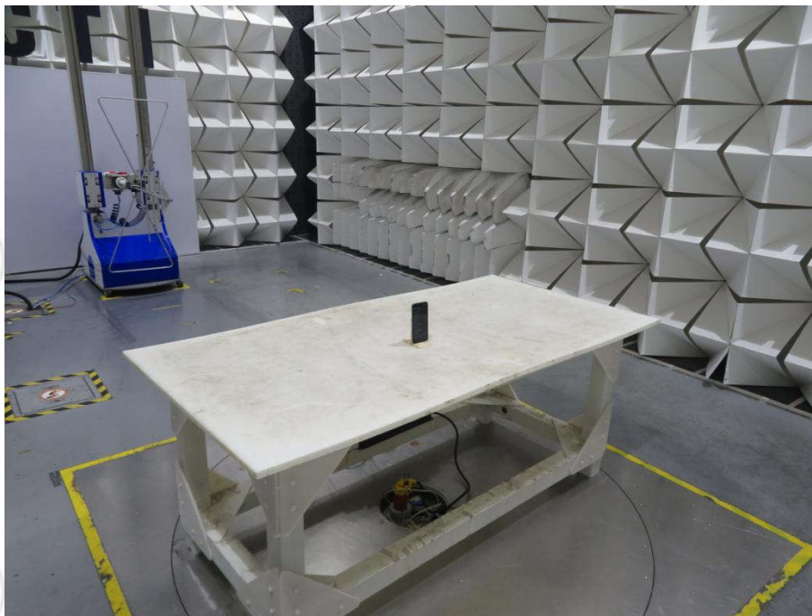
Radiated spurious emission Test Setup-1(Below 1GHz)
