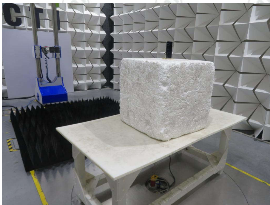
Radiated spurious emission Test Setup-3(Above 1GHz)
