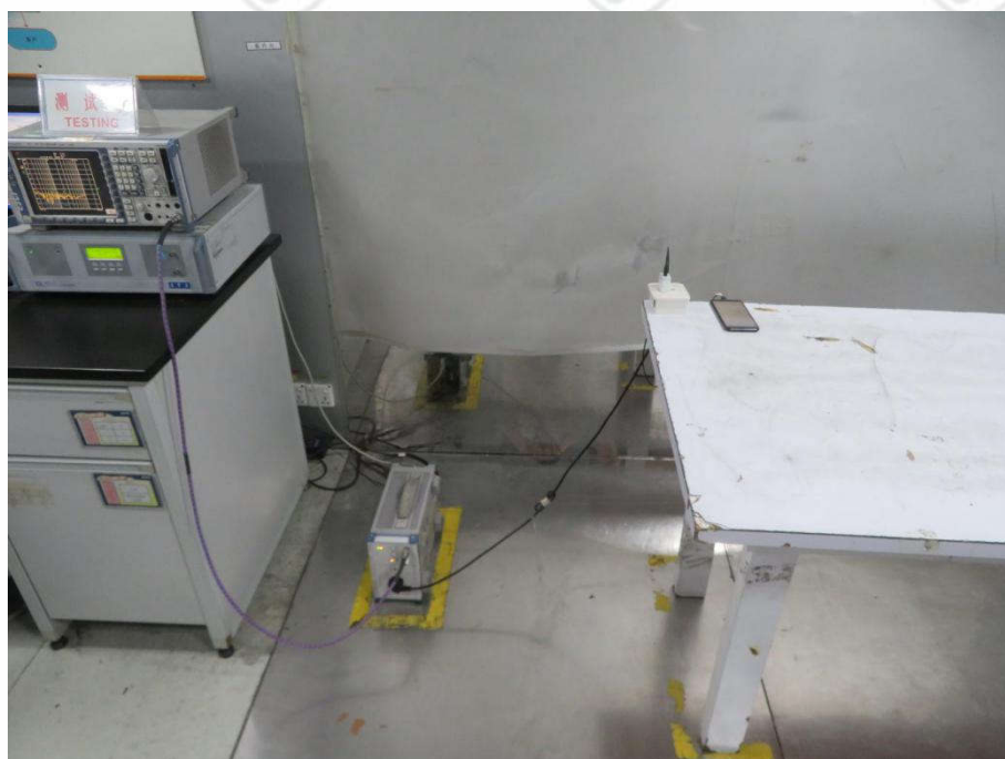
Conducted Emissions Test Setup
