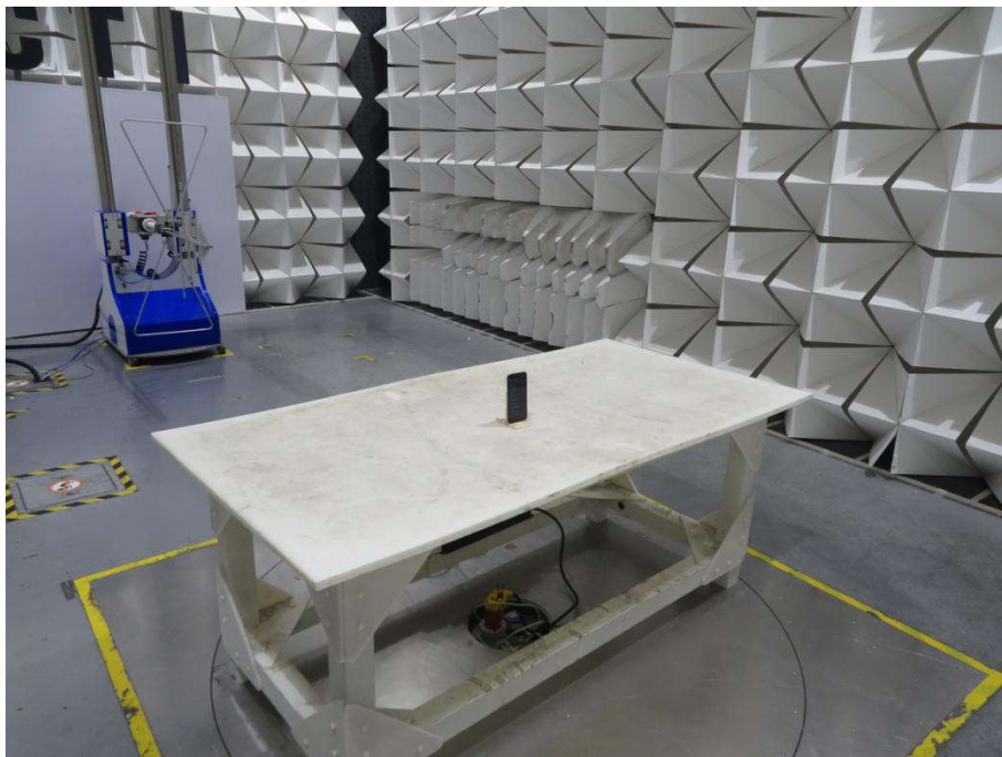
Radiated spurious emission Test Setup-1(Below 1GHz)
