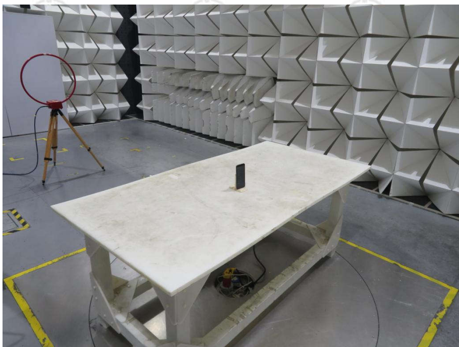
Radiated spurious emission Test Setup-2(Below 30M)
