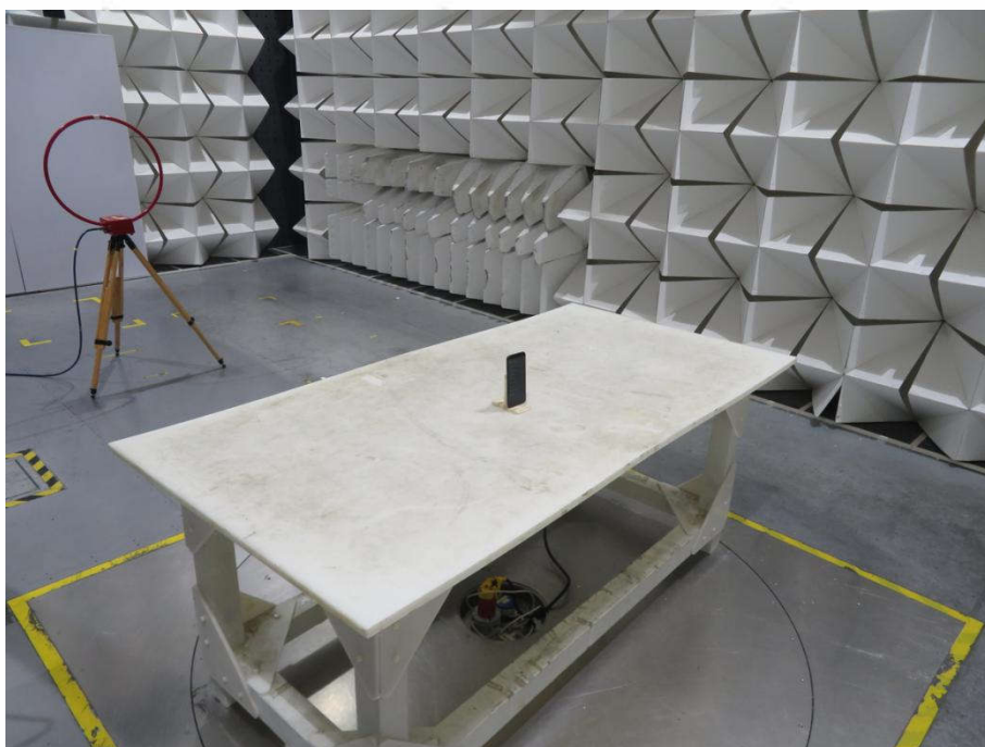
Radiated spurious emission Test Setup-2(Below 30M)
