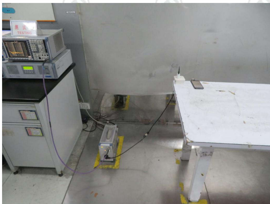
Conducted Emissions Test Setup
