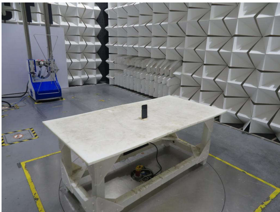
Radiated spurious emission Test Setup-1(Below 1GHz)
