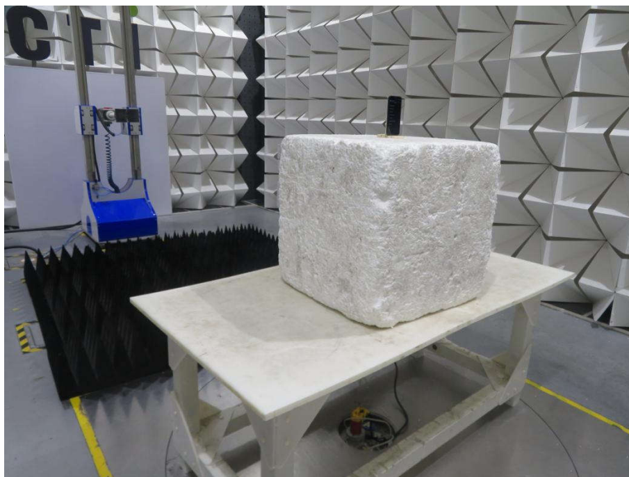
Radiated spurious emission Test Setup-3(Above 1GHz)
