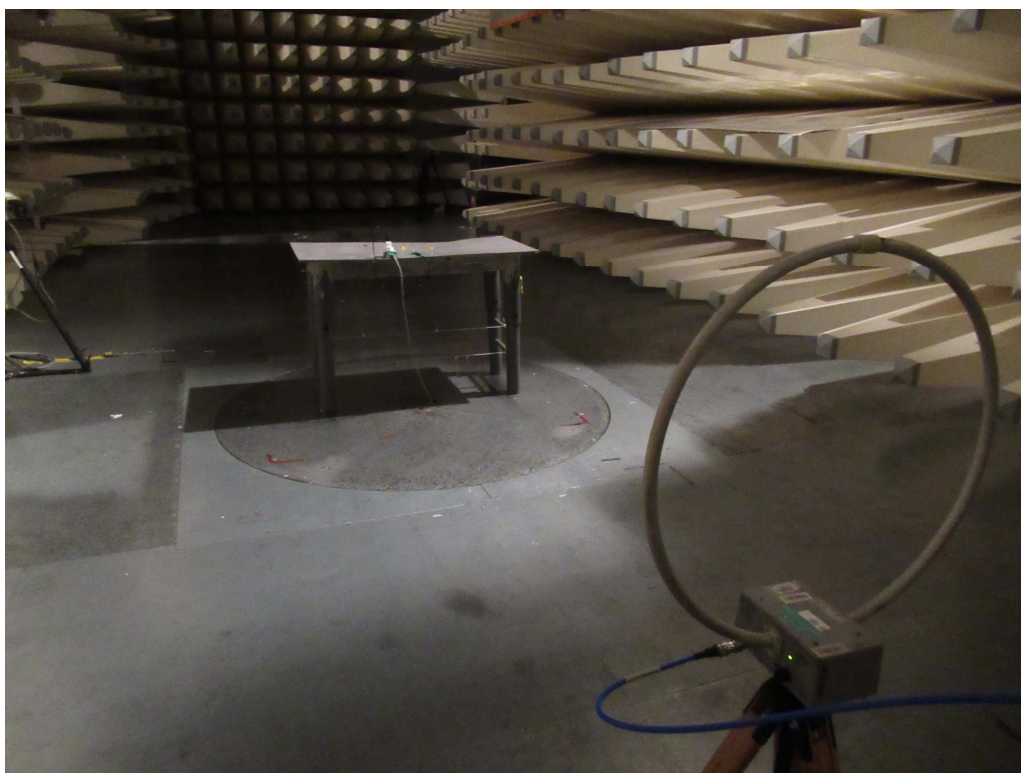
Set-up for Radiated Emission
