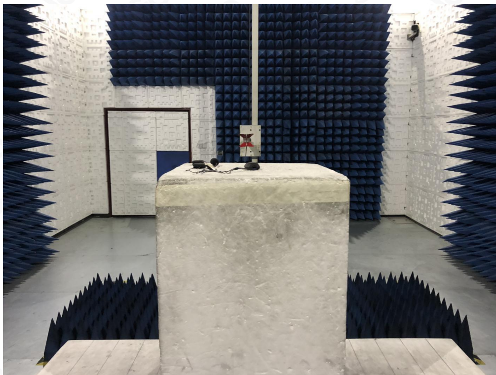
RADIATED EMISSION TEST SETUP ABOVE 1GHZ
