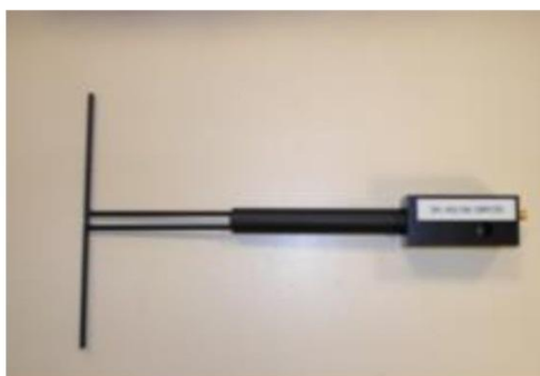
Figure 1 – Satimo COMOSAR Validation Dipole
