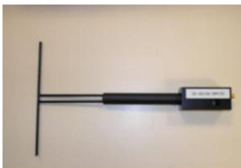
Figure 1 – Satimo COMOSAR Validation Dipole
