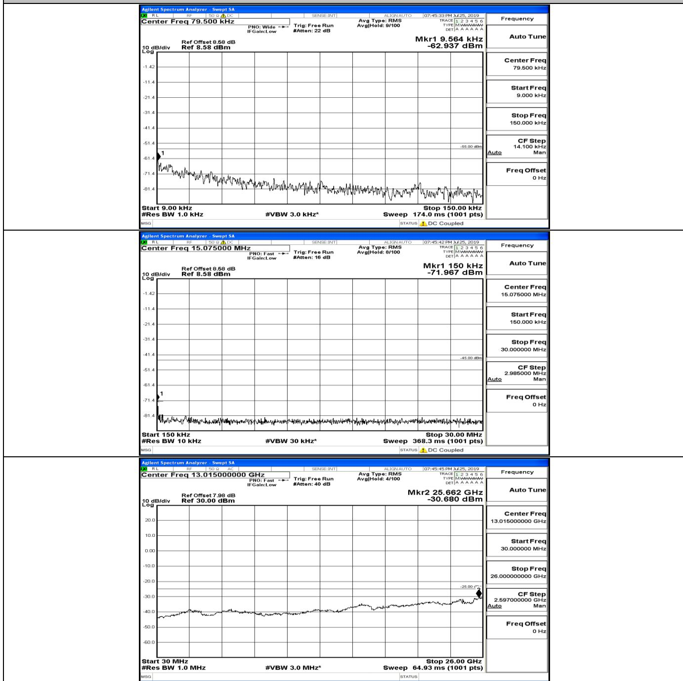
CSE Test Graph(s) (Channel Bandwidth: 10 MHz)\_MCH\_16QAM
