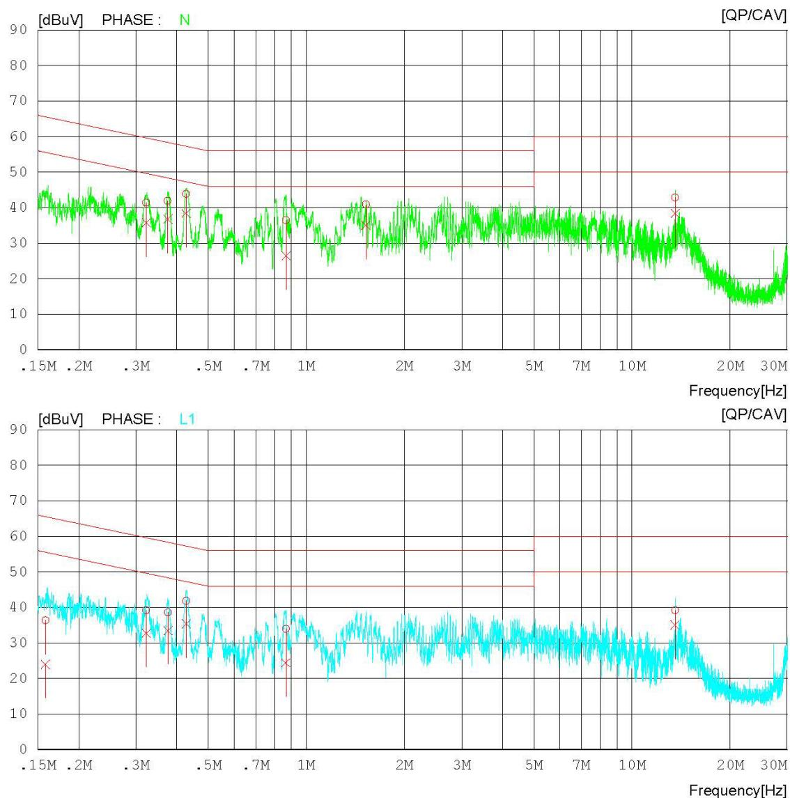
**Measurement Data****Results of Conducted Emission**
