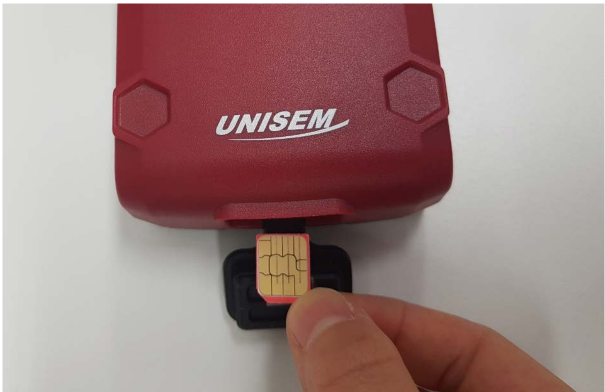
< Figure. Actual device USIM insertion example>
