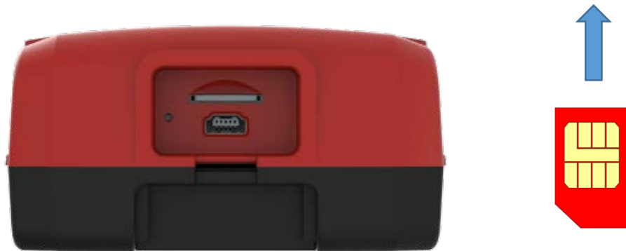
<Figure. Device USIM insertion direction>
