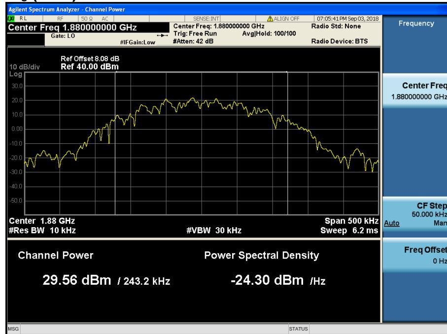
$$\text{PAPR (dB)} = \text{P}_{\text{Pk}} (\text{dBm}) - \text{P}_{\text{Avg}} (\text{dBm}) = 29.75 \text{ dBm} - 29.56 \text{ dBm} = 0.19 \text{ dB}$$
