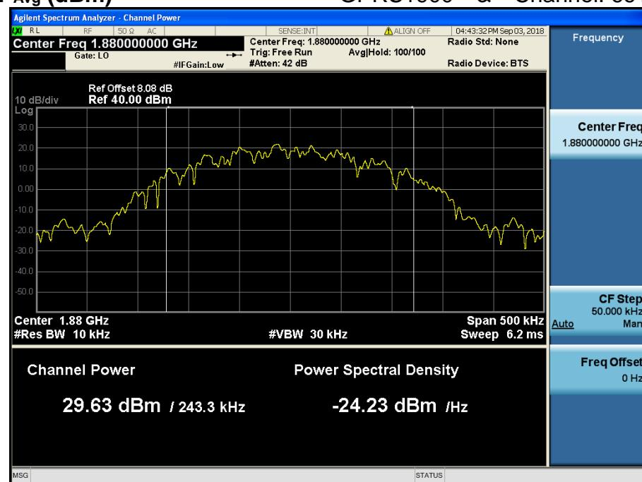
$$\text{PAPR (dB)} = \text{P}_{\text{Pk}} (\text{dBm}) - \text{P}_{\text{Avg}} (\text{dBm}) = 29.71 \text{ dBm} - 29.63 \text{ dBm} = 0.08 \text{ dB}$$
