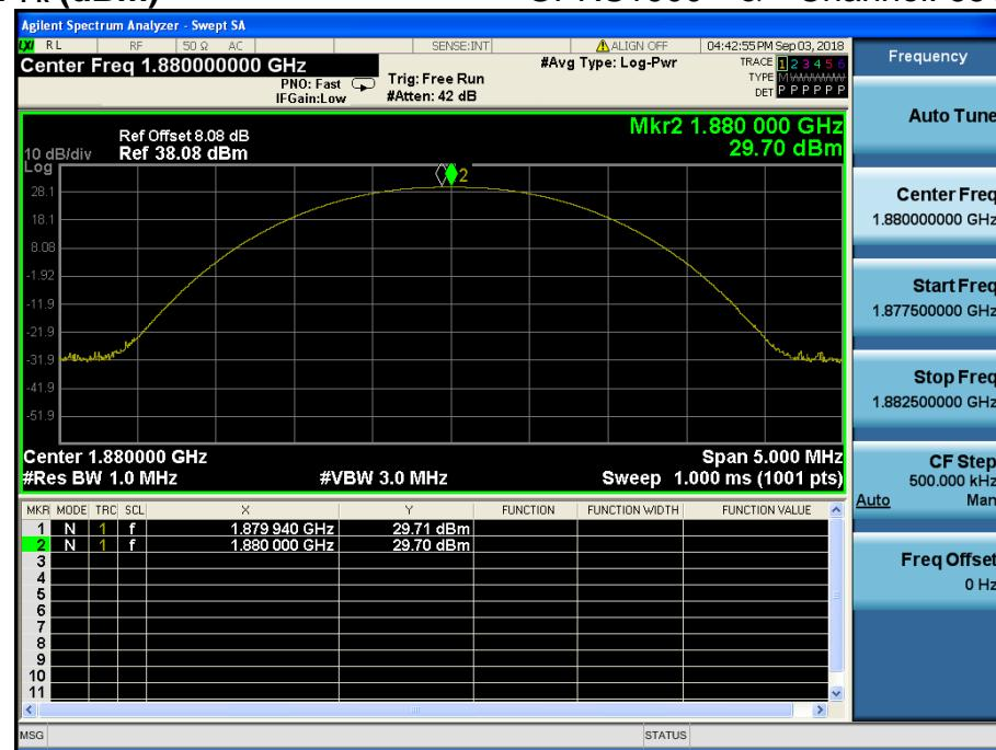
**-P<sub>Avg</sub> (dBm)**      GPRS1900 & Channel: 661
