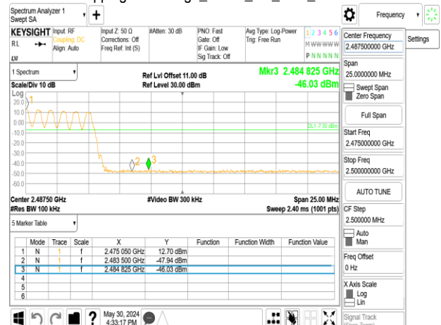
Hopping Band Edge_GFSK_1M_DH5_2480MHz
