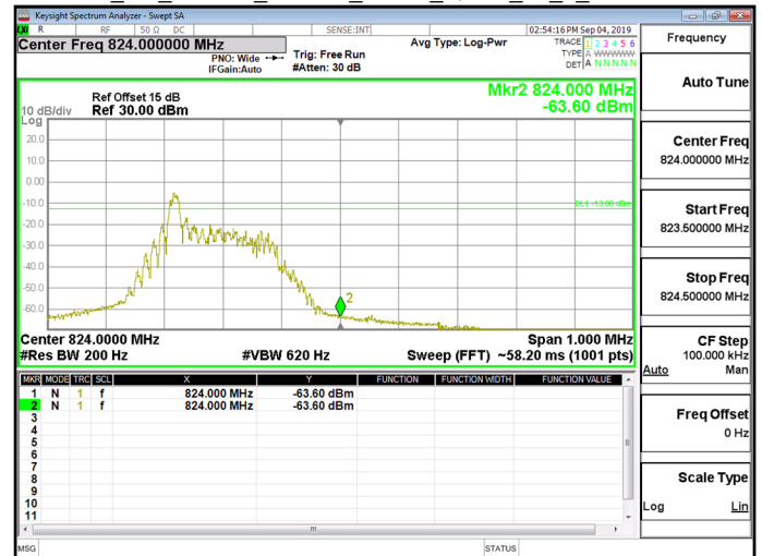
NB_IoT_Band26_Part90s_15kHz_QPSK_12_0_CH26788
