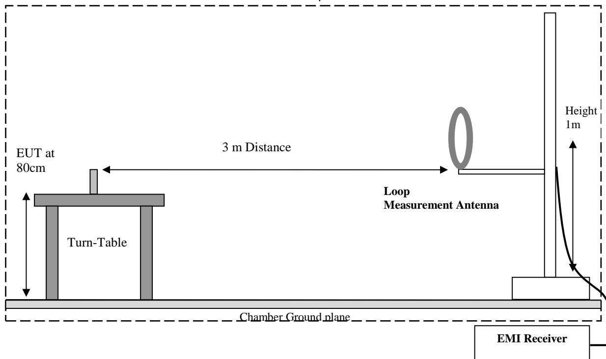
Radiated Emissions Test Setup 30MHz-1GHz Measurements
