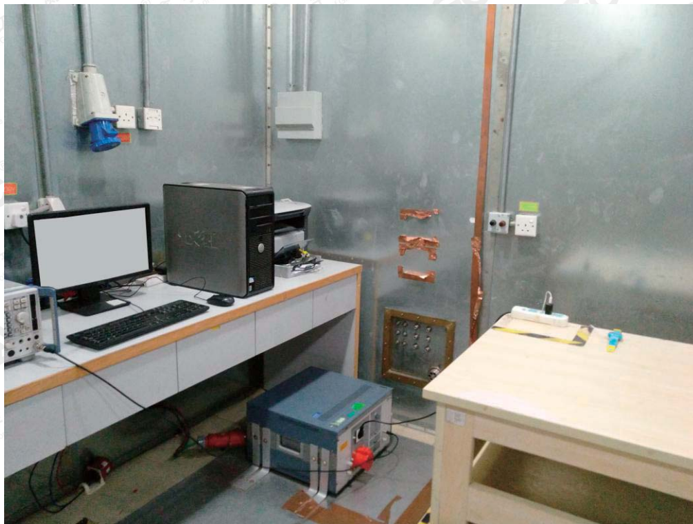
RADIATED EMISSION TEST SETUP
