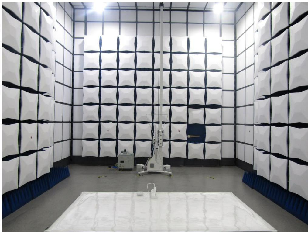
RADIATED EMISSION ABOVE 1G TEST SETUP
