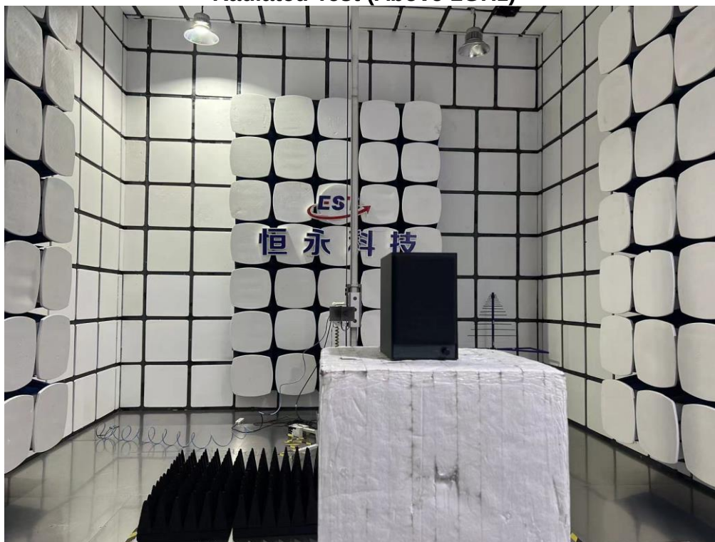
Radiated Test (Above 1GHz)
