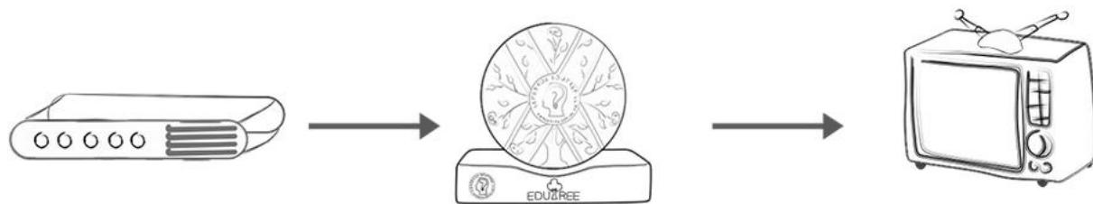
EduTree has AV and HDMI interface for connecting with set top box and TV. Some of the old TV and set top box have only AV (Yellow, Red and White) cable connections. So AV ports can be used in that case. See below image for more information.
