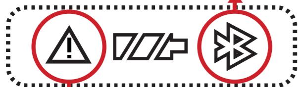
**In the event of an emergency overheat,** the emergency shut off icon will display in the LCD screen. Turn off the battery or remove bottle from AC/DC adapter & reinstall to reset the protection circuit.
