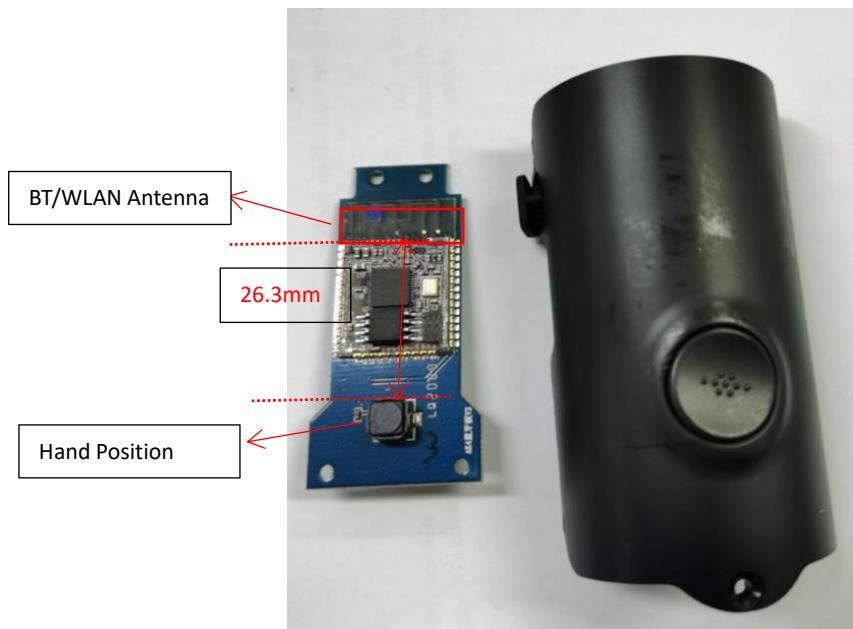
Note: According to hand-held condition the nearest distance between BT/WLAN Antenna to human hand is **26.3** mm.
