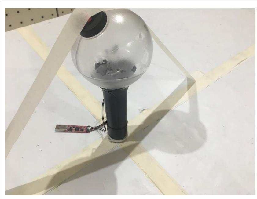
**2. Photo of Radiated Spurious Emission Test (Below 1 GHz)**
